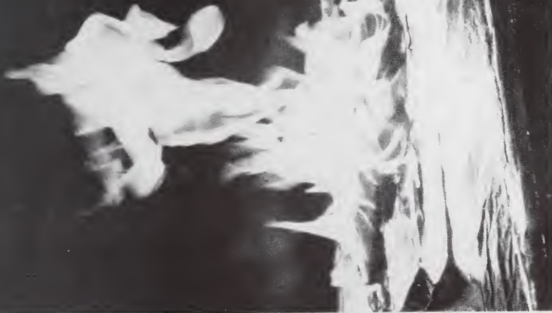
Figure 11. Bare Polyurethane #2 Mattress Specimen 7 Minutes After Ignition in the Horizontal Position in the Hood.
