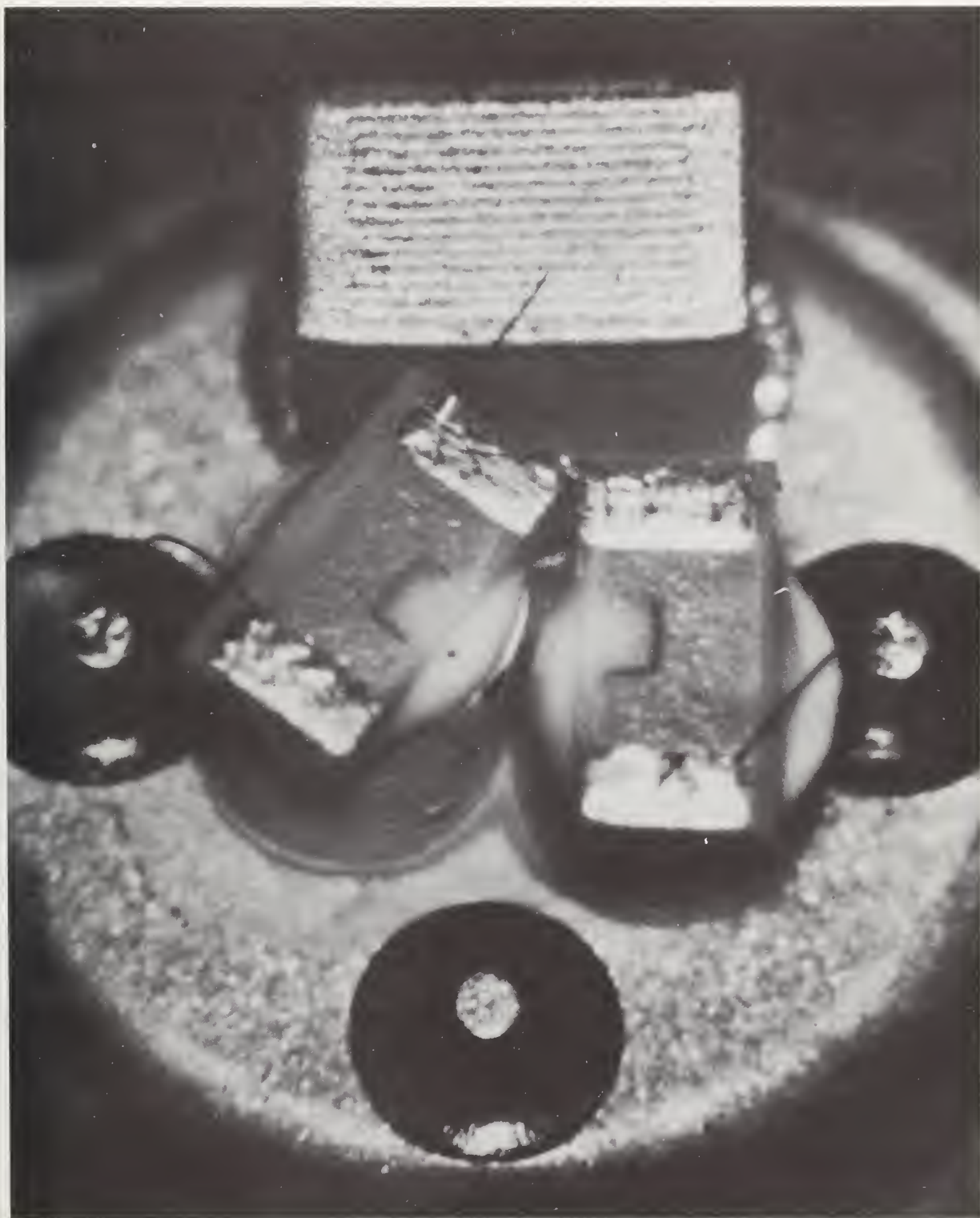
Figure 9. Photograph of an R-C Delay Time Network Having The Circuit Shown In Figure 1a.
