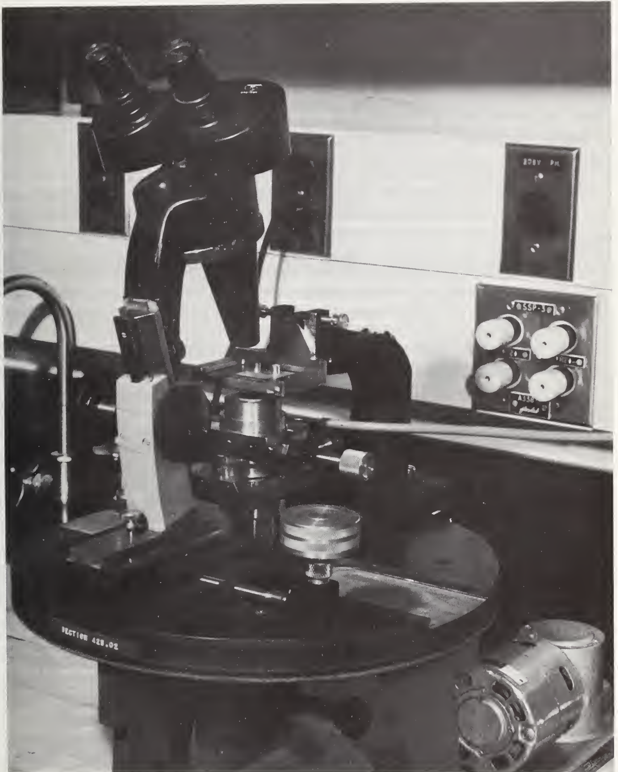
Figure 23. The Work Station Used to Move a Probe Assembly and a PRU Wafer Relative to Each Other.
