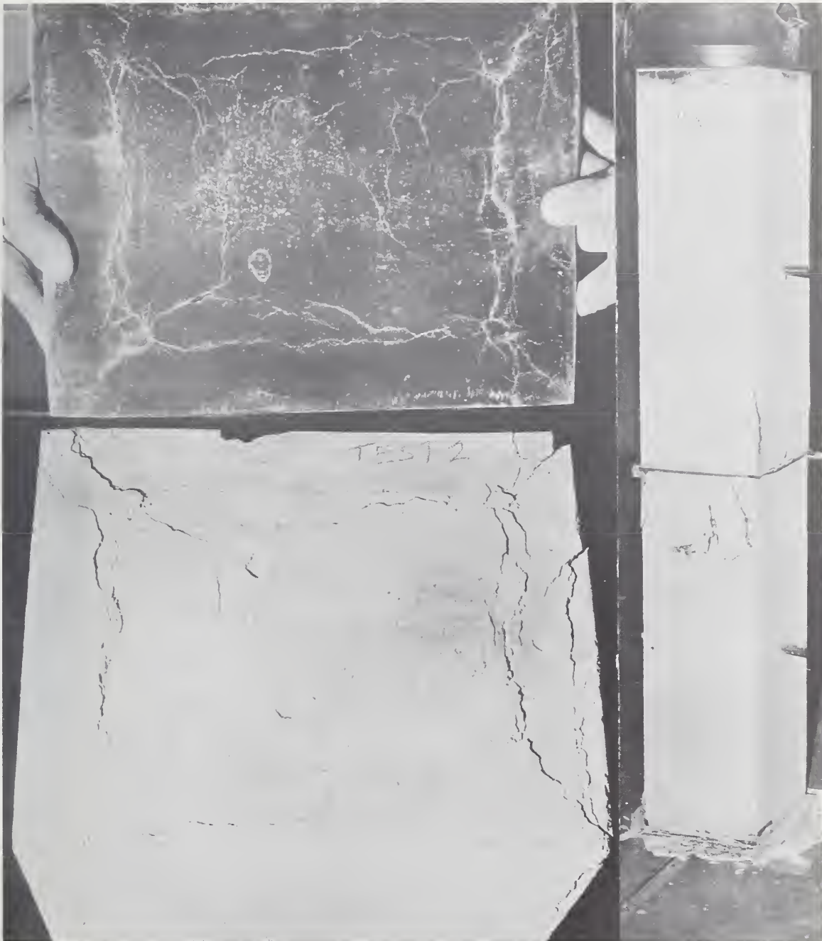
FIGURE 4.5 TYPICAL FAILURE OF CONNECTION USING 1/4-IN NEOPRENE PAD
