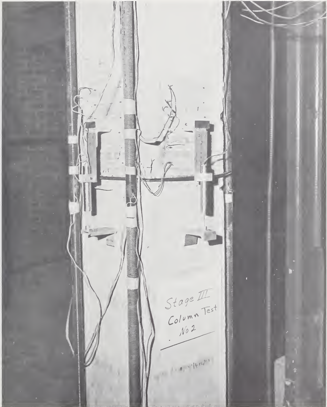
FIGURE 4.15 INSTRUMENTATION OF TEST SPECIMEN WITH GROUTED DOWEL
