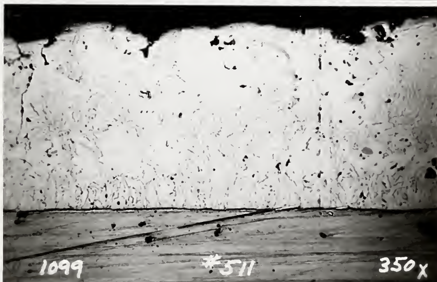
Figure 17. Heat-treated series. Top 250°C for 2 hrs, center 400°C for 1 hr, bottom 600°C for 1 hr. Chromium deposited on copper from bath containing 3 g/l Tl NO_3 . No etch.
