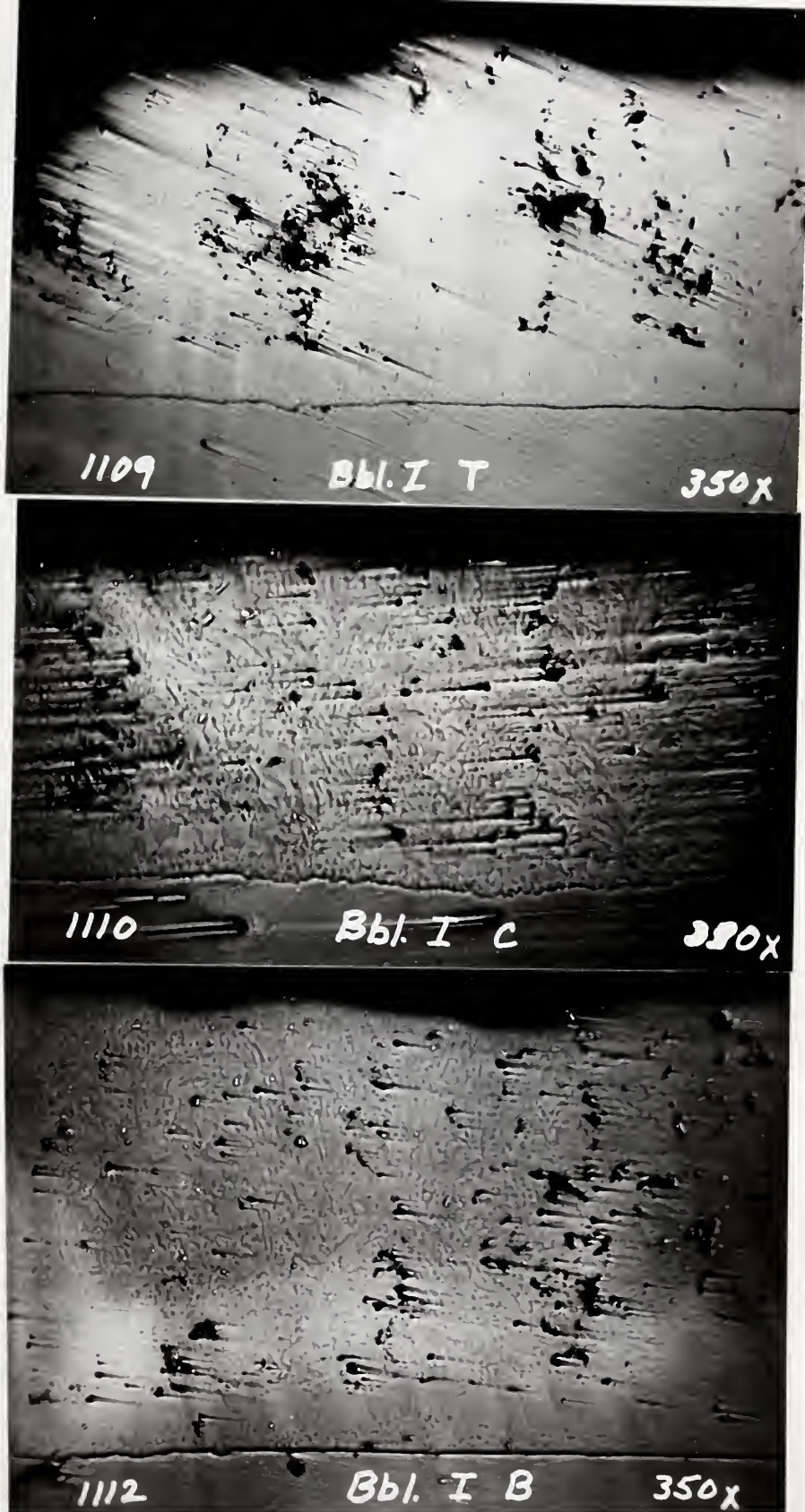
Figure 16. Chromium deposit on inside of stainless steel tube 3/8 inch ID x 20 inches long. Chromium deposited at 45°C/30 asd in tube in vertical position from bath containing 3 g/l Tl NO 3 and 30 g/l B 4 C. Cross-sections taken from top, center, and bottom of tube. Hard particles resist polishing and leave "tails" of raised Cr. No etch.
