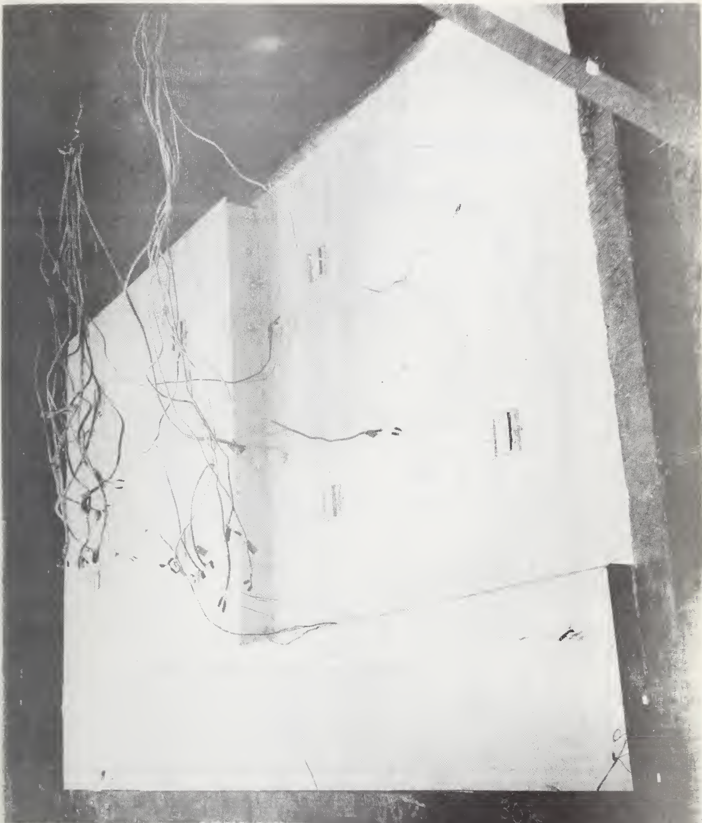
Fig. 2 Unexposed surface of the complete wall assembly mounted in the furnace and connection of the thermocouples.
