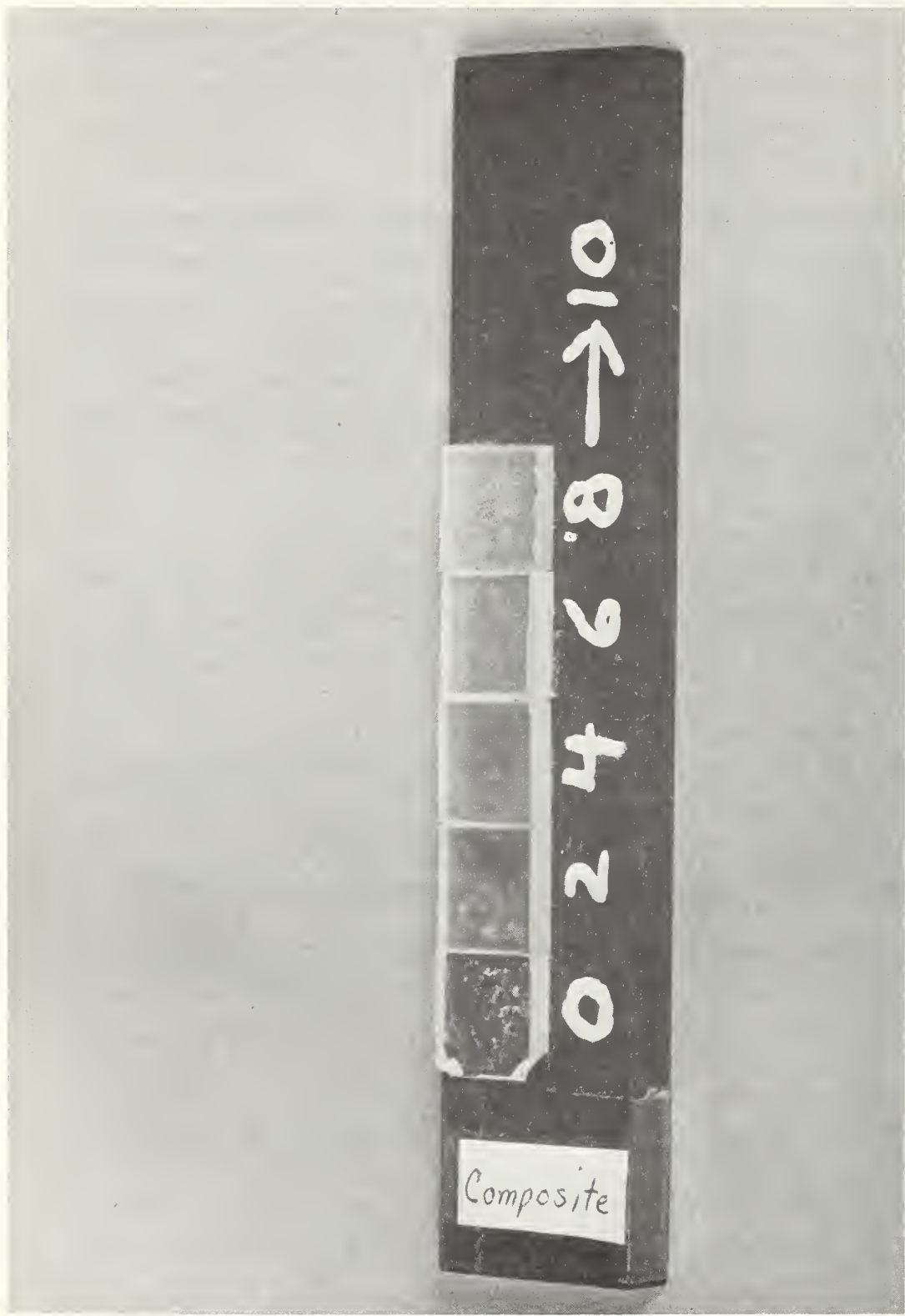
Fig. 1 - Surface texture evaluation guide composed of glass blocks of increasing roughness (see text). The evaluator (using a dental explorer) matches the roughness of the restoration with that of one of the blocks.
