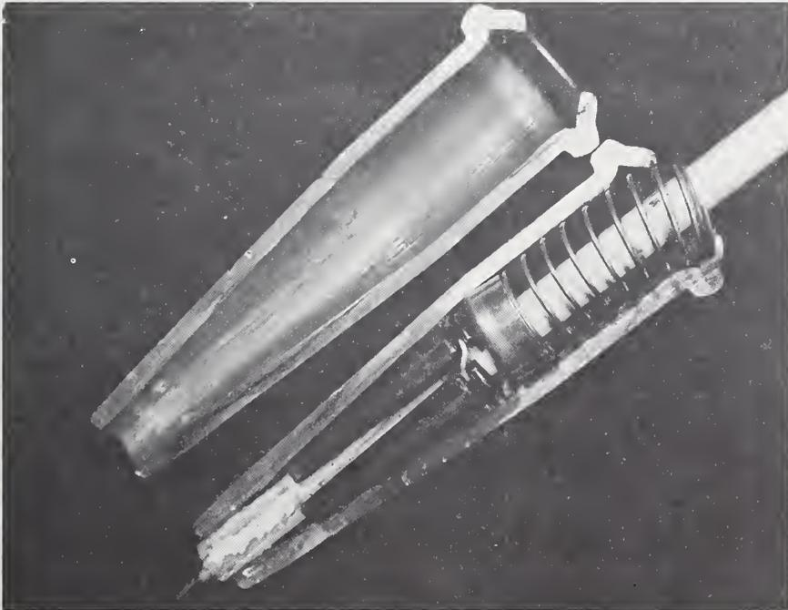
Figure 4 - Type R/V end fitting.
