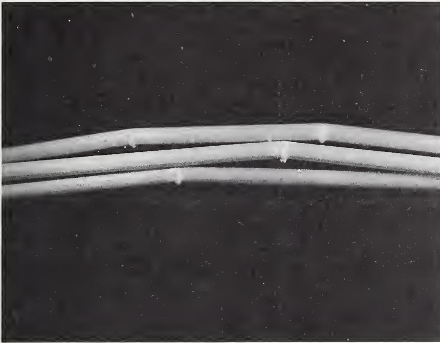
Figure 21 - Typical buckles in 1/2-in Material E, resulting from coiled storage at elevated temperature.
