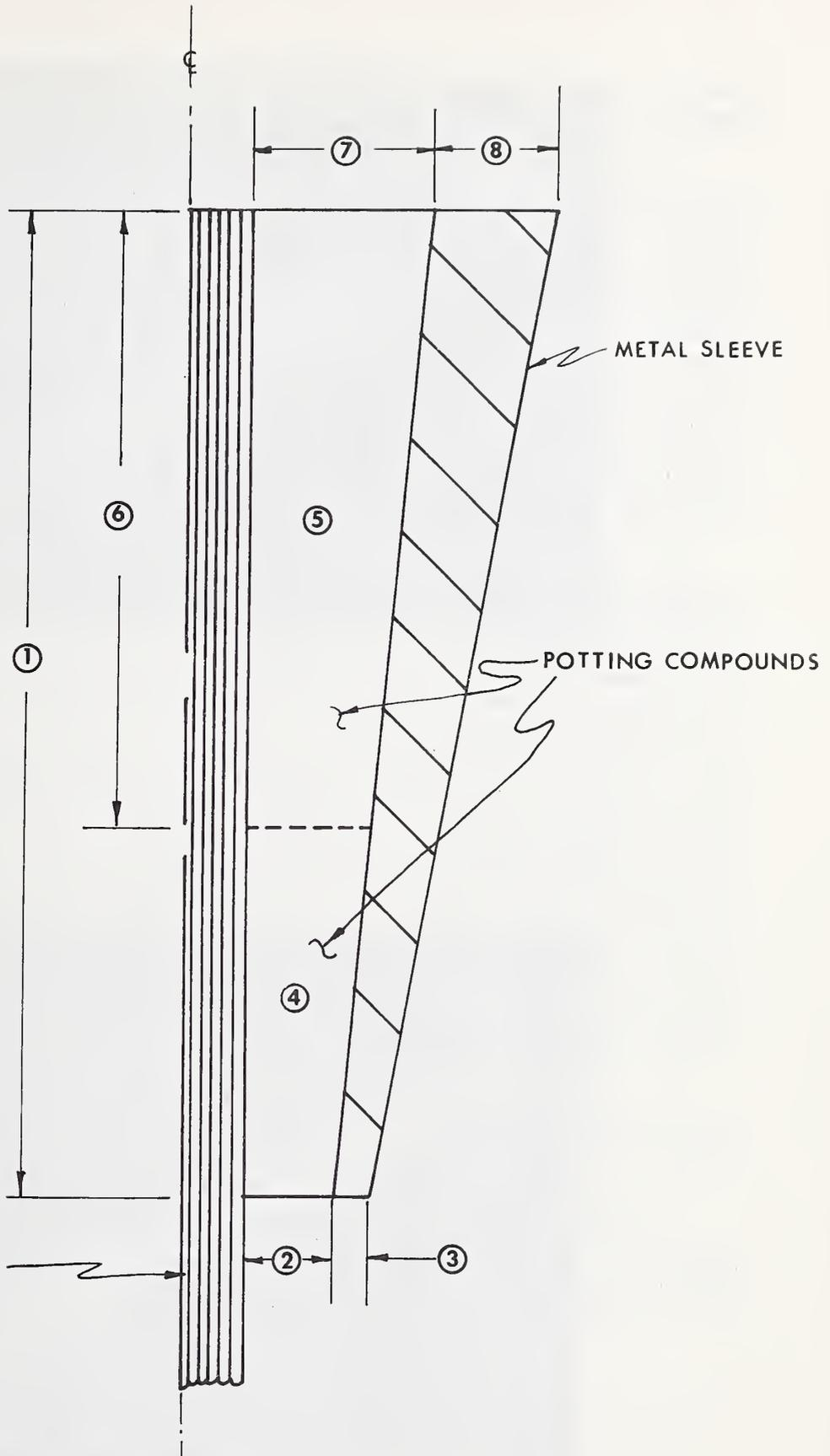
Figure 10 - Parameters for one general class of end fittings.
