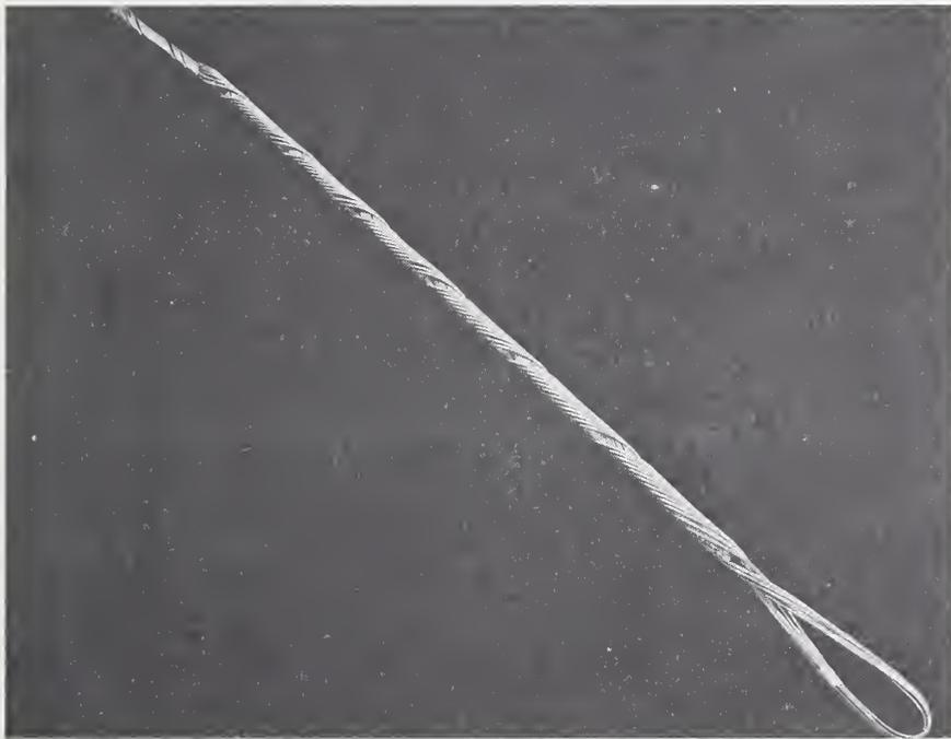
Figure 3 - Type F/A end fitting.
