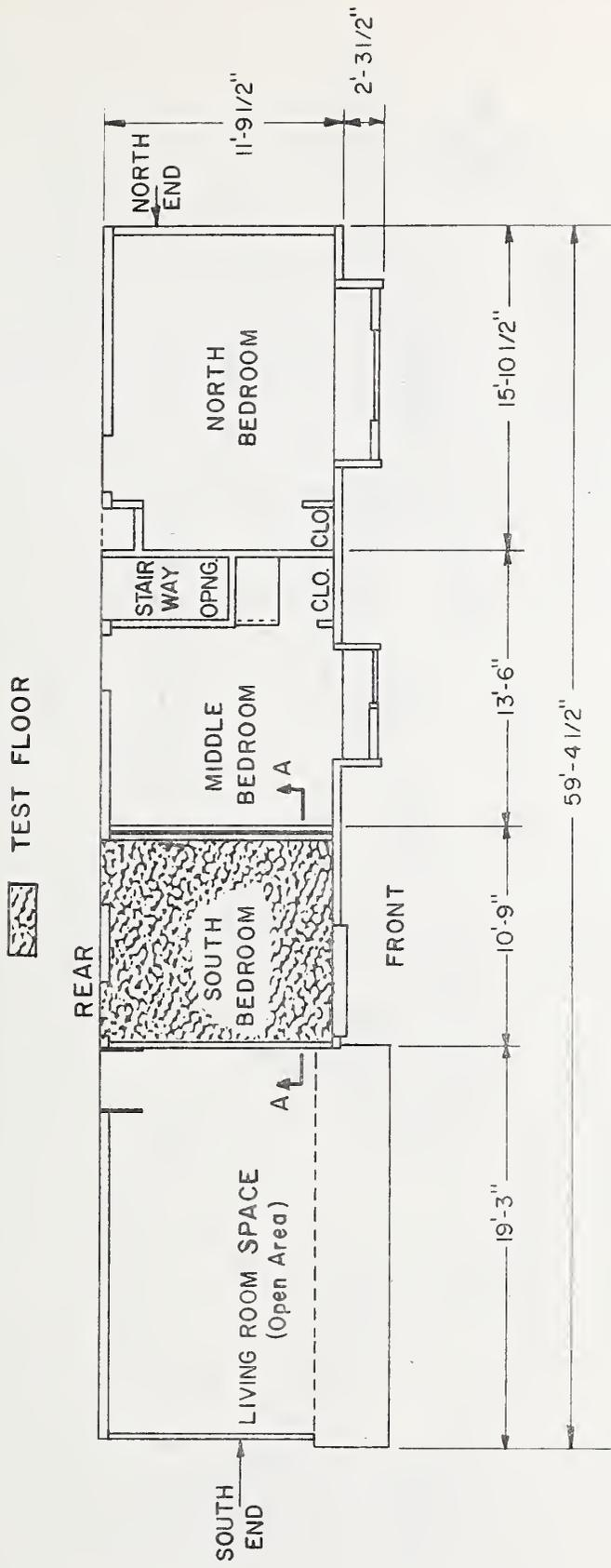
Figure 3.2 Test Floor For Sustained Load- Test 3
