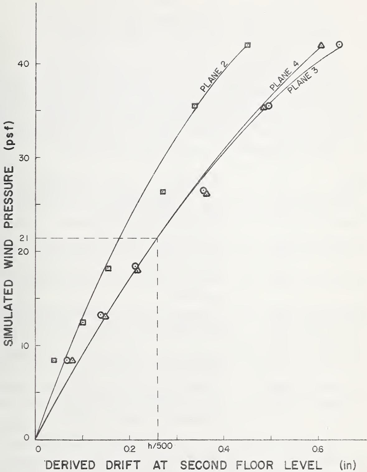
Figure 7.2 Wind Pressure versus Derived Drift Curves - Test 1
