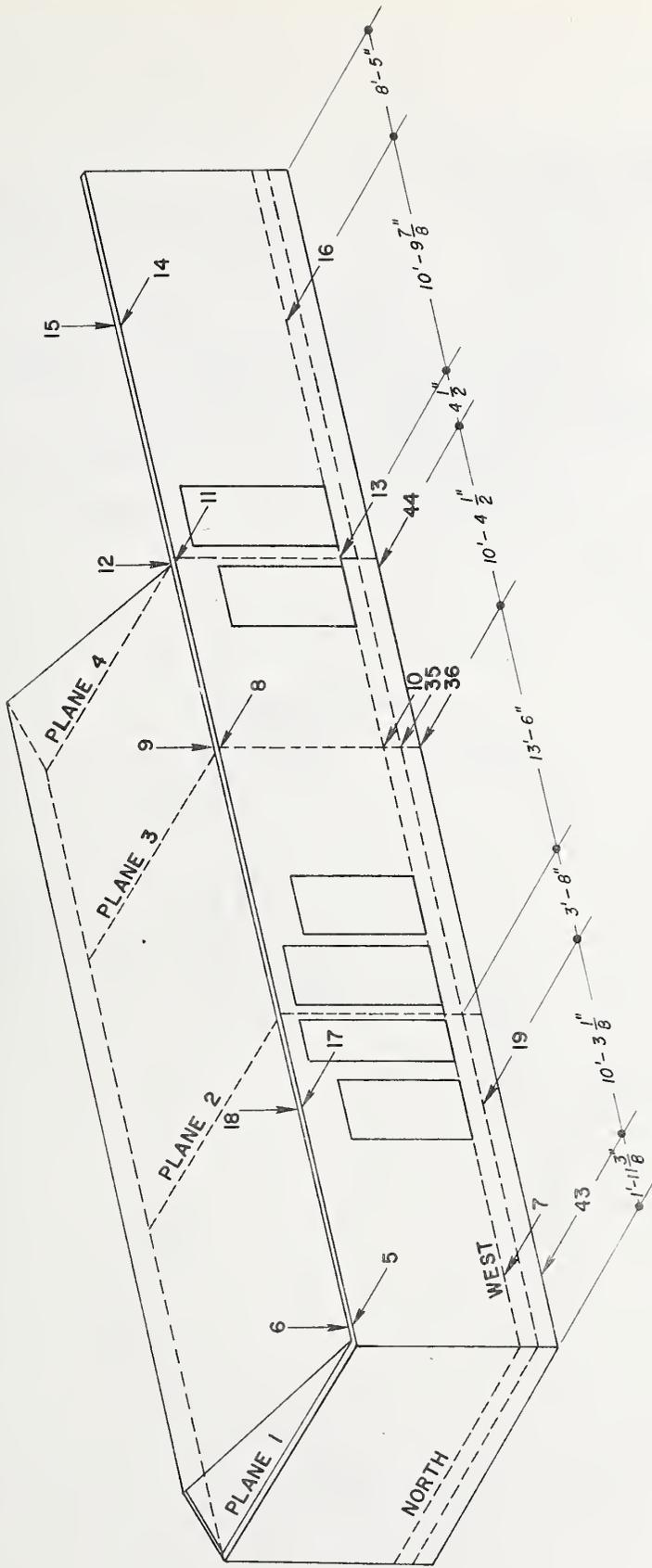
Figure 4.2 Exterior Instrumentation on the Rear - Test I
