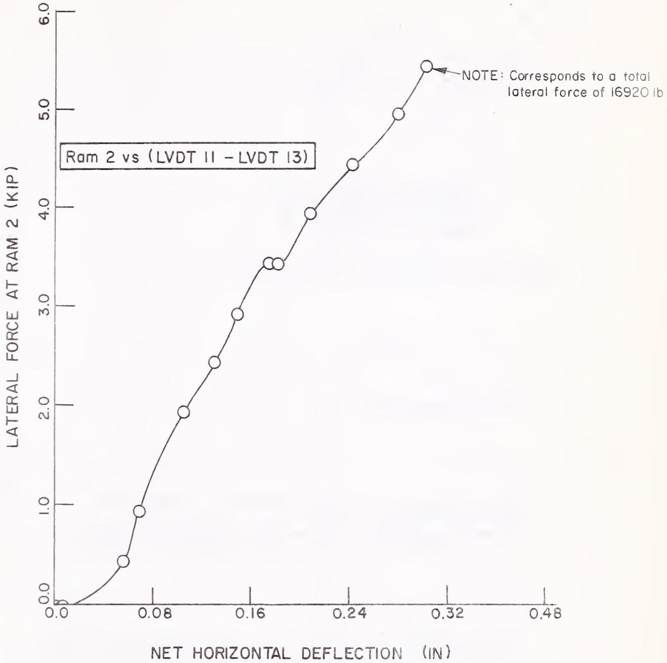
Figure 6.9 Lateral Force at Ram 2 versus Net Horizontal Deflection Along Plane 4 - Test 6
