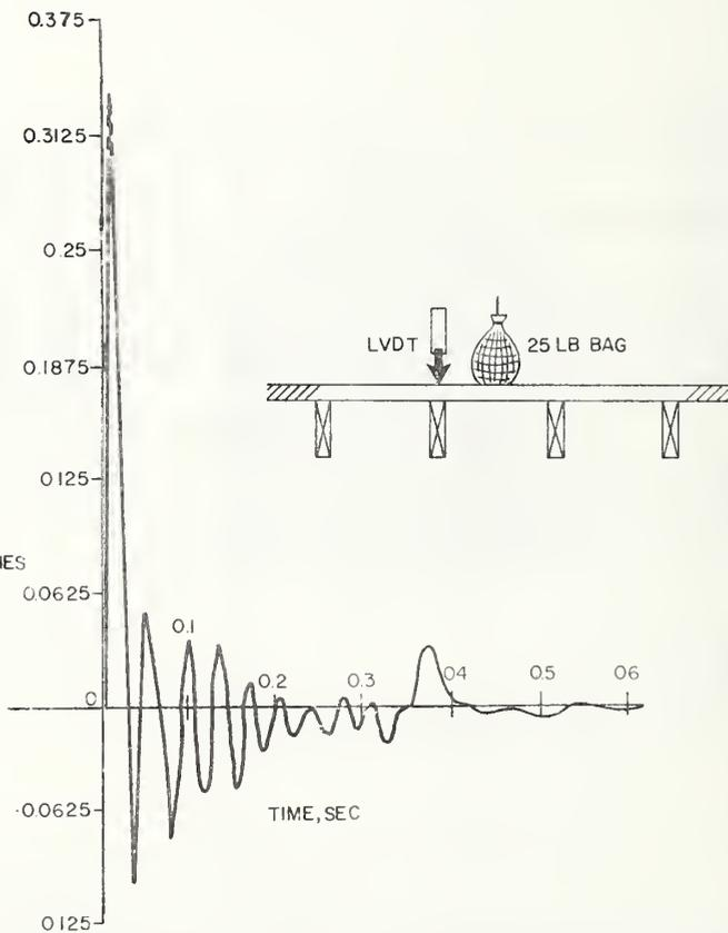
Figure 6.2 Deflection versus Time Traces for Tests 2A and 2B
