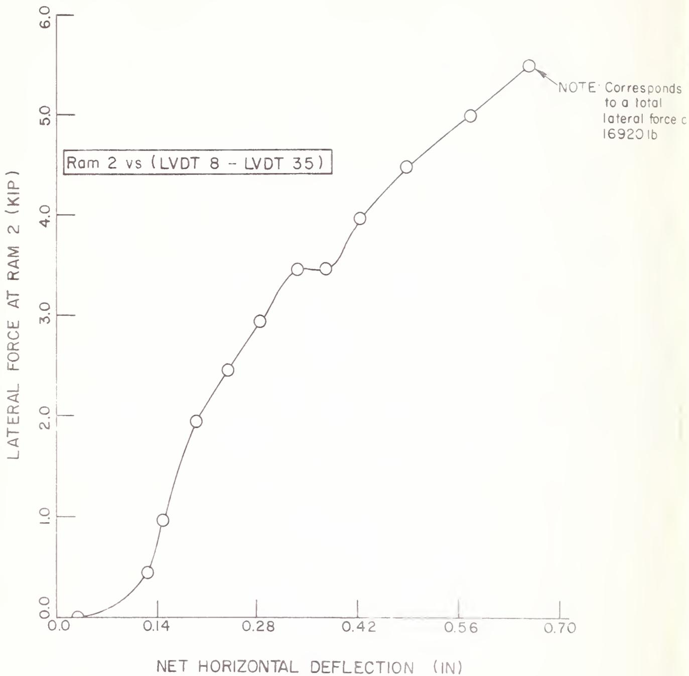
Figure 6.8 Lateral Force At Ram 2 versus Net Horizontal Deflection Along Plane 3 - Test 6
