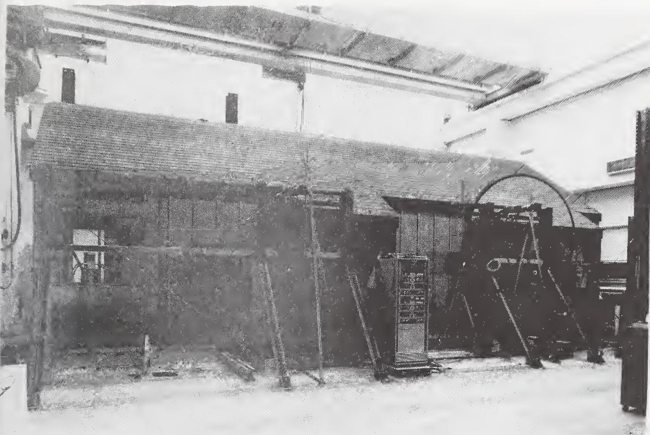
Figure 4.10 Test Setup for Repeated Racking
