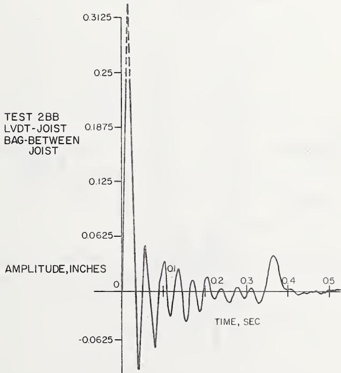
Figure 6.3 Deflection versus Time Traces for Tests 2AA and 2BB
