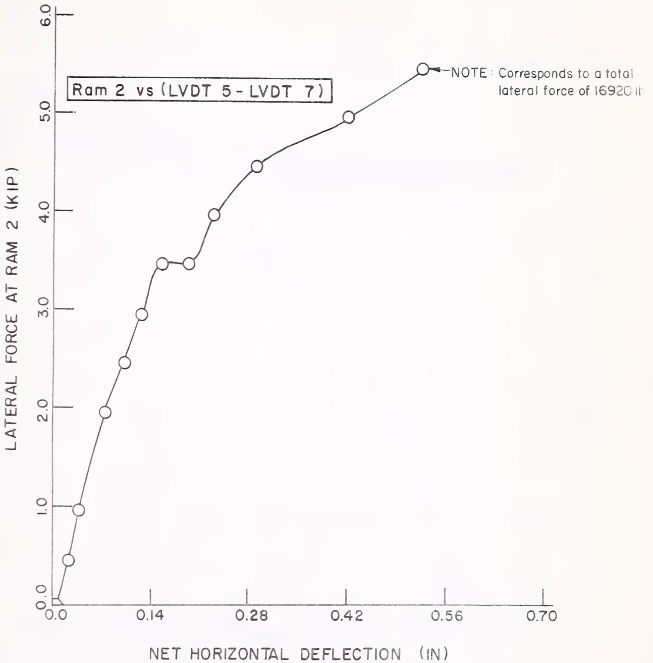
Figure 6.7 Lateral Force at Ram 2 versus Net Horizontal Deflection Along Plane 1 - Test 6
