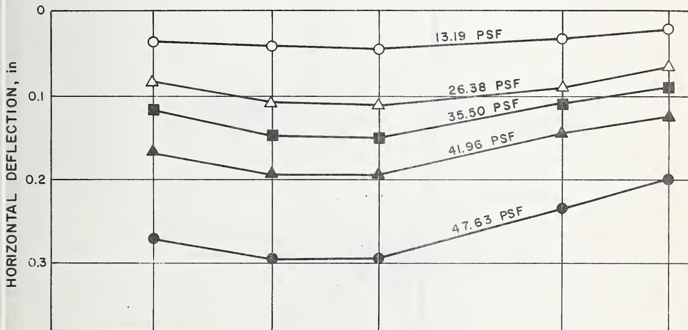
LATERAL DISPLACEMENT PROFILE ALONG TOP REAR OF MODULE
