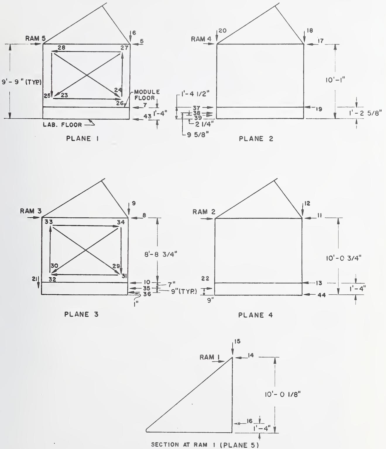
Figure 4.4 Cross Sections Showing Loading Rams and Instrumentation
