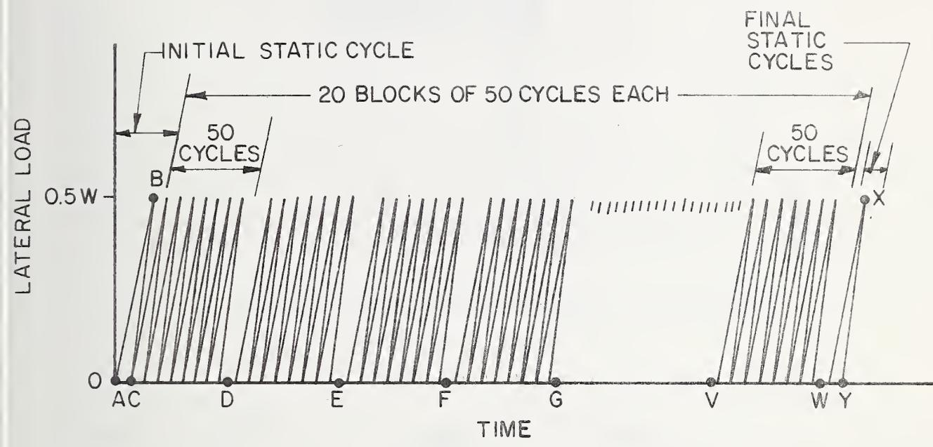
Figure 5.2 Loading Sequence for Test 4
