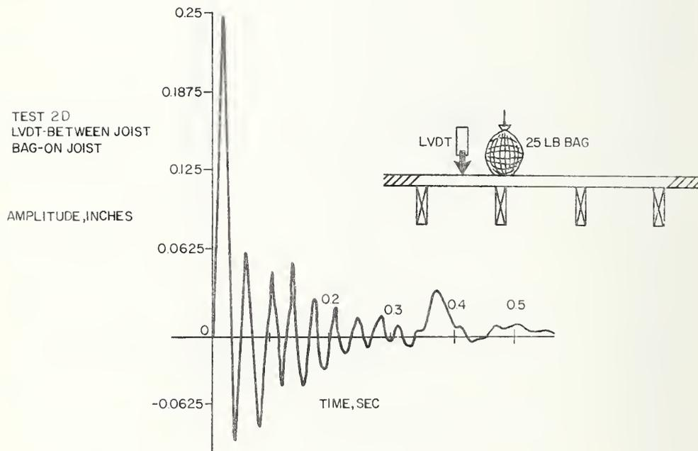
Figure 6.4 Deflection versus Time Traces for Tests 2C and 2D
