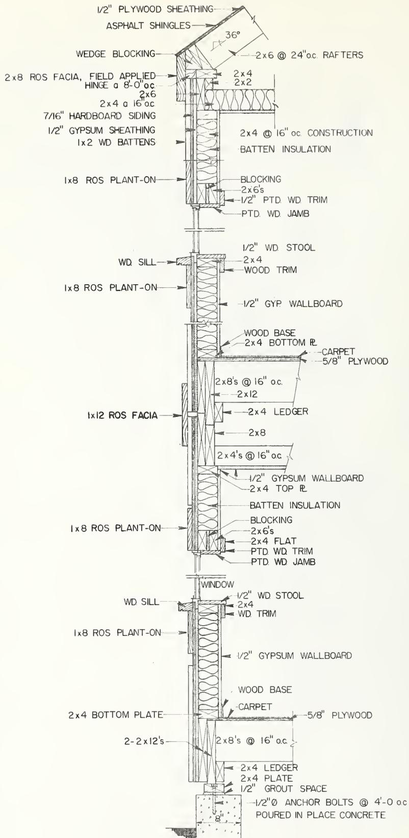
SECTION THROUGH EXTERIOR BEARING WALL
