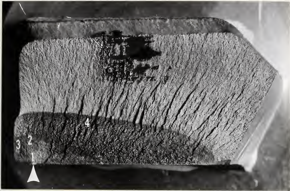
Figure 1. Fracture surface of the submitted part as received. Arrow indicates fracture origin. Numbers 1 through 4 indicate areas of the fracture surface examined with the scanning electron microscope. X 6
