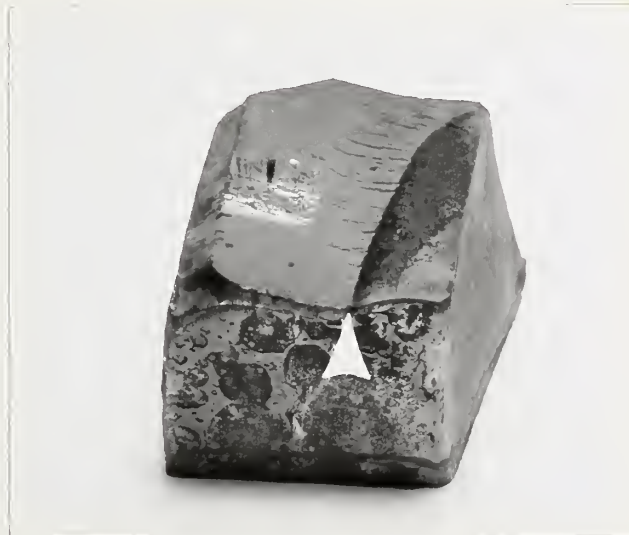
Figure 2. View of the fracture surface showing the change in the plane of the fracture at the junction (arrow) between the slower propagating part of the fracture and the faster propagating part of the fracture. X 3
