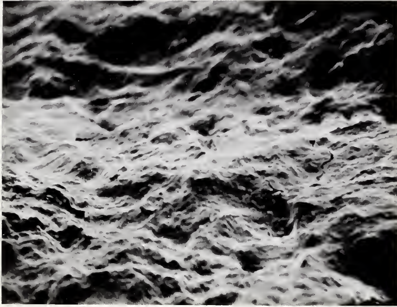
Figure 7. SEM from fracture surface at location 3, figure 1, showing what may be fatigue striations. X 1100
