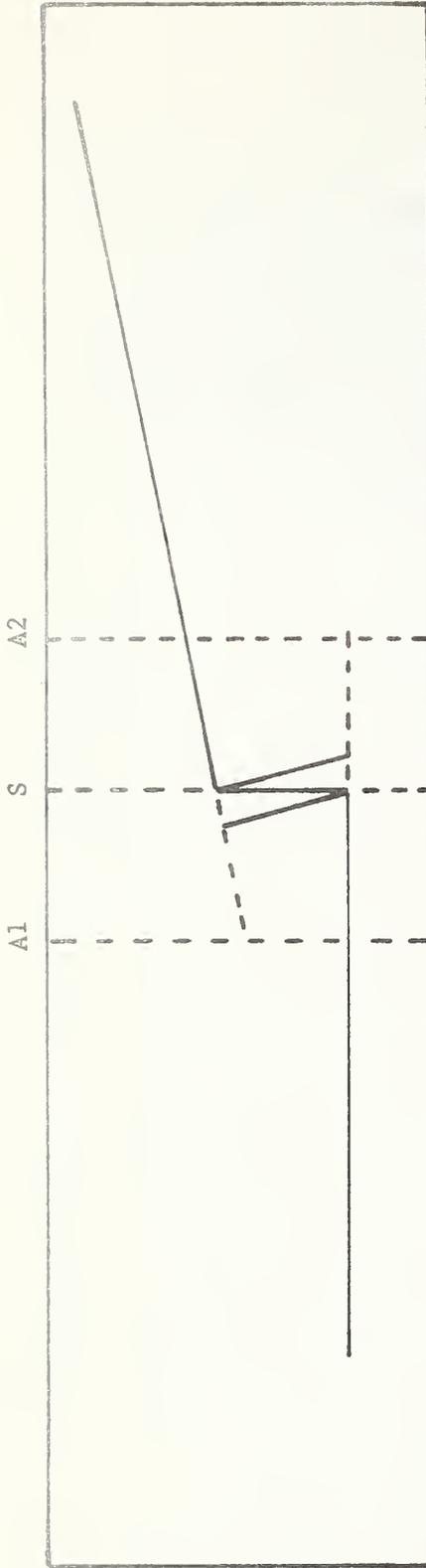
b) EFFECT OF IMPROPER SELECTION OF  $A_1$  AND  $A_2$  (NON-SYMMETRICALLY)
