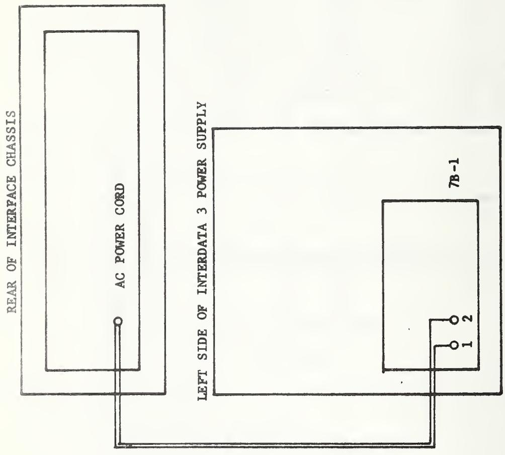
INTERFACE ELECTRONICS: AC POWER CONNECTION
