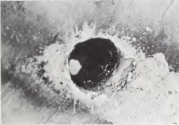
Figure 66. Close-up of Slab 5 Burning Bar Results
