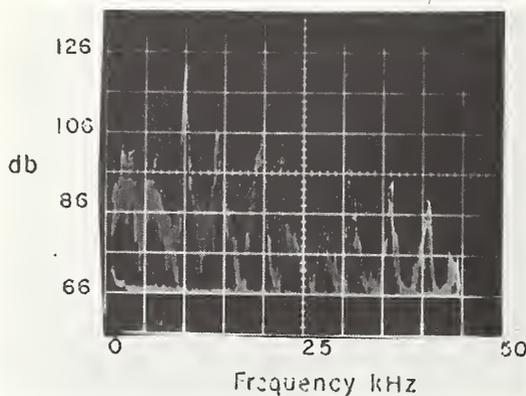
Figure 35. Acoustical Spectra of Rotohammer Drilling, Slab 2
