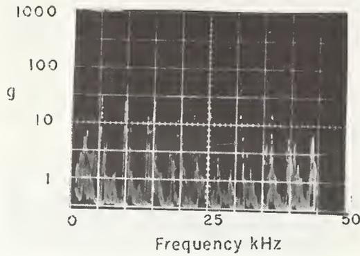
Figure 34. Vibrational Spectra from Rotohammer Drilling, Slab 2
