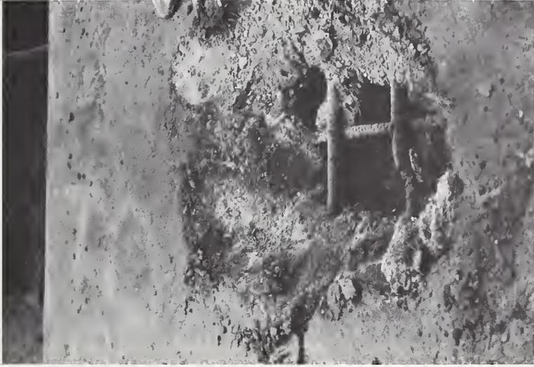
Figure 79. Opening Made in Fibrous Concrete by 18-minute Jackhammer Attack
