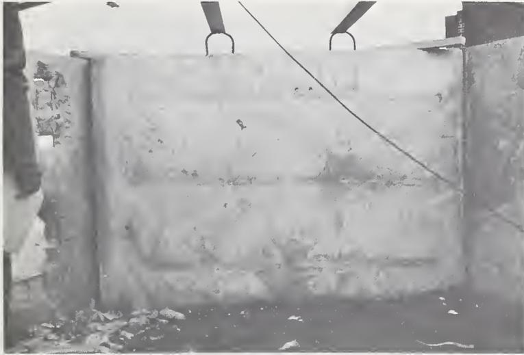
Figure 69. Interior Cracking Produced by JA-4
