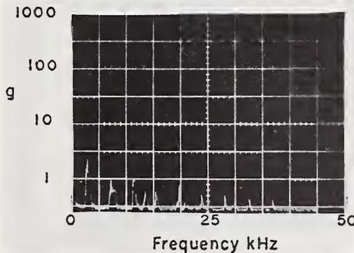
Figure 57. Vibration from 1" Drill
