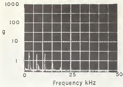
Figure 58. Vibration from 1-1/2" Drill
