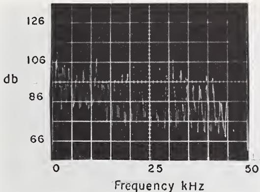
Figure 42. Acoustical Spectra from Demolition Saw
