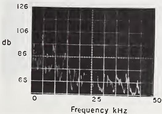
Figure 37. Acoustical Spectra from Rotohammer and Chisel on Slab 2
