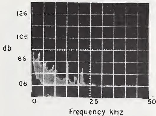
Figure 30. Acoustical Spectra of Cutting Torch
