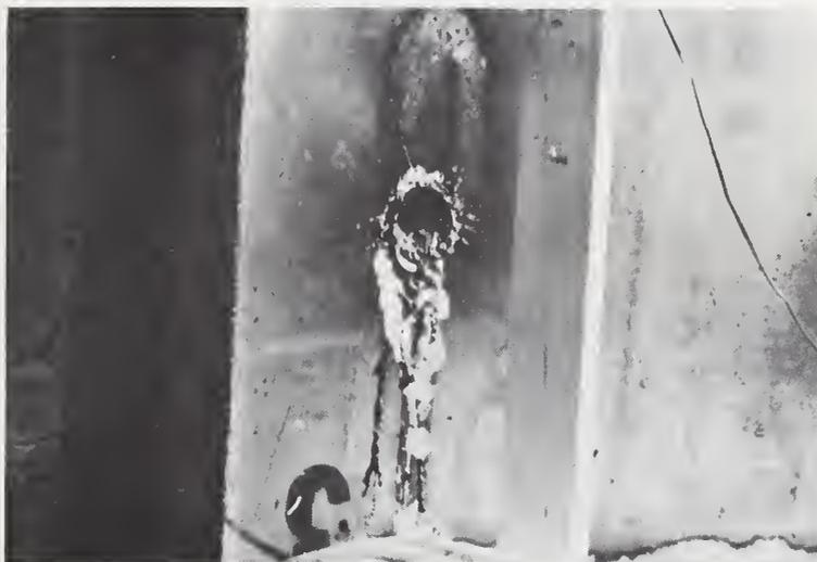
Figure 52. Attack 3D, Burning Bar Hole
