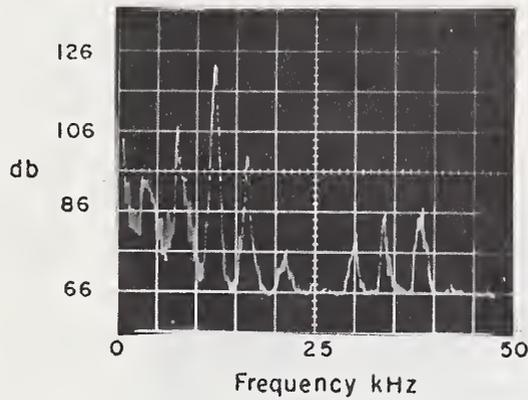
Figure 14. 1B1, Acoustical Disturbances from the Rotohammer and Drill
