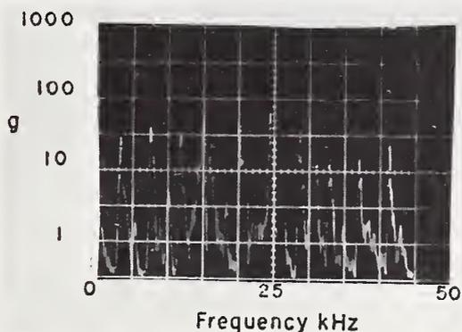
Figure 36. Vibrational Spectra from Rotohammer and Chisel on Slab 2
