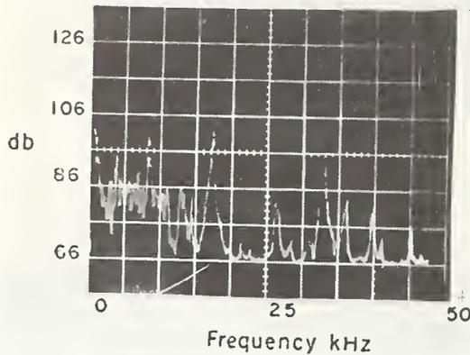
Figure 16. 1B2, Acoustical Disturbance from Rotohammer and Chisel
