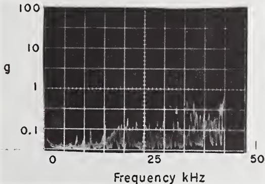
Figure 43. Vibrational Spectra from Demolition Saw
