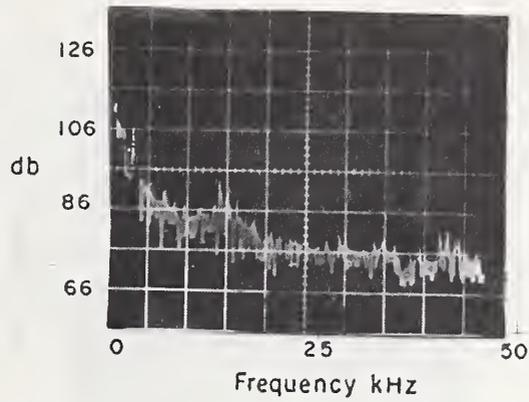
Figure 10. 1A3, Sound from Cutting Torch
