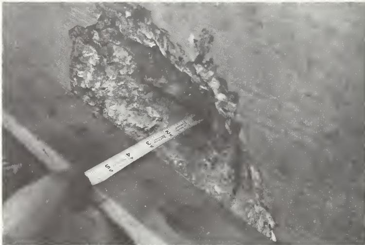
Figure 51. Spalling Produced by 12.10 Minutes of Attack by 16 lb. Sledgehammer
