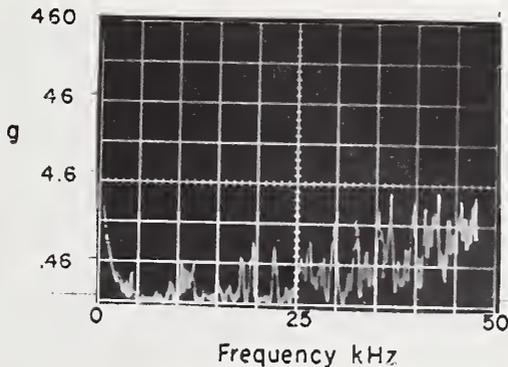
Figure 25. 1F1, Vibrational Disturbance from Demolition Saw and Abrasive Cutoff Wheel
