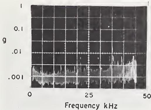
Figure 40. Vibrational Spectra from Burning Bar Attack on Slab 2
