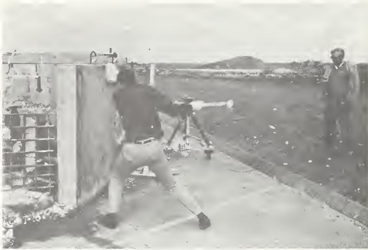
Figure 50. 16 lb. Sledgehammer Attack on Slab 3
