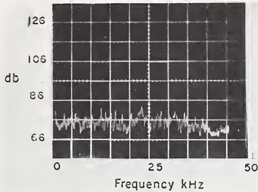
Figure 39. Acoustical Spectra from Burning Bar Attack on Slab 2
