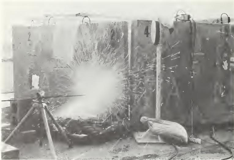
Figure 38. Burning Bar Attack on Slab 2
