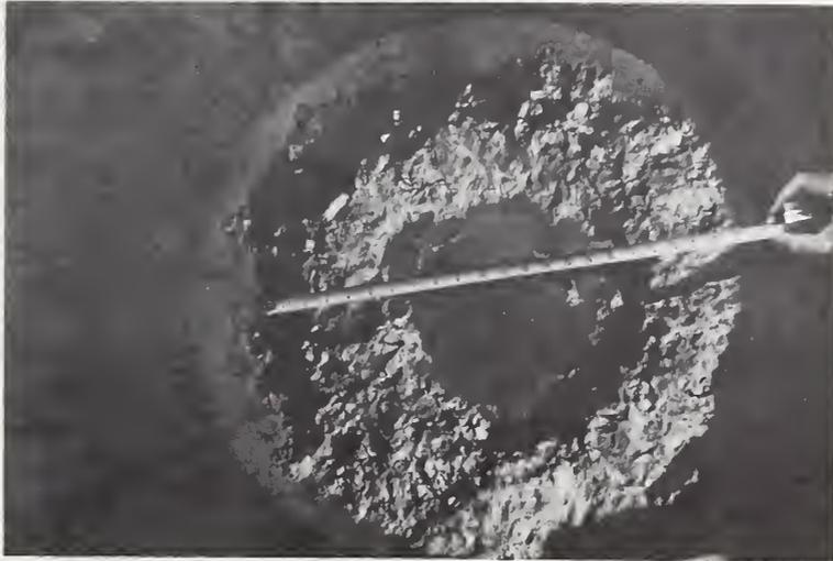
Figure 55. Exterior View of JA-4 Effects on Slab 3
