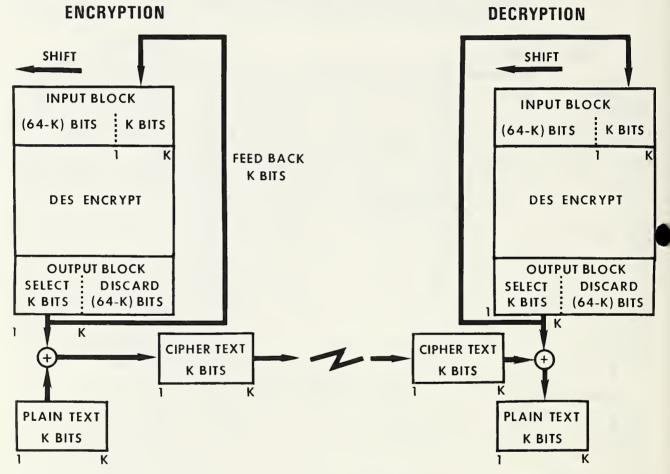
FIGURE 4: K-BIT OUTPUT FEEDBACK (OFB) MODE
