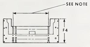
NOTE: 26 contacts on 0.100 inch (2.54 mm) spacing = 1.200 inches (30.48 mm)
