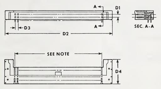
NOTE: 60 contacts on 0.100 inch (2.54 mm) spacing = 2.90 inches (73.66 mm)
