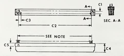
NOTE: 60 contacts on 0.050 inch (1.27 mm) staggered spacing = 2.950 inches (74.93 mm)
