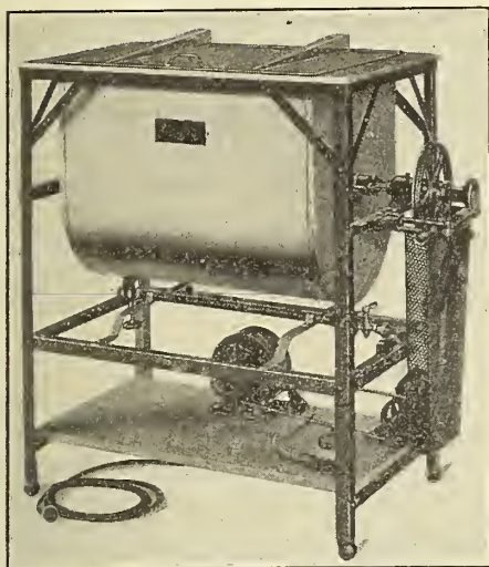
Commercial form of standard machine for testing fastness to washing
