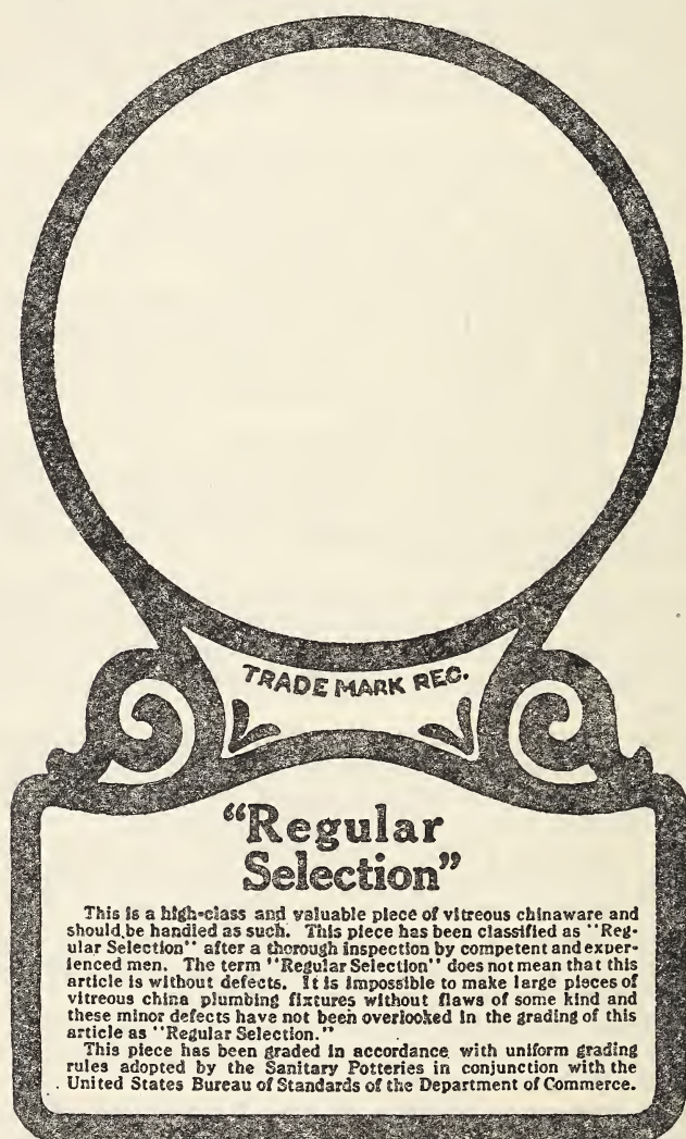
FIGURE 5.—Typical label used on regular selection vitreous china plumbing fixtures
