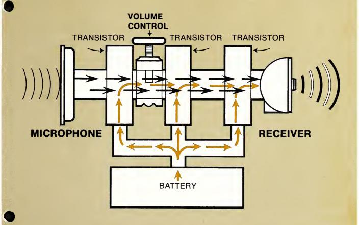
The system consists of a tiny *microphone* which picks up sound waves from the air and converts them into electrical signals, an *amplifier* which increases the strength of the electrical signals, a *battery* which provides electrical energy to operate the hearing aid, and a tiny loudspeaker called a "receiver" which converts the amplified signals back into sound waves and directs them into your ear through a specially fitted *ear mold*.
