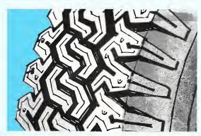
If studs are used, 100 studs per tire will probably be enough to do the job, and 150 studs per tire should be the maximum. A greater number will decrease traction on wet and dry pavements, exactly the opposite result from what you intended. You need enough rubber to grip dry pavement, and "sweep" a path through the water film on wet pavement.
