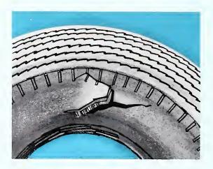
Various types of blow-out-and punctureresistant tires are on the market. Some have a steel safety belt underneath the tread. Some have an inner tire separated from the main body of the tire by an air space. Some use a sealant to prevent the escape of air if a tire is punctured. Some such feature is frequently a selling point in the "Premium Tire." In some tires of this type there is a tendency to increased heat buildup. Some others are difficult to balance satisfactorily.
