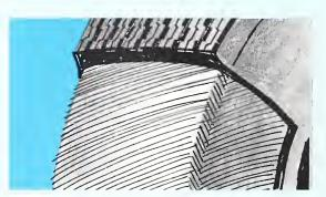
Rayon is the oldest of the manmade fibers. It has good strength, dimensional stability, and abrasion resistance, but it tends to degenerate if it is continually exposed to water. This could cause trouble in a tire if a cut exposed the fabric to the weather. This could be particularly troublesome if a cut went undetected in a wet season. Rayon does not flat spot.
