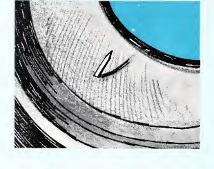
In a blow-out, the cord gives way and the tire deflates suddenly. After a blow-out a tire may not be reusable. Blow-outs may be caused by a slow weakening of the cord as a result of flexing, or by impacts with such things as rocks, pot holes or curbs. Blow-outs can be especially dangerous if they occur at high speed, or on a curve. A blow-out on a front tire produces a hard, steady pull; on the rear, a dangerous weaving motion.
