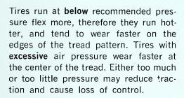
Unequal pressure, particularly in the front tires, can cause uneven braking—another possible cause of accidents.
