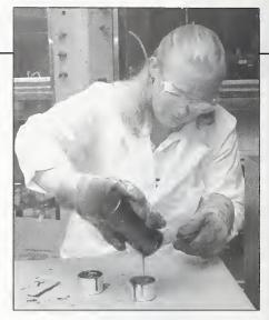
Kathryn Tice, AMRL research associate, is preparing hot performance graded asphalt binder test samples for placement in a pressured aging vessel for optimizing use in highway construction.
