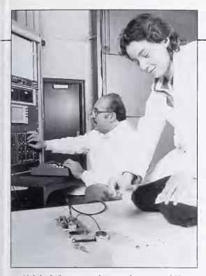
Nicholas J. Carino, research structural engineer, and Mary Sansalone, graduate student, are shown performing some of the initial tests that led to the development of the impactecho. Sansalone is about to create an impact by dropping a steel ball next to the point displacement transducer and Carino is ready to observe the resulting surface motion displayed on a waveform analyzer.
