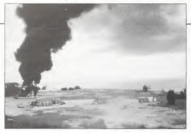
Crude oil burn at the U.S. Coast Guard Safety and Fire Test Detachment mesoscale burn facility in Mobile, Alabama.
