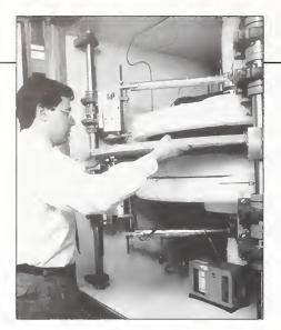
Robert Zarr, research mechanical engineer inserting an insulation sample in NIST's Line Heat Source Guarded Hot Plate, a large-capacity device for measuring the thermal resistance of insulation and other low-density materials up to 380 mm thick and 1 m in diameter. The Hot Plate provides calibrated specimens for guarded hot plates in other laboratories.
