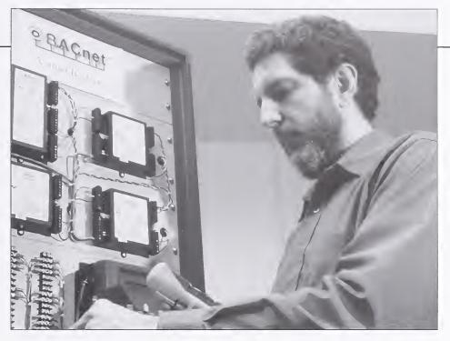
Steven Bushby, leader, Mechanical Systems and Control Group, checks wiring connections for controllers in the BACnetTM Virtual Building.
