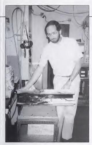
Thomas Ohlemiller, chemical engineer, examines the results of an experiment to characterize the smoldering combustion of blown-in cellulosic insulation in attic spaces.
