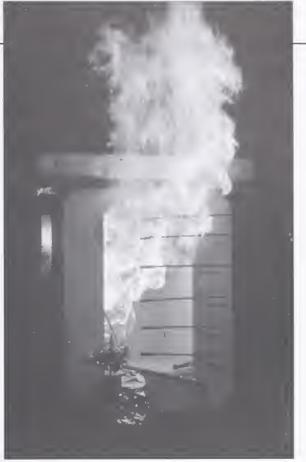
A scale model experiment used to investigate carbon monoxide formation during underventilated burning within an enclosure.
