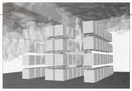
Computer simulation of a rack storage cartooned plastic commodity fire test using the NIST Large Eddy Simulated Fire Model.
