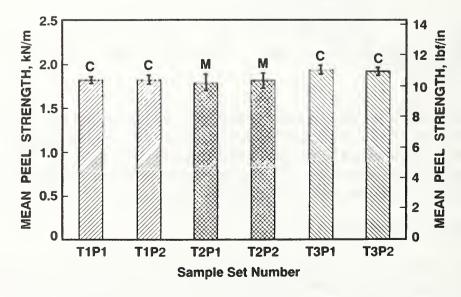
Figure C2. Mean peel strength of the sample sets prepared to examine TS1 tape variability. (T1, T2, and T3 indicate the three tapes, and P1 and P2 indicate the two primers; the failure modes are: C = cohesive and M = mixed cohesive/adhesive).
