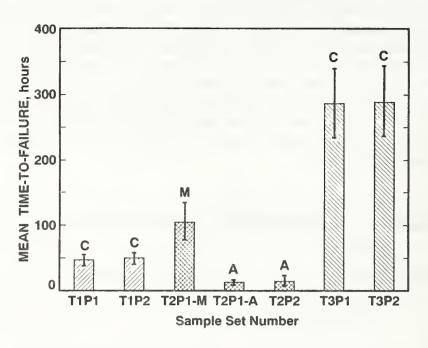
Figure C1. Mean times-to-failure of the sample sets prepared to examine TS1 tape variability. (T1, T2, and T3 indicate the three tapes, and P1 and P2 indicate the two primers; the failure modes are: C = cohesive, A = adhesive, and M = mixed cohesive/adhesive. In the case of T2P1, some specimens failed adhesively and some in a mixed mode; a distinction between the two groups is shown by the -M and -A after the T2P1 sample set number.)
