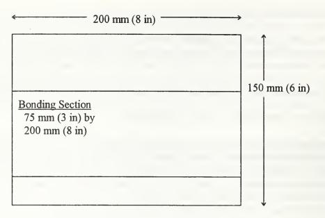
Figure A1. Plan view of a piece of EPDM used in specimen preparation.
