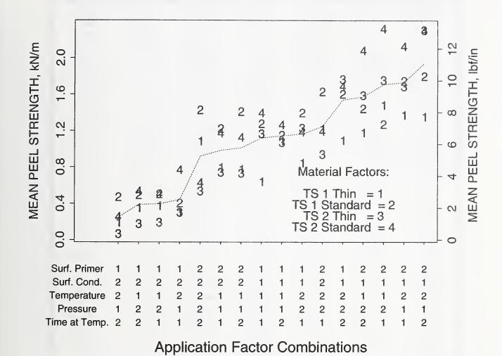
Figure 3. Mean Peel Strength Versus the Combinations of Application Factors. (Primer: Unprimed = 1, Primed = 2; EPDM Surface Condition: Clean = 1, Contaminated = 2; Application Temperature: Low = 1, High = 2; Application Pressure: Low = 1, High = 2; Time-at-Temperature: Short = 1, Long = 2.) The dotted line represents the mean for the four sample sets of tape-bonded specimens prepared at each combination of application factors.)
