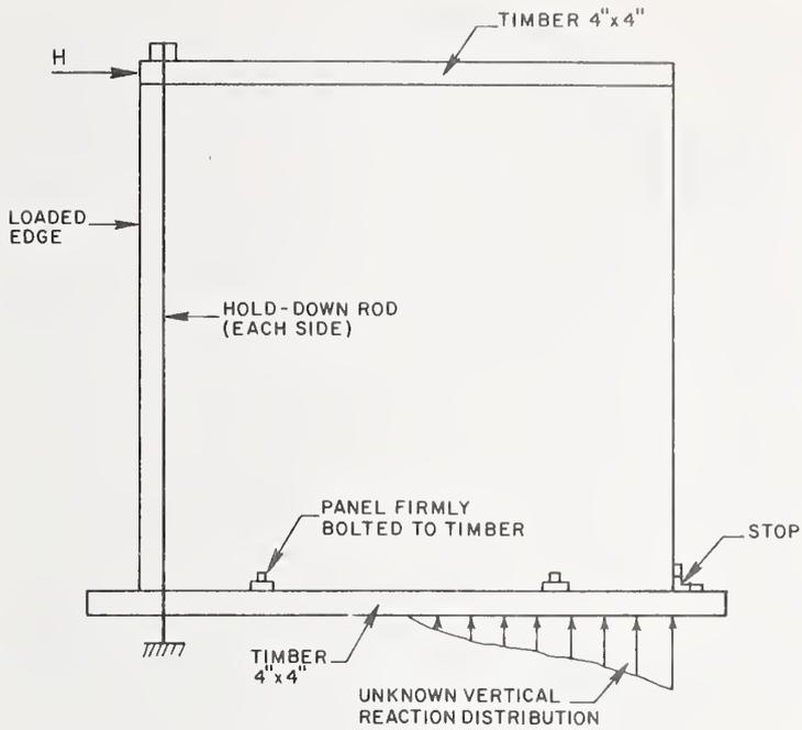
Figure 2.1 - ASTM Standard Method E72-74 [2].
