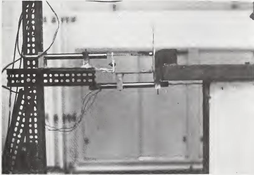
*Figure 3.11 - Closeup view of LVDT's 7 and 12.*
