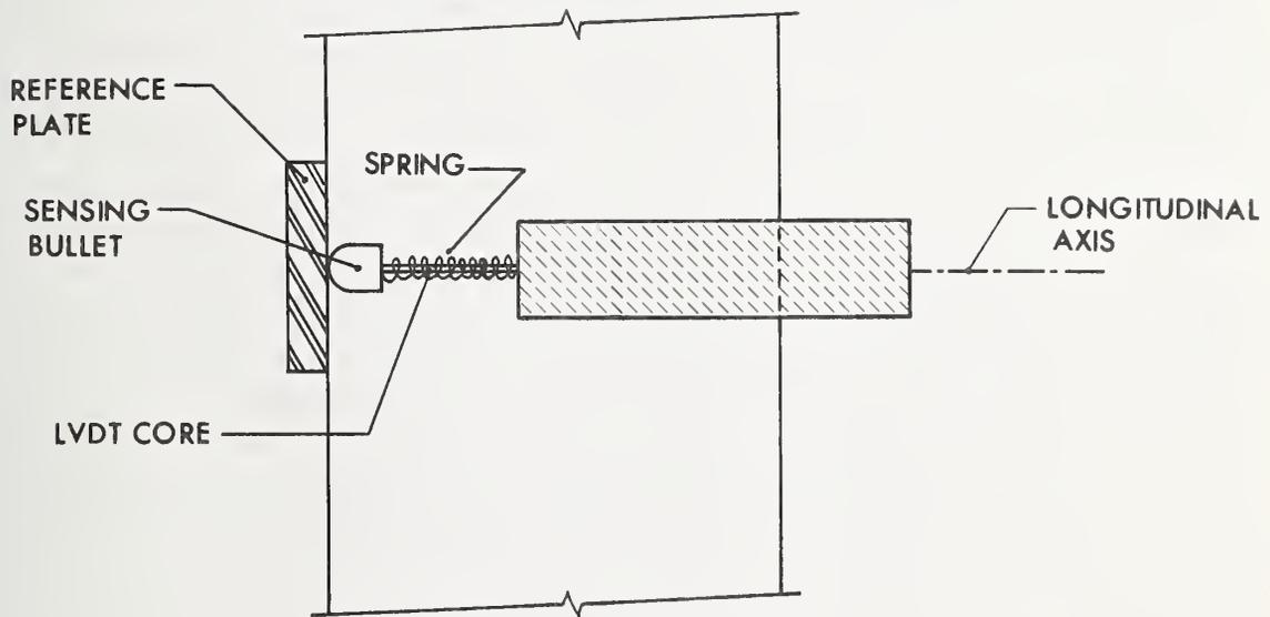
Figure 4.5 - Schematic of a typical LVDT.
