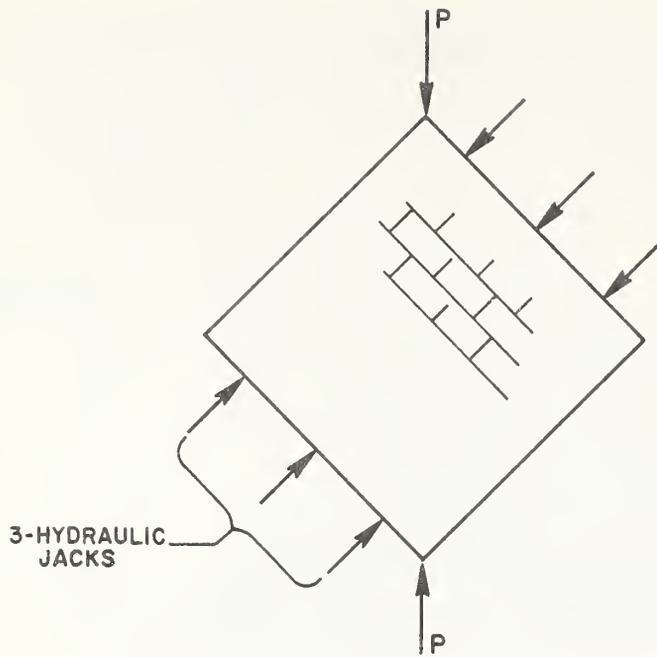
Figure 2.7 - Diagonal compression with uniform edge loading.
