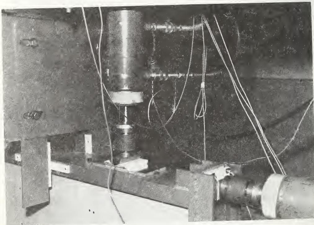
*Figure A.4 - Details of recommended bearing assembly.*
