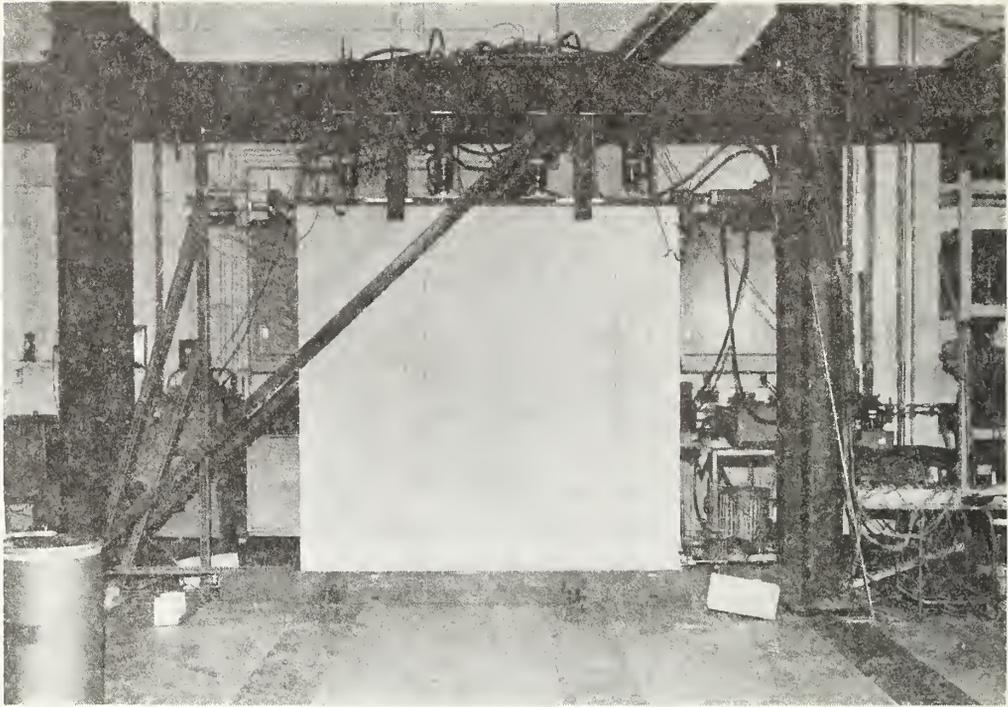
*Figure A.1 - Recommended test setup with dual hydraulic loading systems.*
