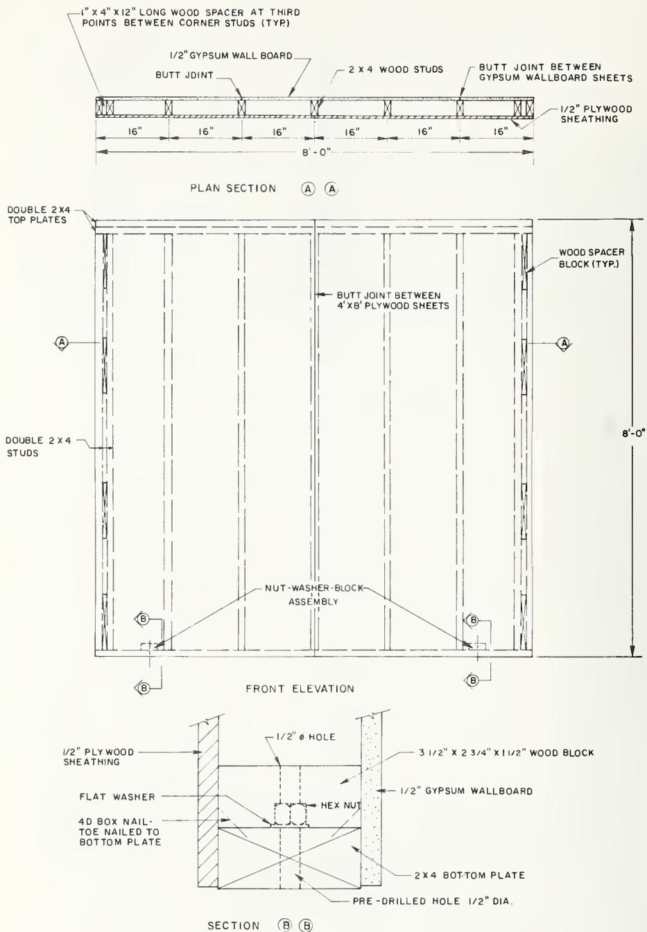
Figure 3.2 - Details of wood-frame test panel.
