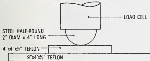
1. Improved rotation capability achieved, but point bearing caused gouging of teflon.
