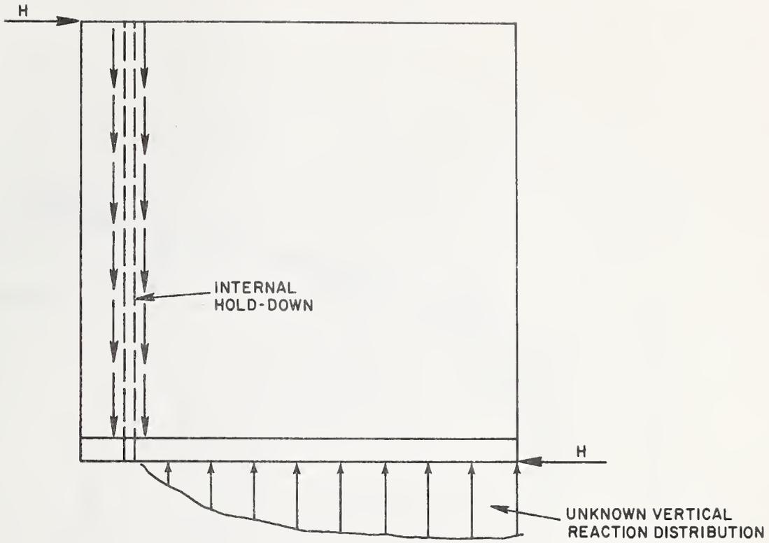
Figure 2.9 - Standard racking with internal hold-down.
