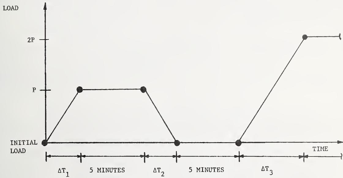
Figure A.5 - Load-time schematic diagram.
