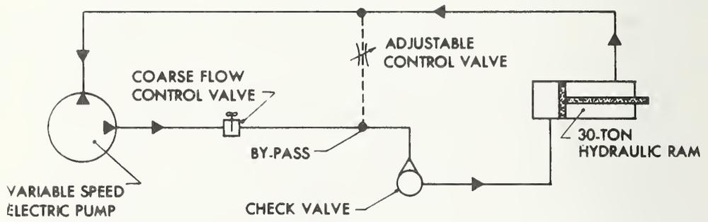
Figure 3.4 - Schematic of horizontal load hydraulic system.
