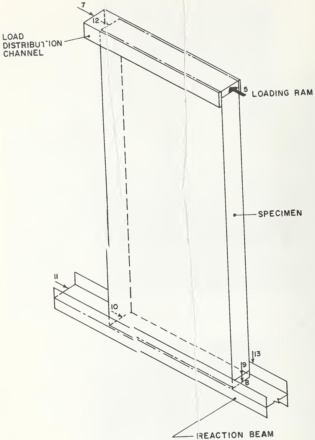
Figure 3.10 - Relative Locations of seven LVDT's.
