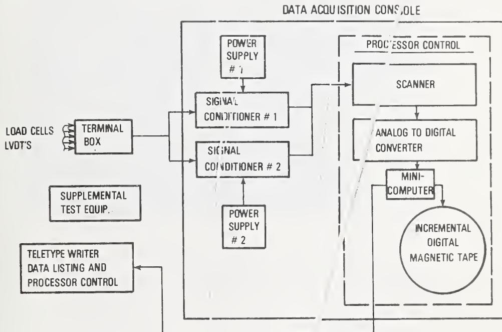
Figure 3.9 - Schematic of data acquisition system.
