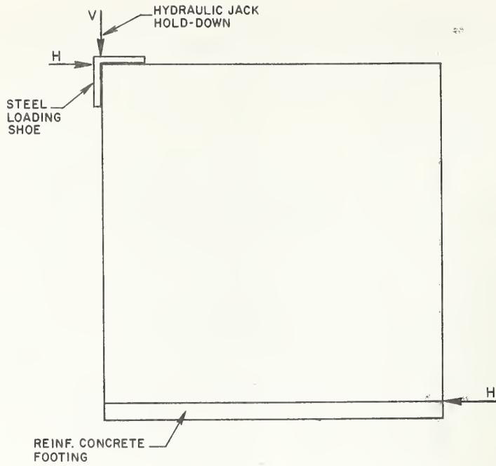
Figure 2.3 - Modified ASTM E72 method.
