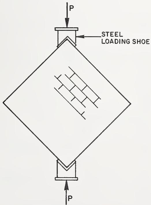
Figure 2.6 - Four by four diagonal compression loading.
