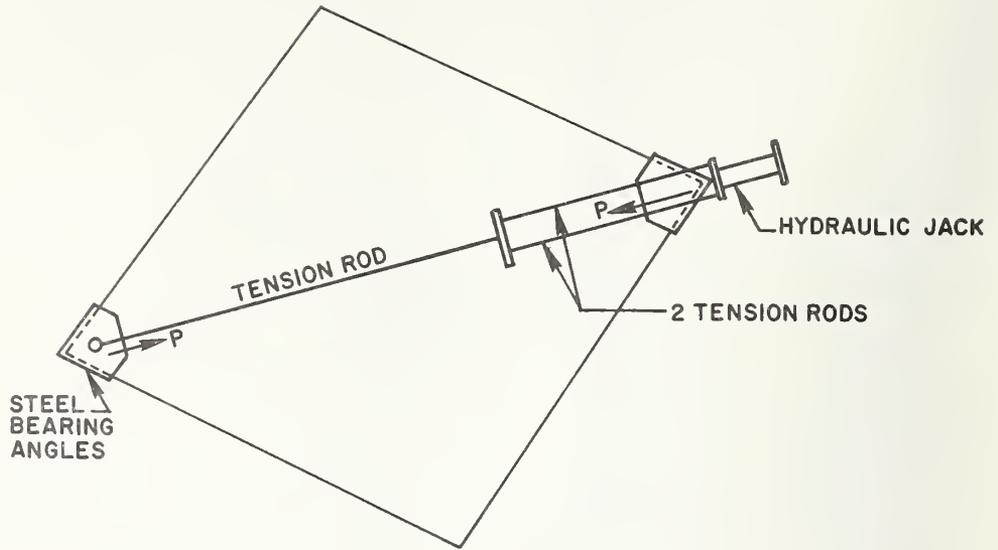
Figure 2.11 - Diagonal compression in horizontal plane.
