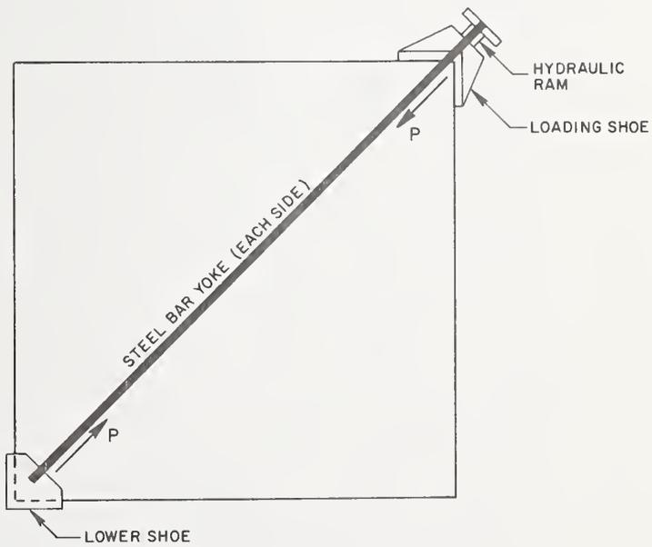
Figure 2.2 - Eight by eight diagonal compression loading.
