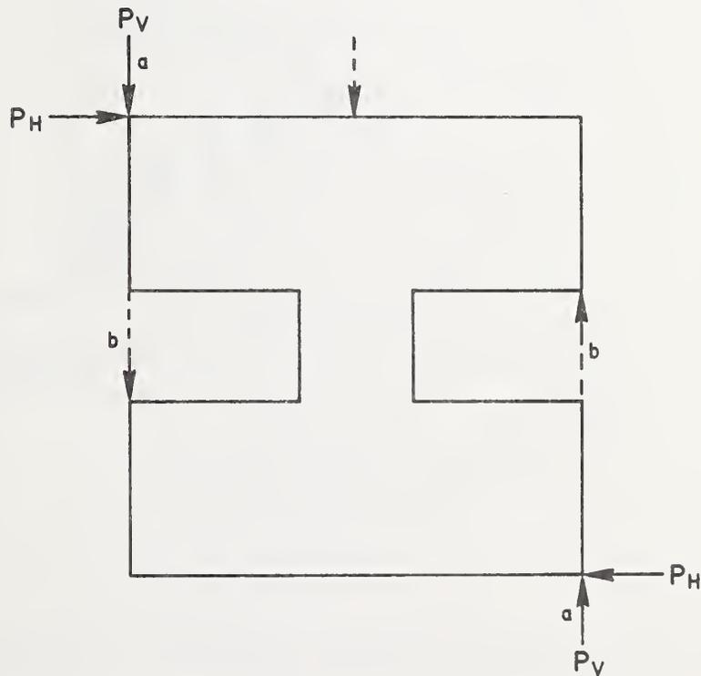
Figure 2.10 - Free body diagram of pier from masonry shear wall.
