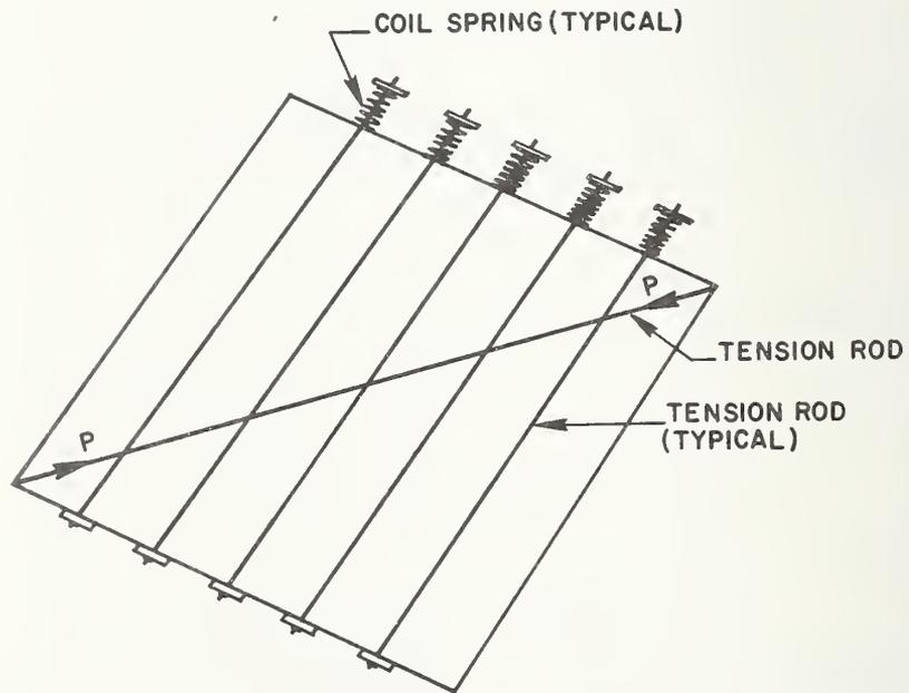
Figure 2.12 - Horizontal diagonal test with compressive edge loading.
