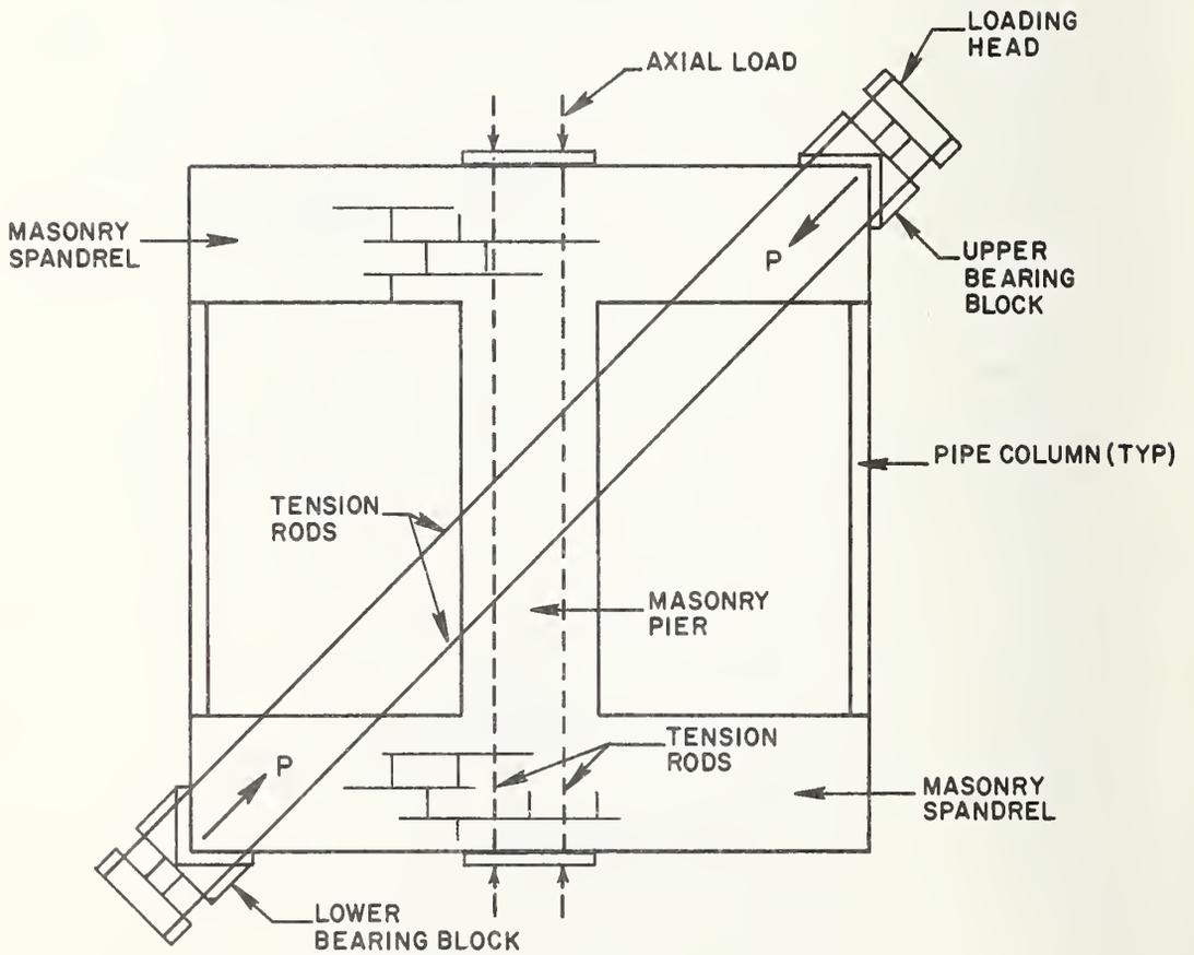
Figure 2.8 - Diagonal loading on masonry piers.
