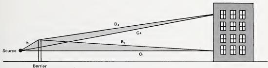
(b) Example of a building located far from a barrier, showing that the effect of receiver height on the attenuation is minimal.
