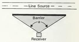
Figure 5.1–8. Barrier Geometry Showing the Included Angle, a.
