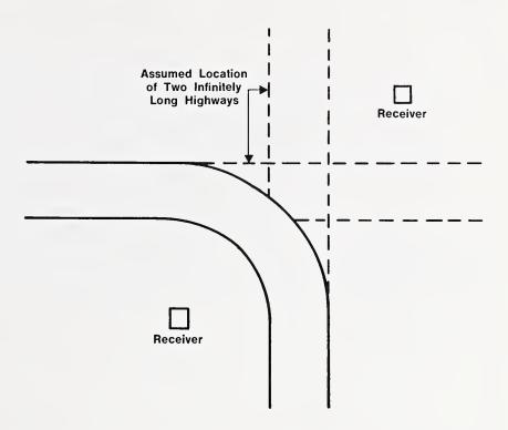
Figure 5.2-2. Example of a Highly Curved Highway.
