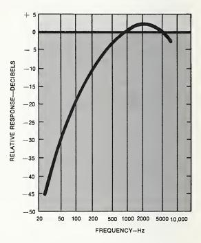
Figure 3–1. Frequency Response Curve for A-weighting [1, 2, 3].
