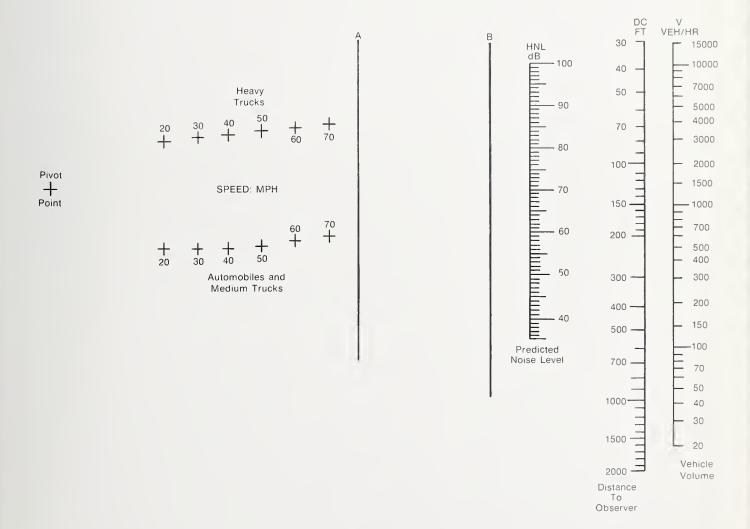
Figure 5.2–1. Highway Noise Prediction Nomogram [3].
