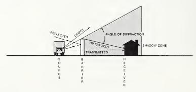
Figure 5.1-5. Paths along which sound energy can travel from the source to the receiver [2]. Also shown is the shadow
