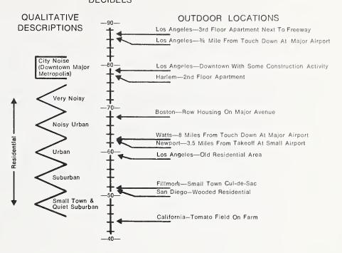
Figure 3–3. Examples of Outdoor Day-Night Equivalent Sound Levels Measured at Various Locations [4].
