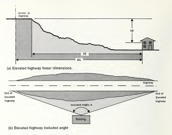
Figure 5.2-8. Elevated Highway Dimensions.
