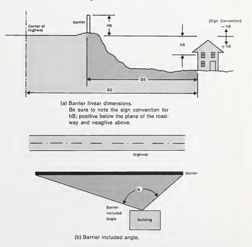
Figure 5.2-7. Highway Barrier Dimensions.
