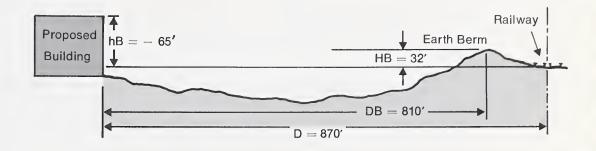
Figure 5.5-11. Cross-Section Showing Railway Earth Berm.
