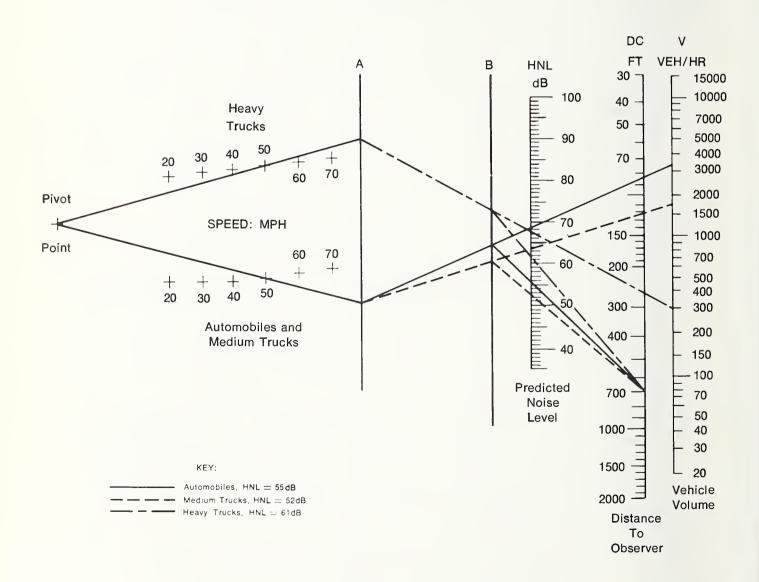
Figure 5.5-7. Highway Noise Nomogram for Highway #1 of Example.
