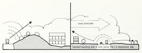
Figure 7–2. Use of Natural Noise Figure 7–3. Selection of Building Sites Barriers. Relative to Wind Direction.
