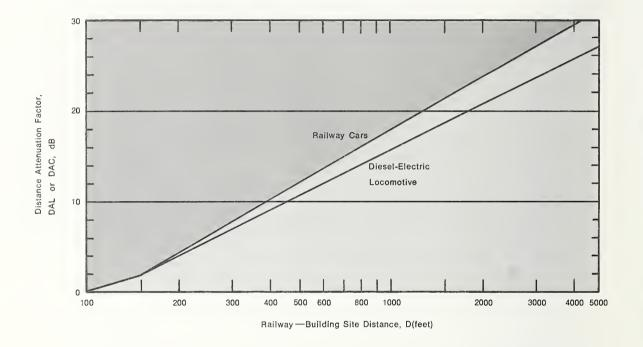
Figure 5.3-9. Railway Noise Attenuation With Distance [1].
