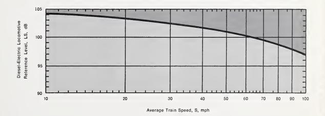
Figure 5.3-8. Diesel-Electric Locomotive Reference Level, LS, at 100 feet [1].
