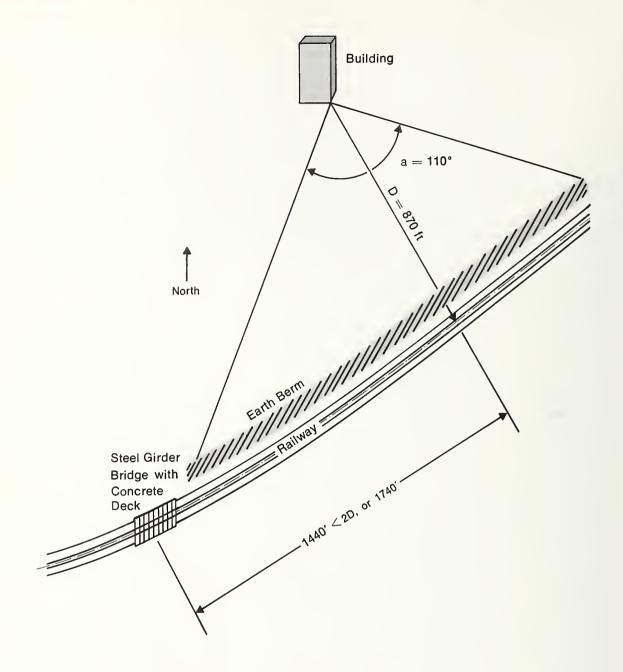
Figure 5.5-8. Local Map Showing Details of Railway.
