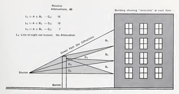
(a) Example of a building located close to a barrier, showing the change in attenuation for receiver locations at each floor.
