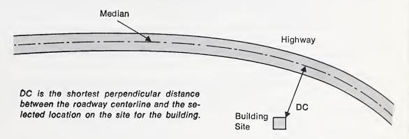
Figure 5.2-6. Determination of Roadway—Building Site Distance, DC.
