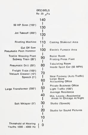
Figure 3–2. Typical A-weighted Sound Pressure Levels [4].
