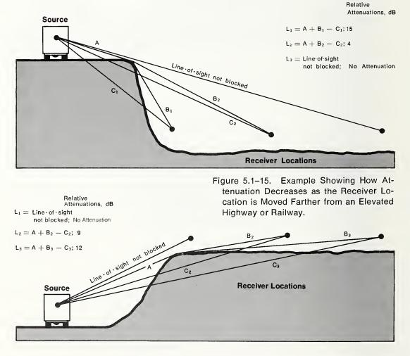
Figure 5.1–16. Example Showing How Attenuation Increases as the Receiver Location is Moved Farther from a Depressed Highway or Railway.
