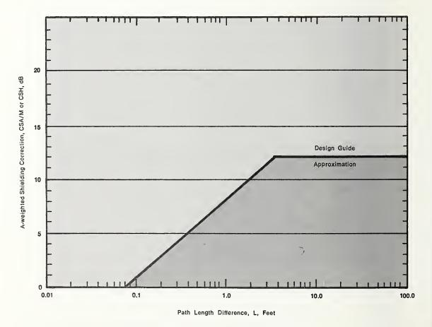
Figure 5.2–11. A-weighted Shielding Correction for Barriers.
