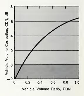
Figure 5.2–10. Vehicle Volume Correction Factor, CDN.
