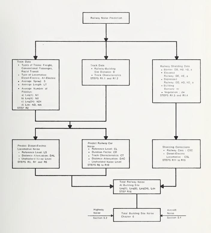
Figure 5.3-1. Railway Noise Prediction Flow Diagram.
