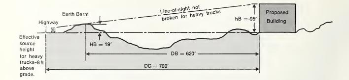
Figure 5.5-5. Cross-section Showing Highway #1 and Earth Berm.
