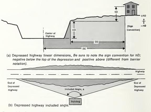
Figure 5.2-9. Depressed Highway Dimensions.
