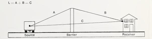
Figure 5.1-9. Barrier Path Length Difference.
