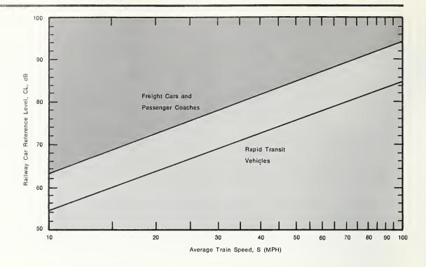
Figure 5.3-11. Railway Car Reference Level at 100 feet [2].
