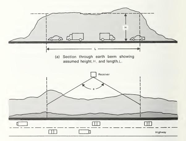
(b) Top view of berm showing the assumed included angle, a.
