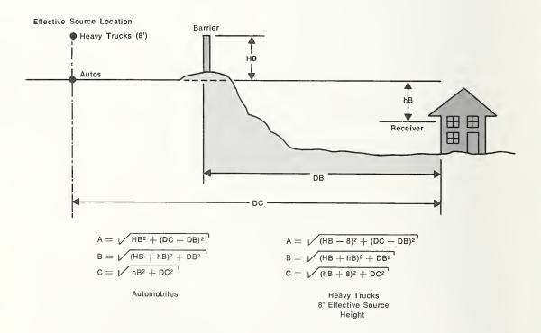
Figure 5.1–12. Example Showing Horizontal and Vertical Dimensions of Source, Barrier, and Receiver Geometry and Equations for A, B and C.
