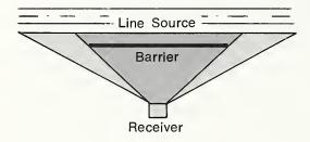
Figure 5.1–7. Paths for Sound Energy to Travel Around the Ends of a Barrier.
