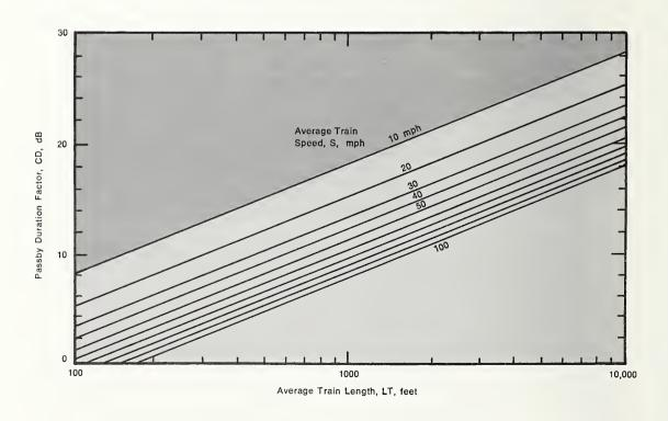
Figure 5.3–12. Duration Correction for Train Passbys.
