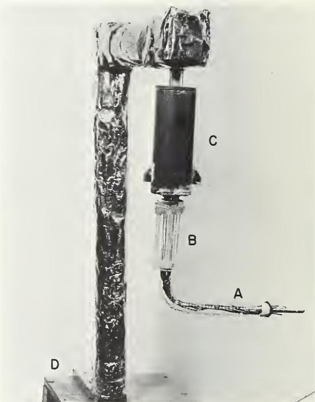
FIGURE 1. The probe housing two thermocouples, two thermistors, and a resistance thermometer. The ice-bath for the thermocouples is housed in the cabinet in the lower portion of the figure. Conduction errors were minimized with the use of the cage-like structure housing the bare lead wires.
