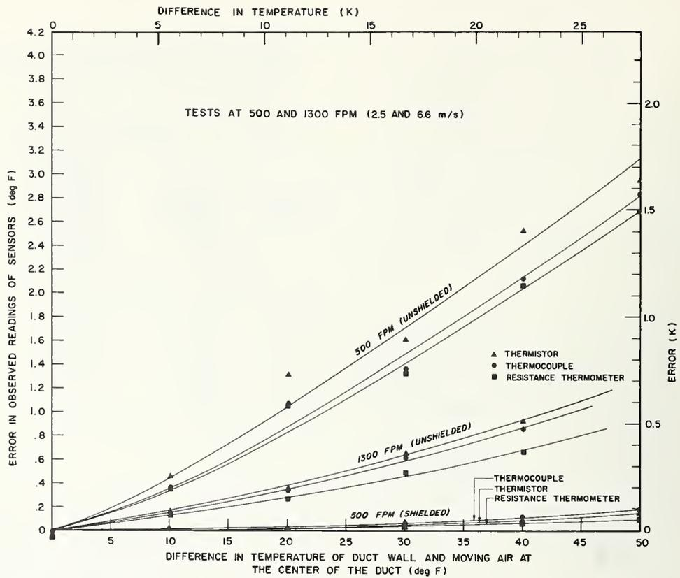
FIGURE 10. Observed radiation error for the three types of sensors in the test probe, when used in air having velocities of 500 and 1300 fpm.
