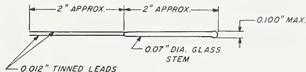
FIGURE 3. Physical dimensions of each of the thermistors.
