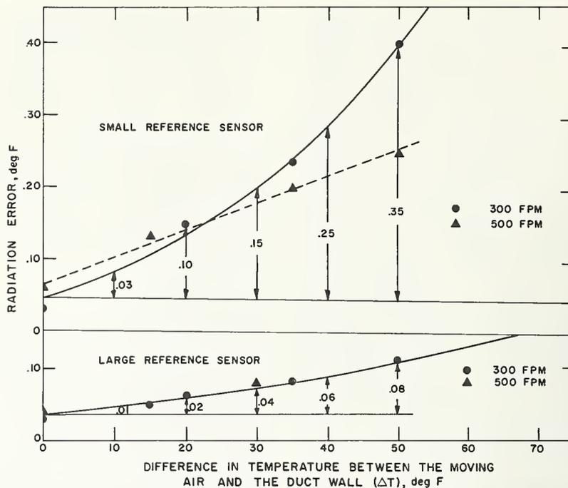
FIGURE 8. Errors in the two reference sensors as a function of the difference in temperature between the duct wall and the air at the reference sensors.
