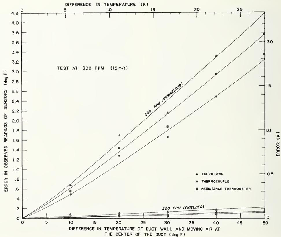
FIGURE 11. Observed radiation error for the three types of sensors in the test probe, when used in air having a velocity of 300 fpm.
