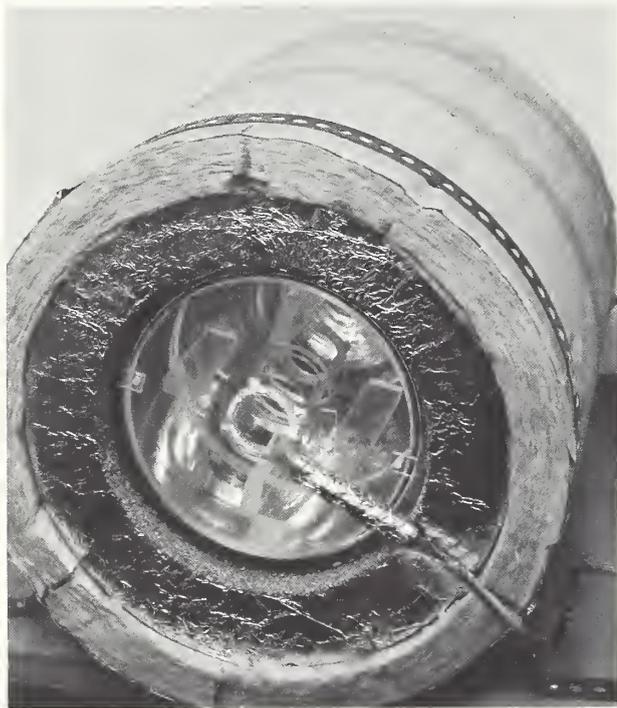
FIGURE 7. Calibration chamber for calibrating the thermistors, thermocouples, and the two reference sensors in still air.
