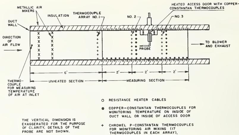
FIGURE 4. Schematic diagram of duct and associated air-mixing, heating, and temperature-sensing equipment.
