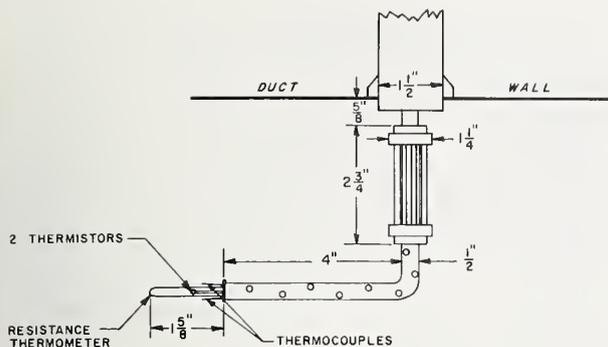
FIGURE 2. Diagram of the probe-end showing the two thermocouples, one of the two thermistors, and the capsule-type platinum resistance thermometer.
