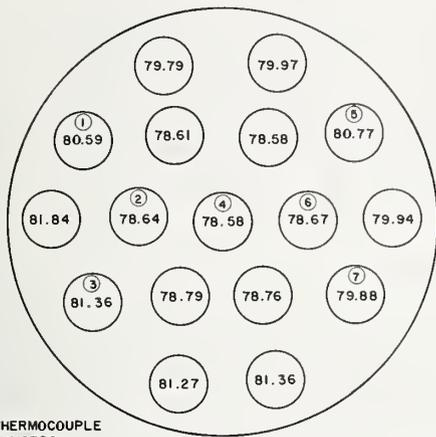
FIGURE 9. Map of air-temperatures in Fahrenheit degrees of a cross-sectional area during a typical test when  $\Delta t = 40$  deg F.
