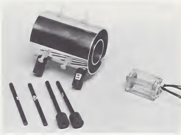
FIGURE 6. Small shield and the reference sensor used in tests where the test probe was unshielded. Removable legs for the shield are shown in lower left.
