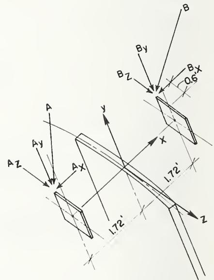
(d) Configuration of cathead leg reactions relative to shell.
