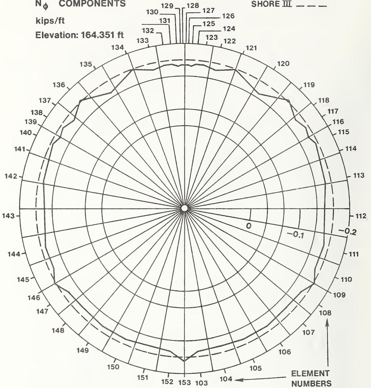
Figure B.4 Comparison of  $N_{\phi}$  from gravity load, load case 1
