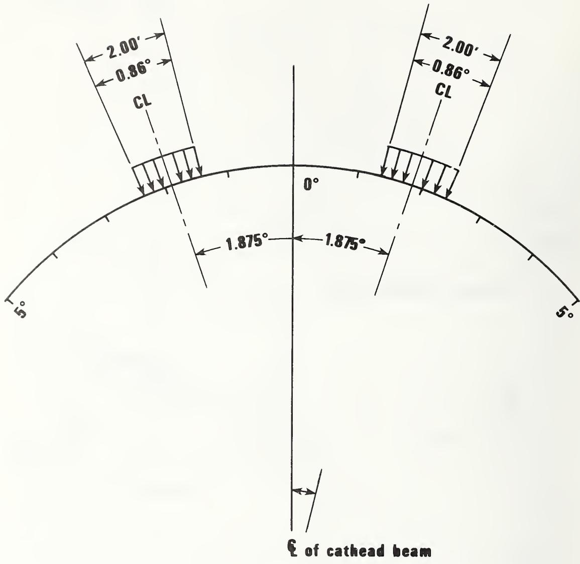
Figure 6.18 Normal force ( $F_x$ ) at cathead for load case 4
