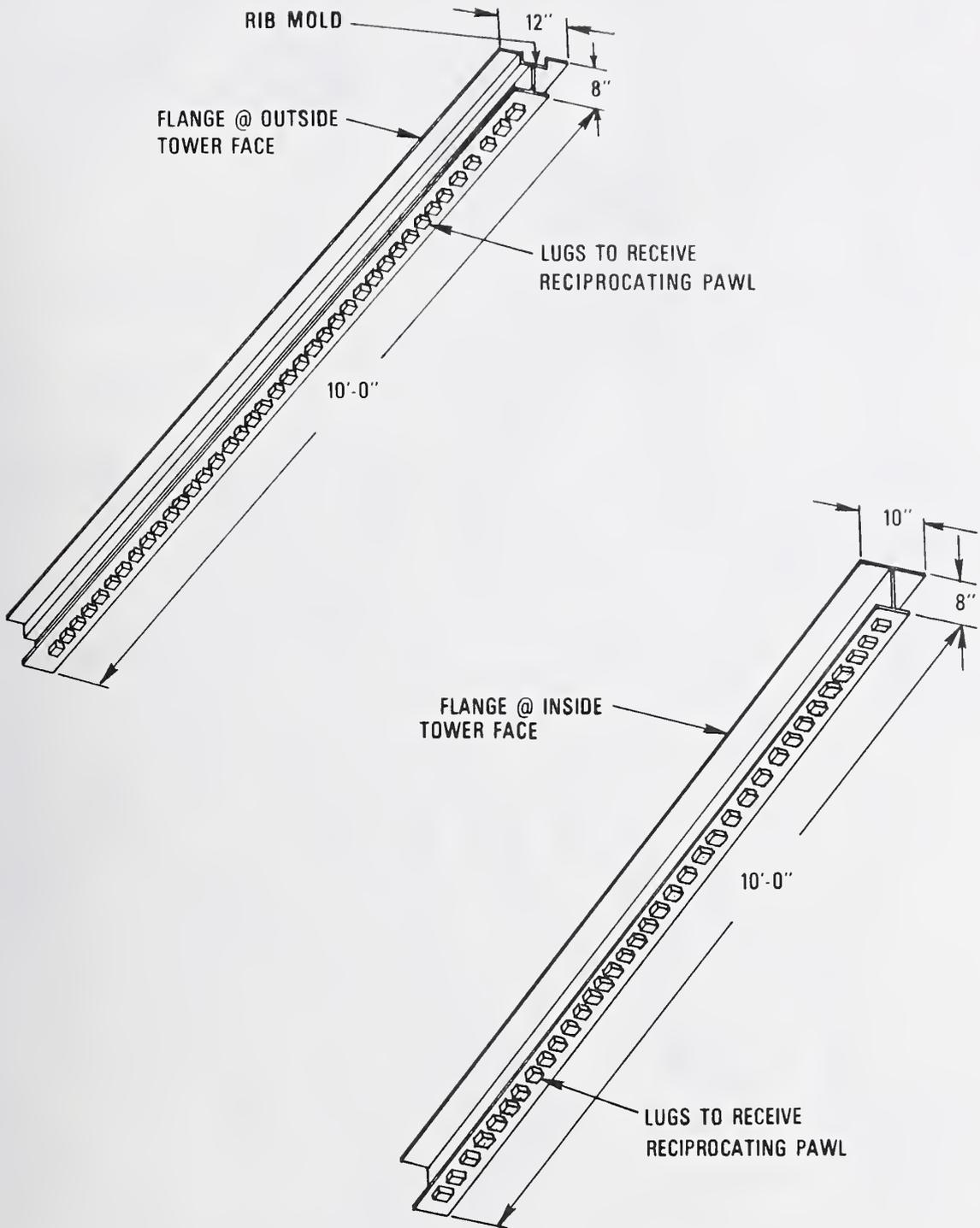
Figure 2.7 Jumpform beam detail
