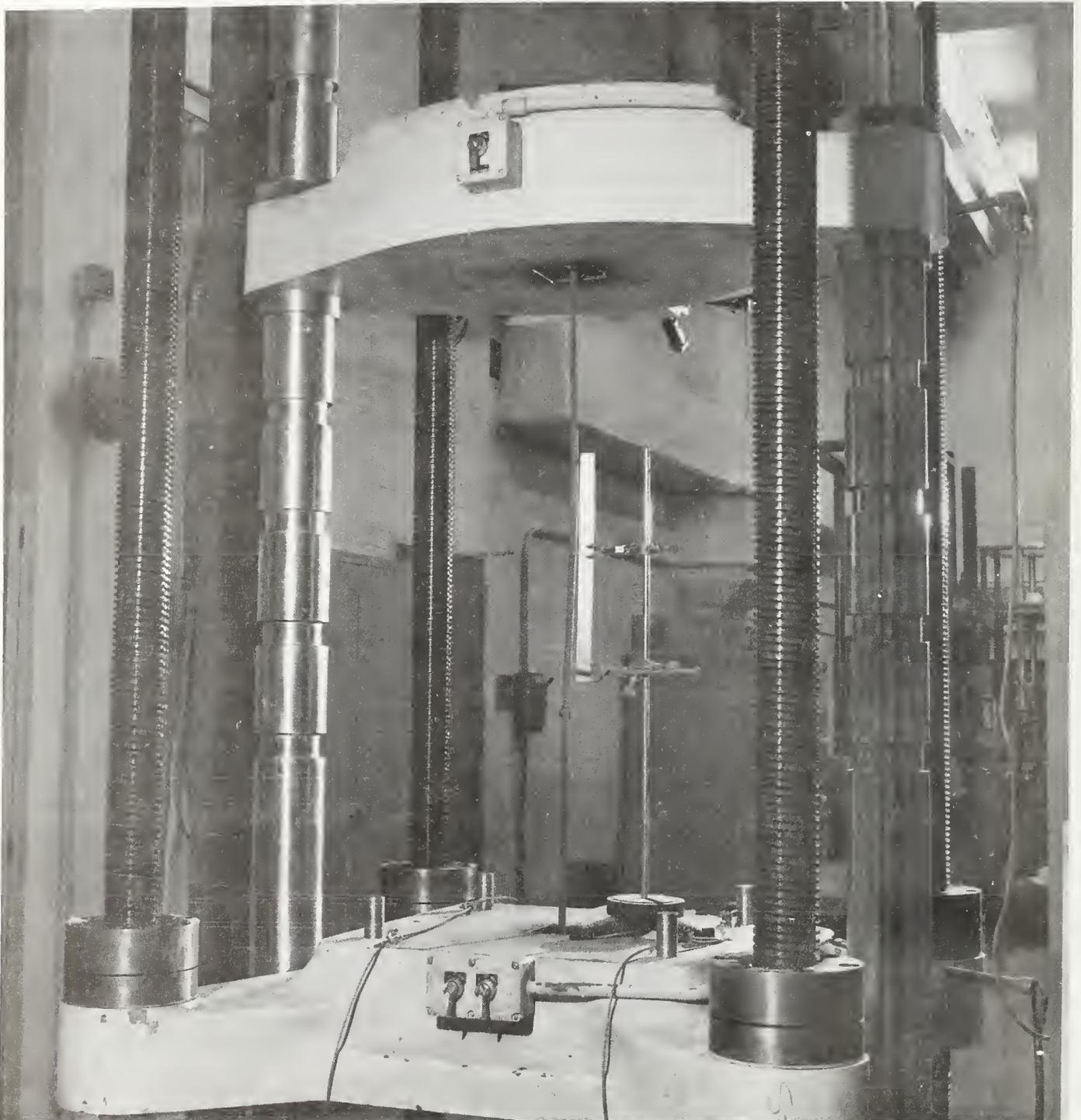
Figure 4.12 Tension Test Setup for Wire Rope
