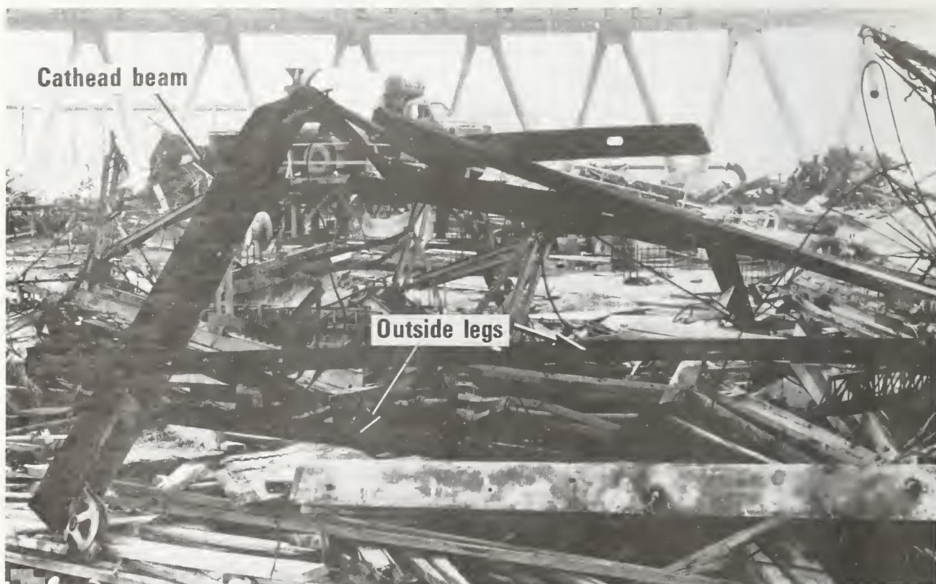
Figure 3.16 Outside Legs of Cathead Gantry No. 4
