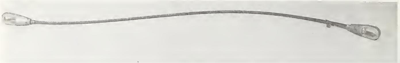
Figure 4.11 Typical Wire Rope Test Specimen
