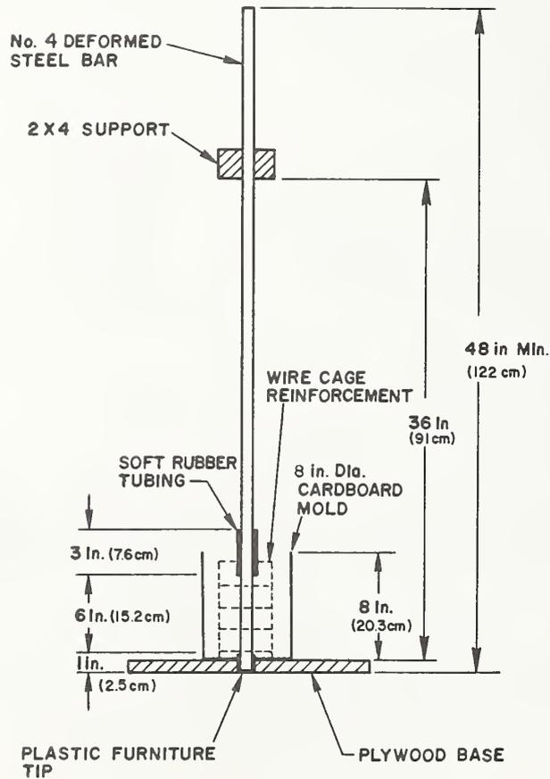
Figure 4.6 Section Through Pull-out Specimen Rack and Mold
