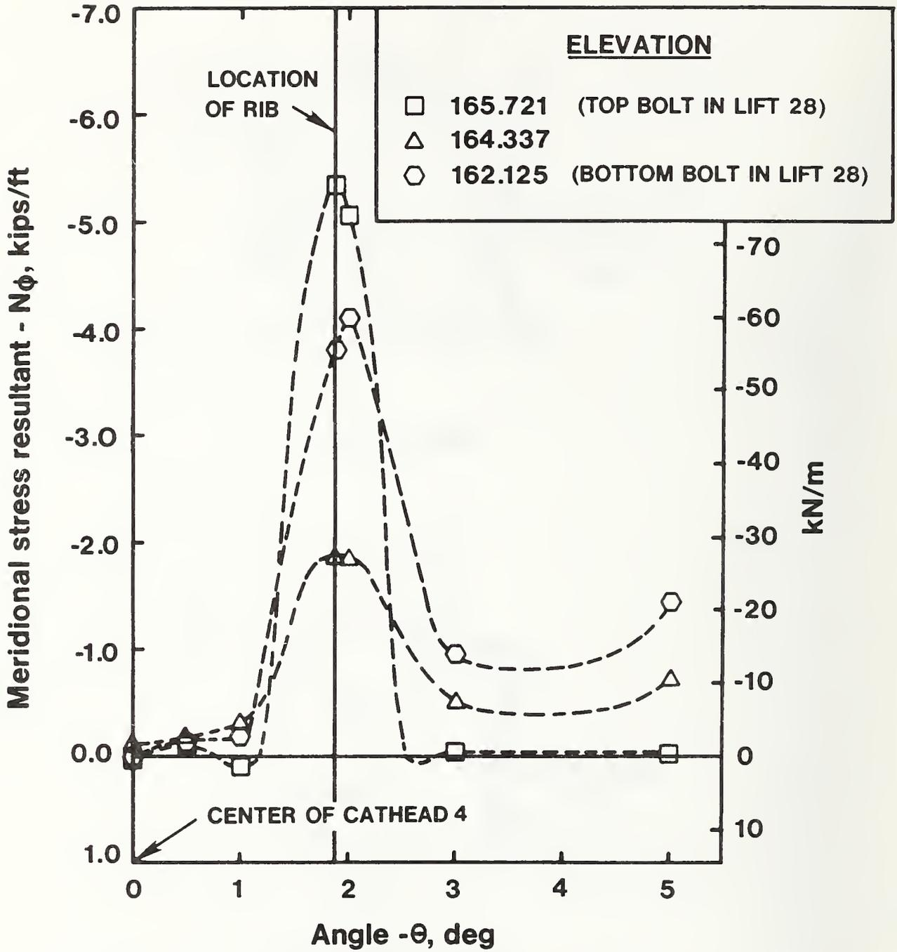
Figure 6.20 Meridional stress resultant at cathead no. 4
