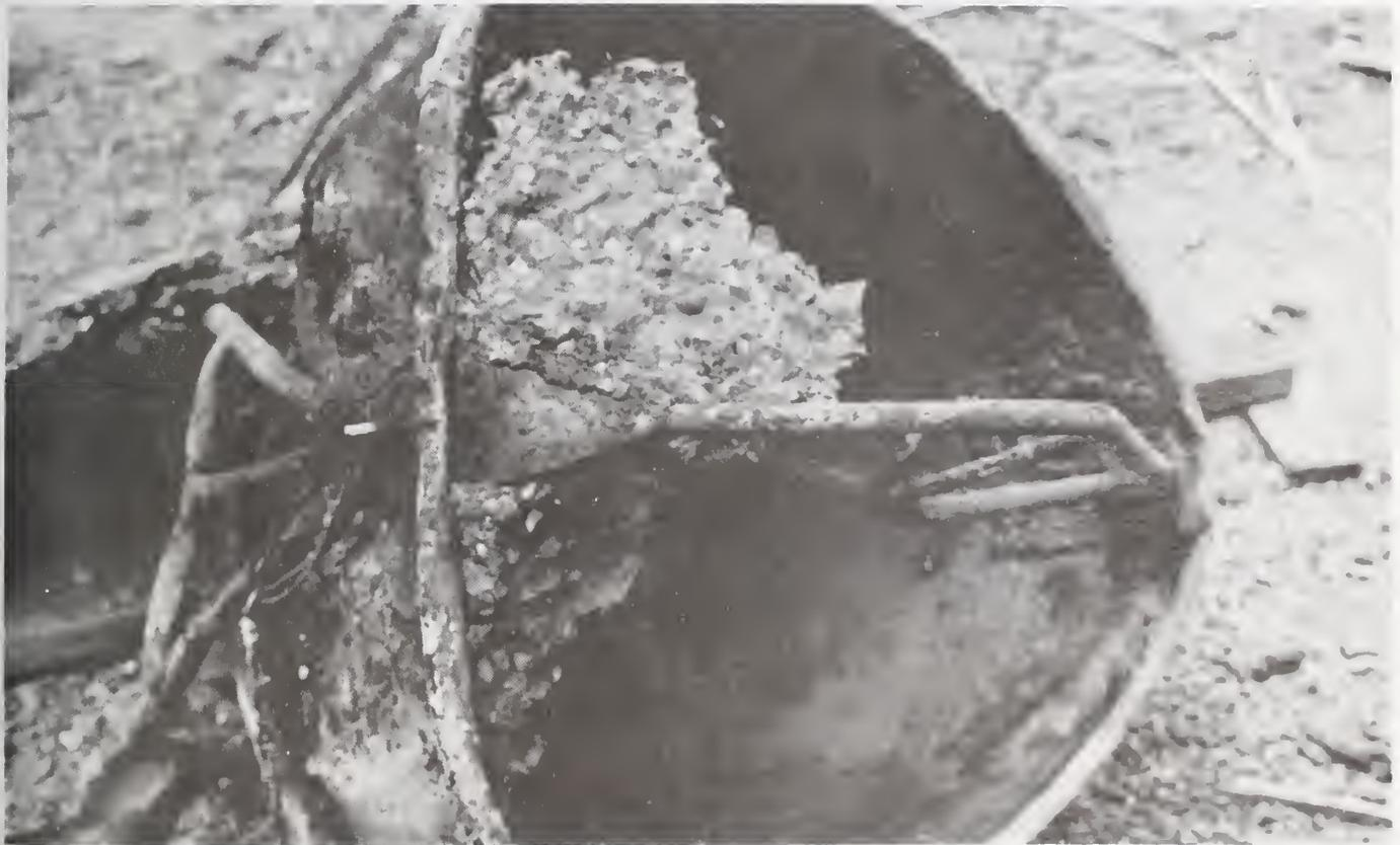
Figure 3.18 Concrete Basket Used for Cathead Gantry No. 4 Which Was Recovered from Wreckage
