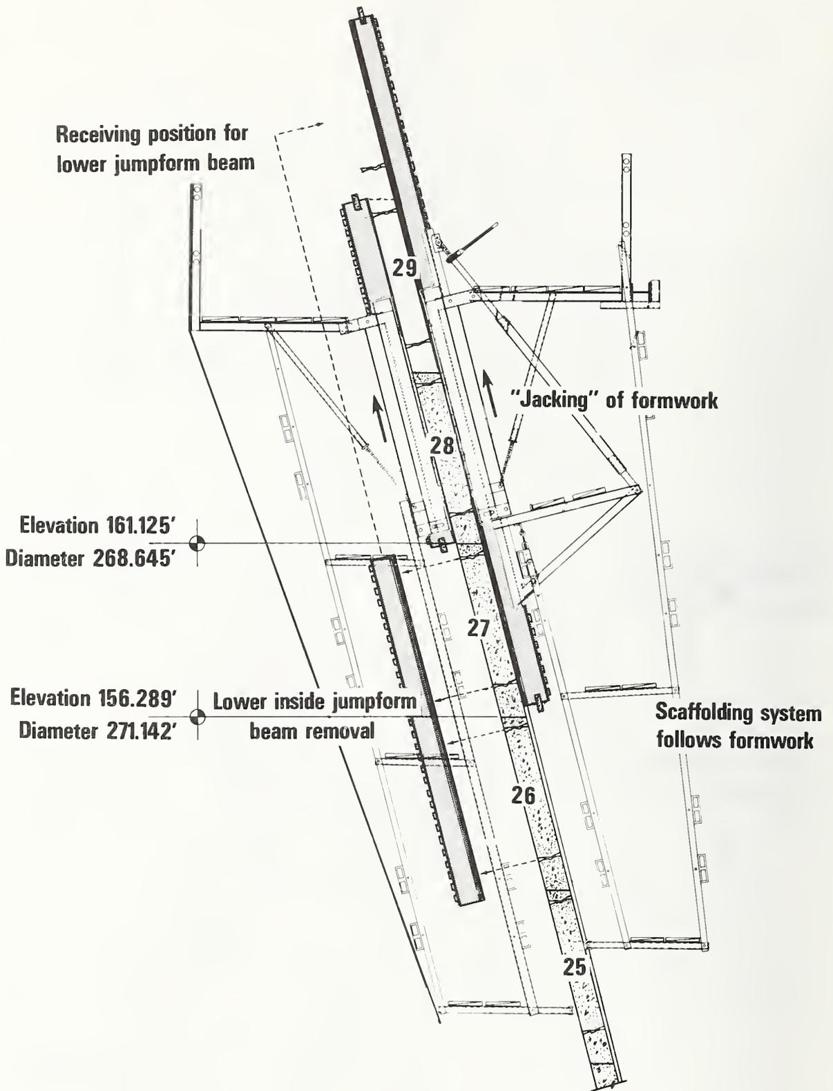
Figure 2.14 Raising of Formwork and Relocation of Jumpform Beam after Casting of Lift 28
