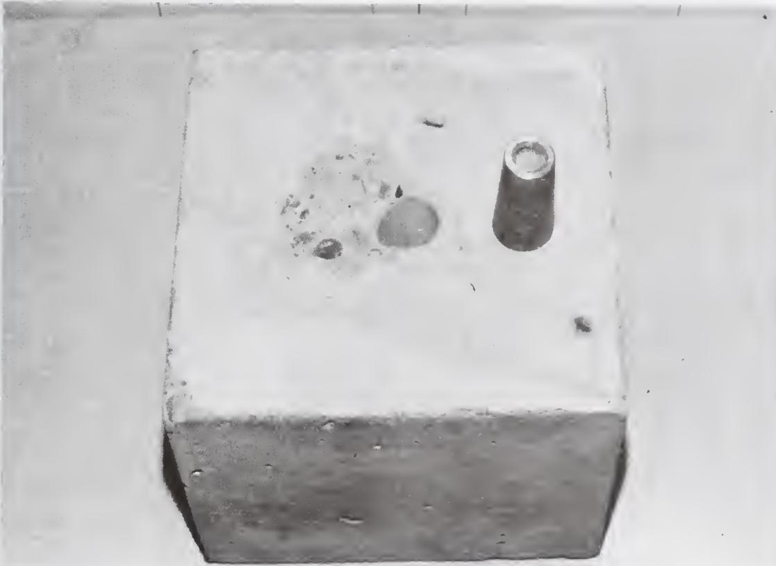
Figure 4.10 Fractured Williams Anchor Bolt Embedded in a Concrete Block
