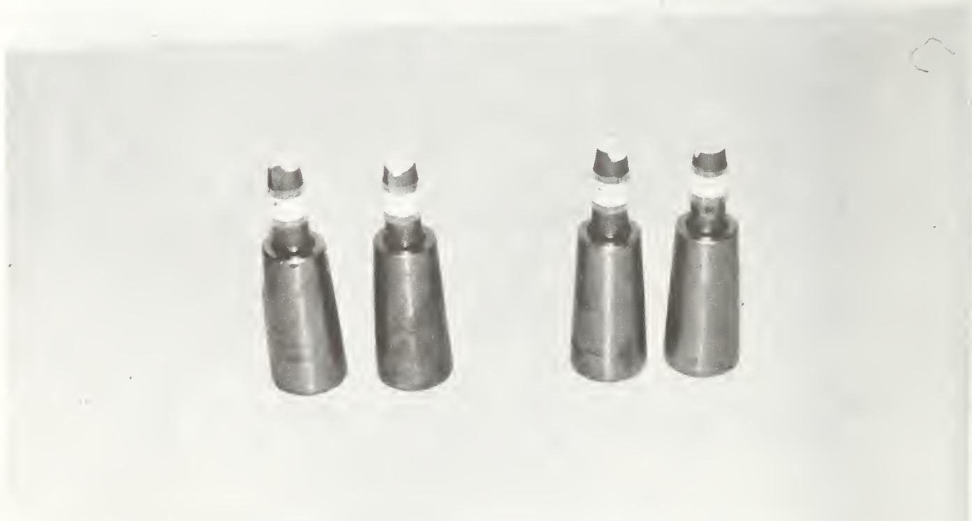
Figure 4.9 Appearance of Williams Anchor Bolts After Tension Test
