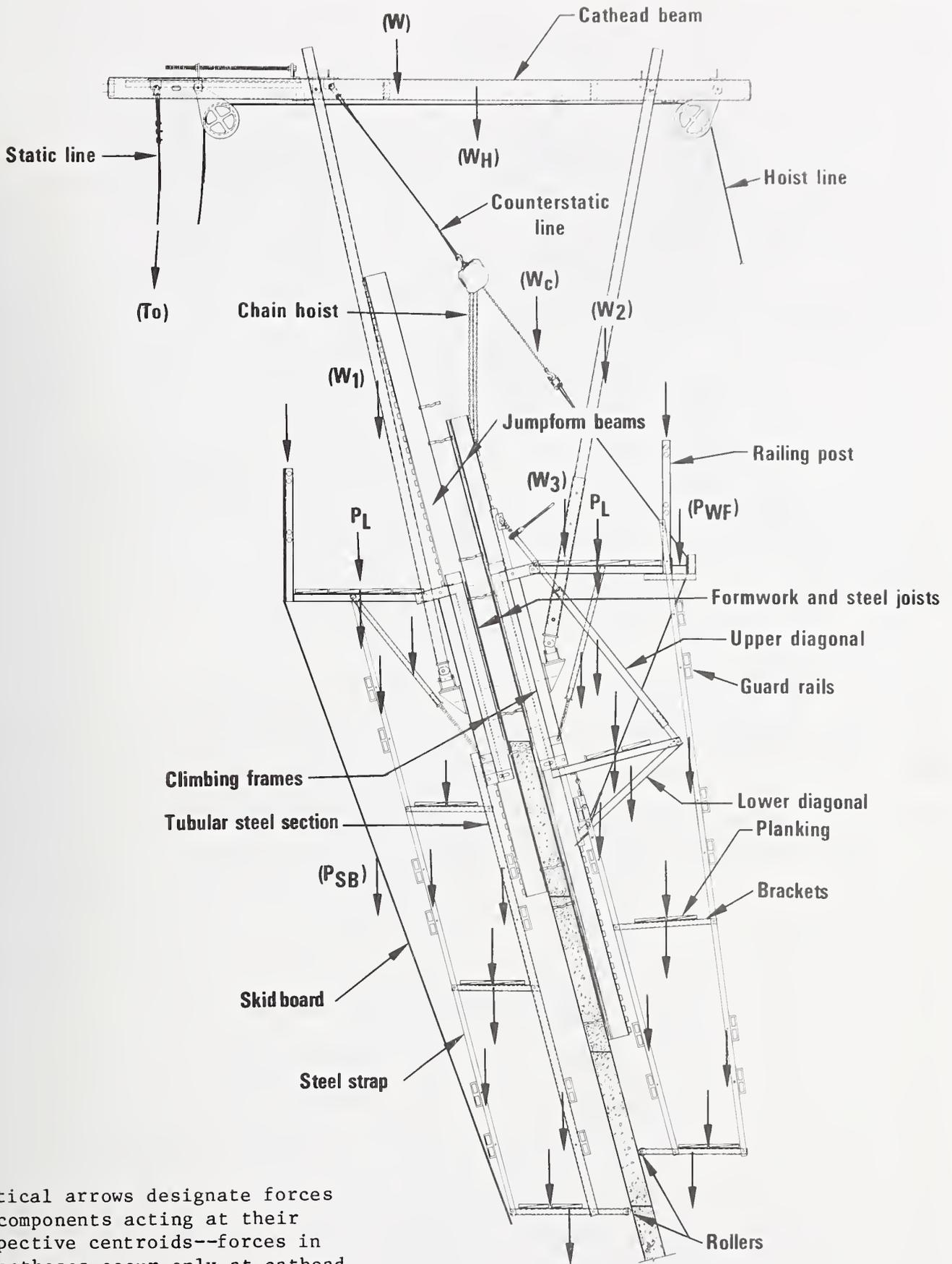
(Vertical arrows designate forces of components acting at their respective centroids--forces in parentheses occur only at cathead locations)
