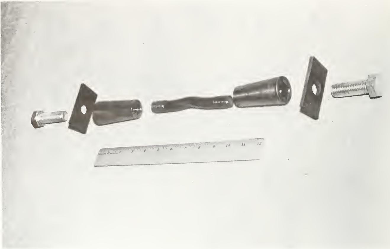
Figure 4.8 Williams Anchor Bolt Assembly
