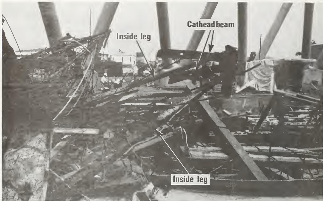
Figure 3.15 Inside Legs of Cathead Gantry No. 4
