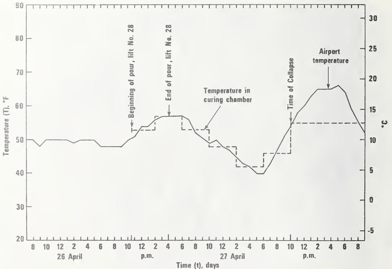
Figure 4.1 Temperature Variation Used to Cure Test Specimens
