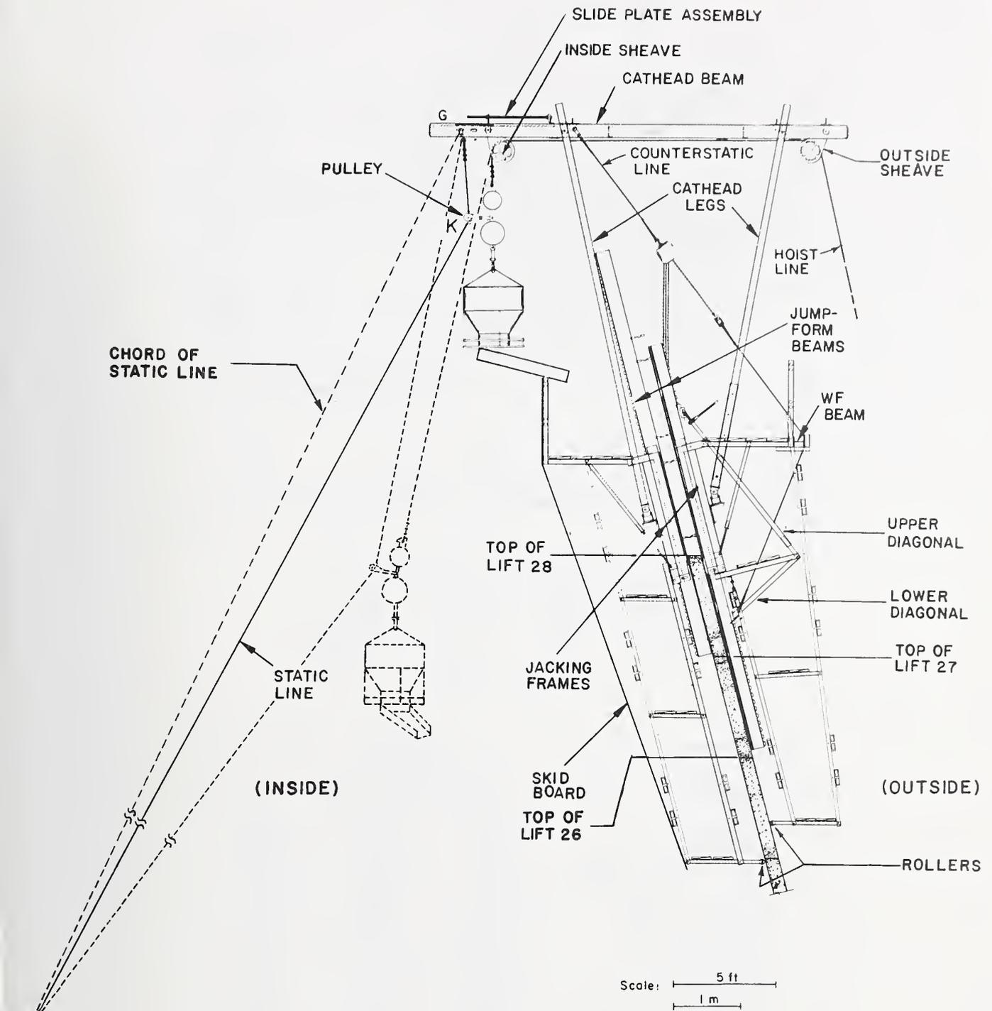
Figure 6.1 General Sectional Configuration of Construction Scheme
