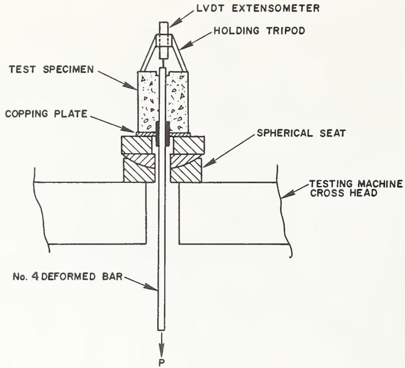
Figure 4.5 Pull-out Test Setup
