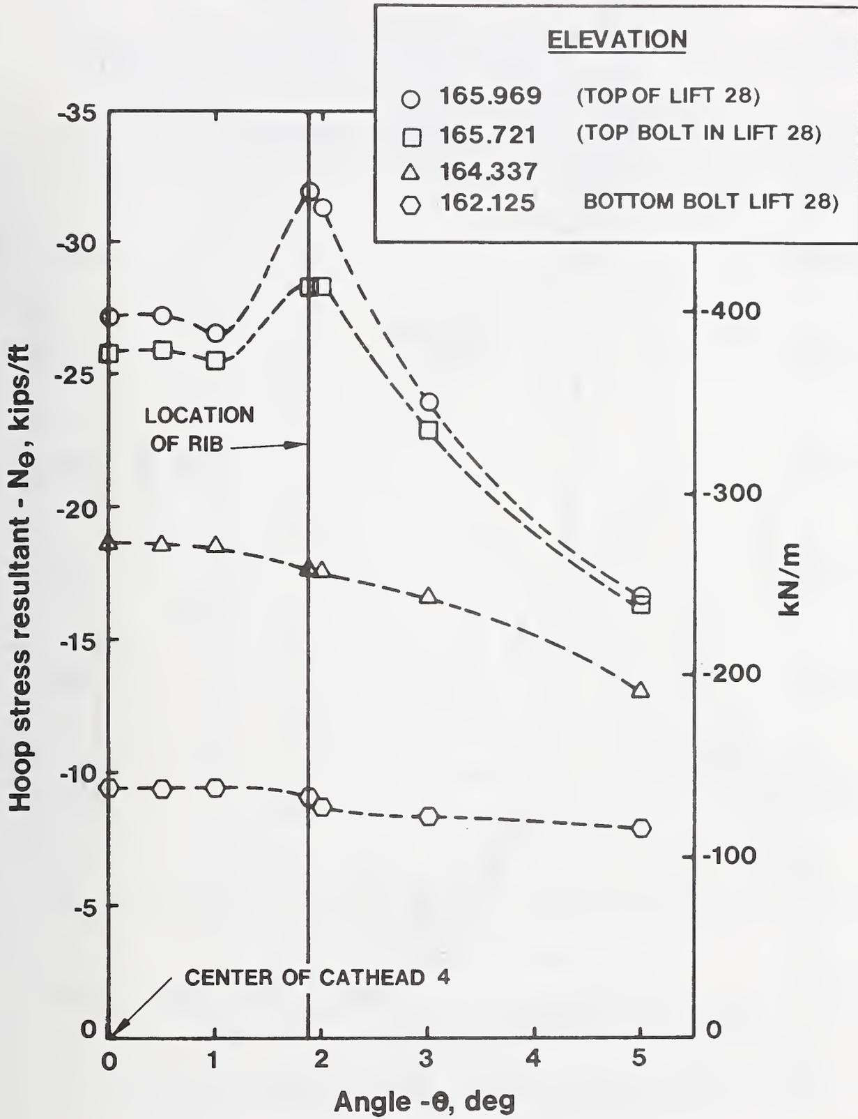
Figure 6.21 Hoop stress resultant at cathead no. 4
