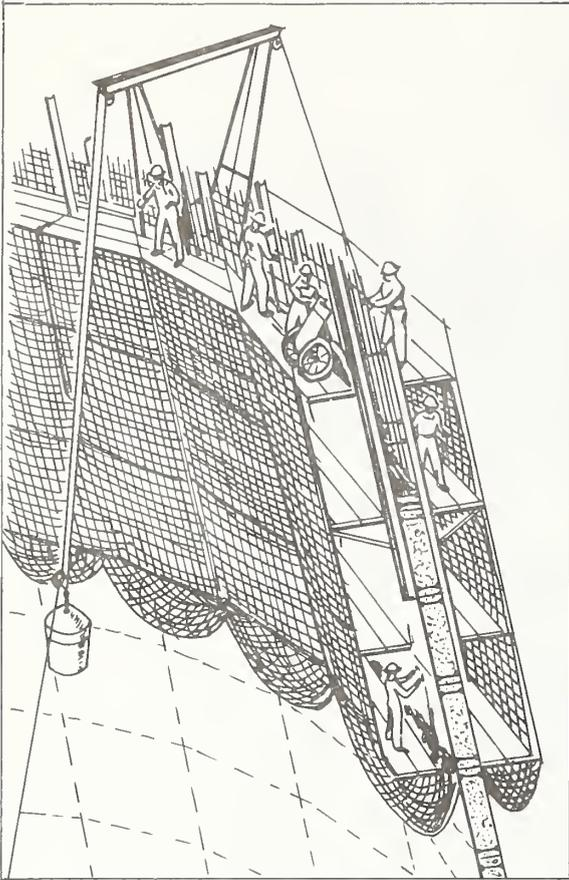
Figure 2.3 Perspective View of the Scaffolding System
