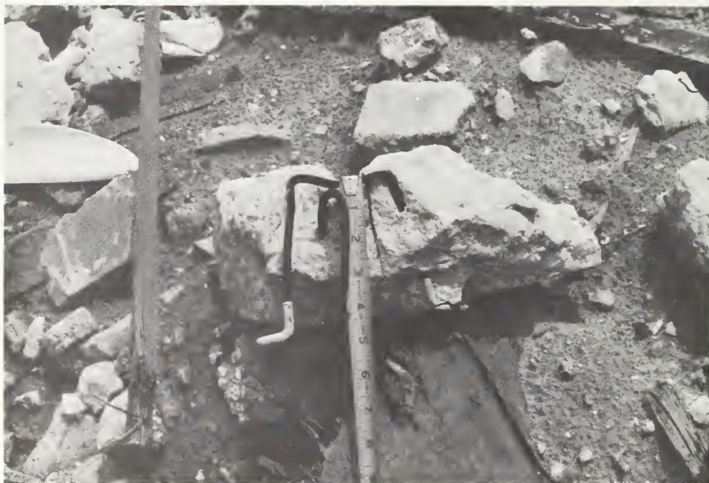
Figure 2.5 Field measurement of chair heights for top bars in column strip
