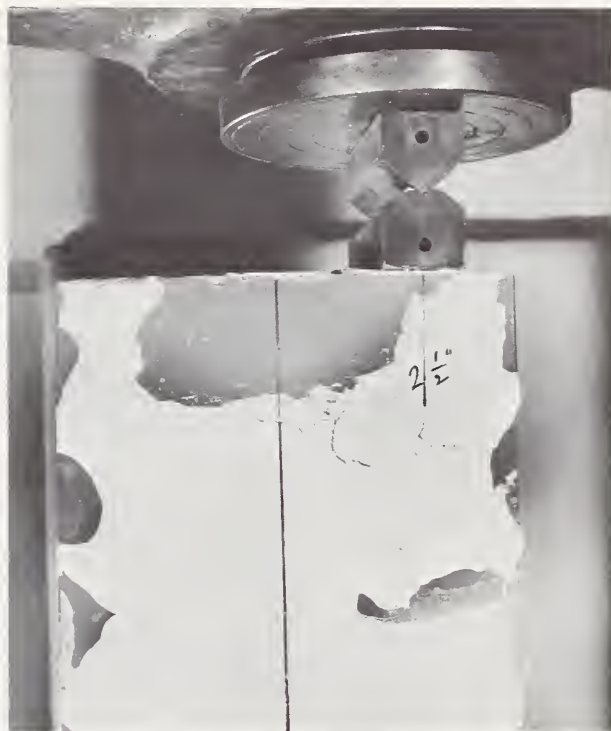
FIGURE 7. Closeup of eccentrically loaded wall showing the loading knife edge.
