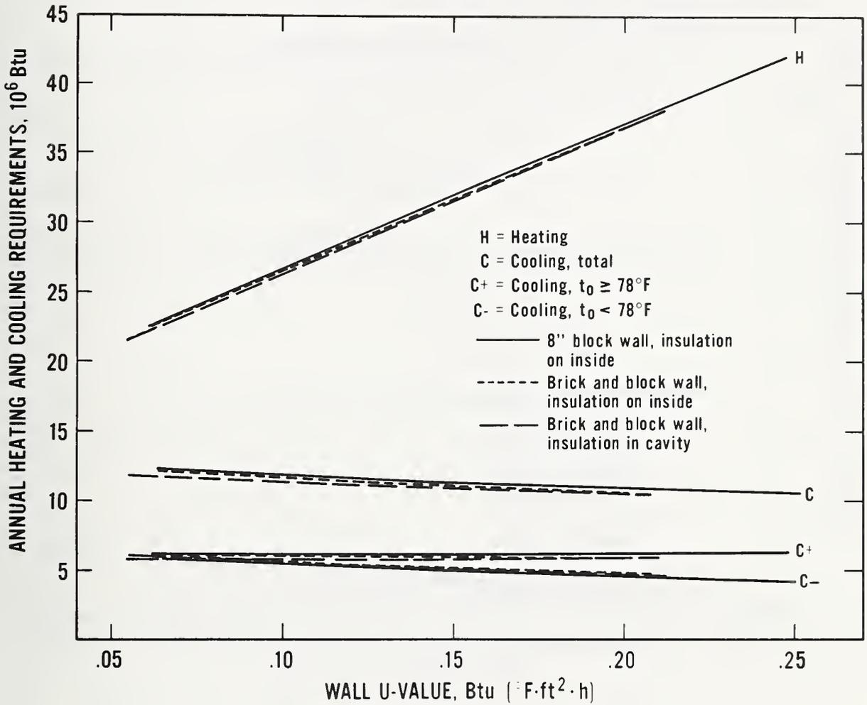
Figure B.14 Indianapolis, Indiana: Relationship Between Annual Heating and Cooling Requirements and Wall U-value for an 1176  $\text{ft}^2$  House (8-in Block Walls and Brick and Block Walls)
