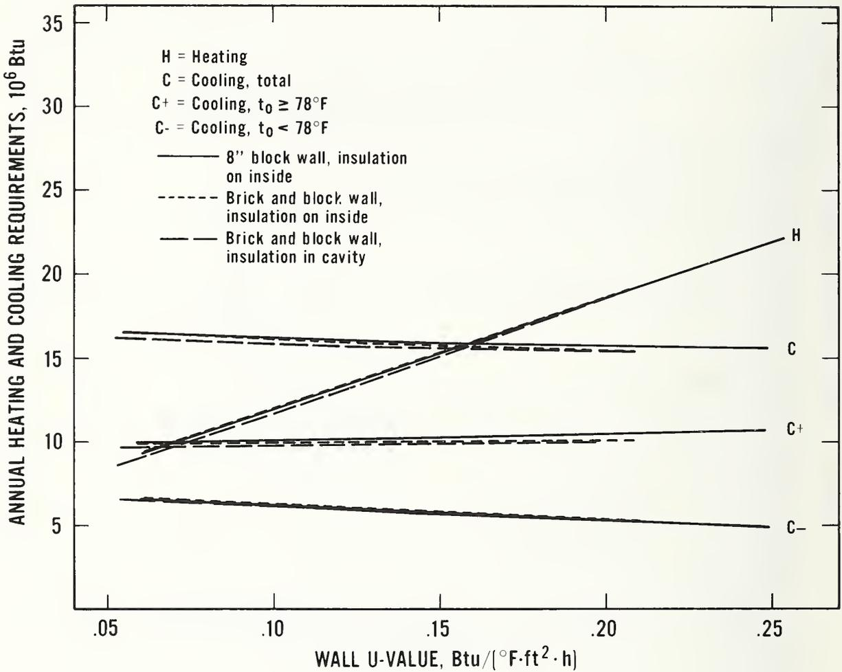
Figure B.19 Washington, D.C.: Relationship Between Annual Heating and Cooling Requirements and Wall U-value for an 1176 ft<sup>2</sup> House (8-in Block Walls and Brick and Block Walls)
