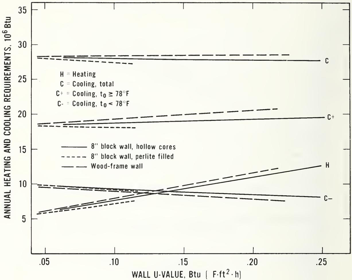
Figure B.5 Jackson, Mississippi: Relationship Between Annual Heating and Cooling Requirements and Wall U-value for an 1176 ft<sup>2</sup> House (8-in Block Walls and Wood-Frame Walls)
