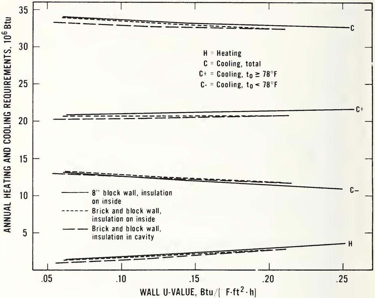
Figure B.15 Jacksonville, Florida: Relationship Between Annual Heating and Cooling Requirements and Wall U-value for an 1176 ft<sup>2</sup> House (8-in Block Walls and Brick and Block Walls)
