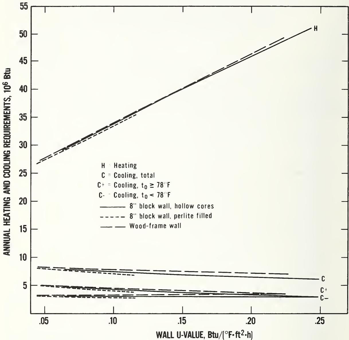
Figure B.1 Albany, New York: Relationship Between Annual Heating and Cooling Requirements and Wall U-value for an 1176  $\text{ft}^2$  House (8-in Block Walls and Wood-Frame Walls)
