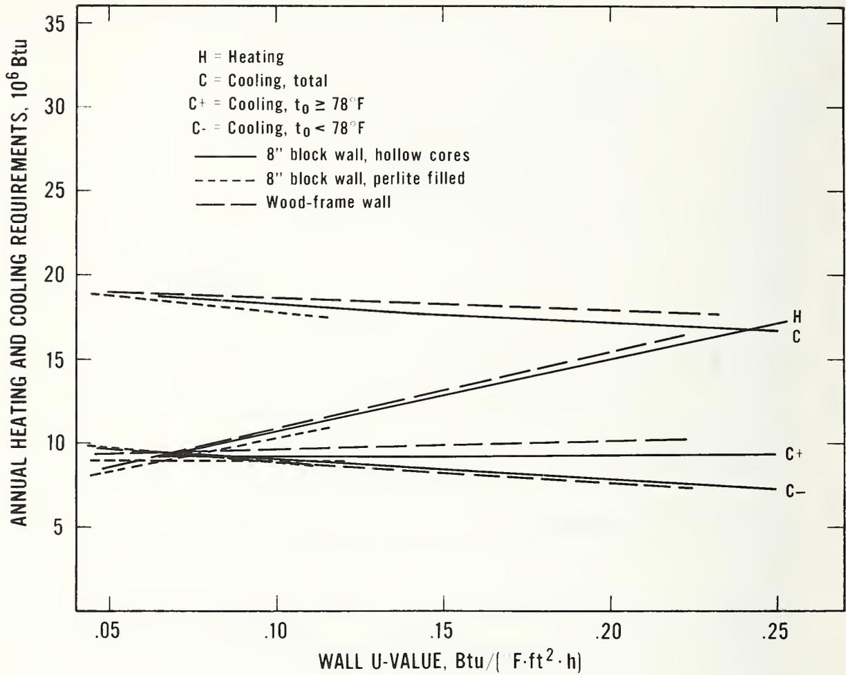
Figure B.3 Atlanta, Georgia: Relationship Between Annual Heating and Cooling Requirements and Wall U-value for an 1176 ft<sup>2</sup> House (8-in Block Walls and Wood-Frame Walls)
