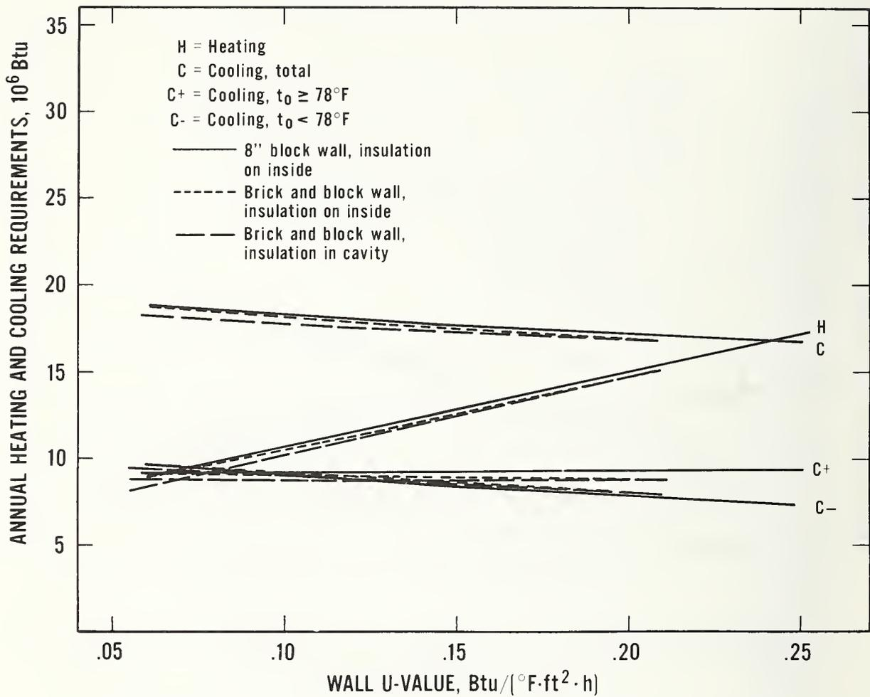
Figure B.13 Atlanta, Georgia: Relationship Between Annual Heating and Cooling Requirements and Wall U-value for an 1176 ft<sup>2</sup> House (8-in Block Walls and Brick and Block Walls)
