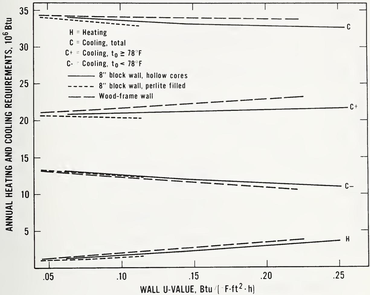
Figure B.6 Jacksonville, Florida: Relationship Between Annual Heating and Cooling Requirements and Wall U-value for an 1176  $\text{ft}^2$  House (8-in Block Walls and Wood-Frame Walls)
