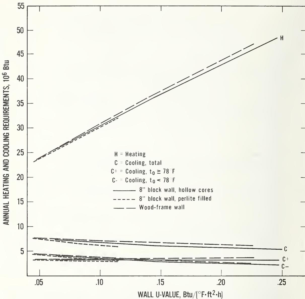
Figure B.7 Madison, Wisconsin: Relationship Between Annual Heating and Cooling Requirements and Wall U-value for an 1176 ft<sup>2</sup> House (8-in Block Walls and Wood-Frame Walls)
