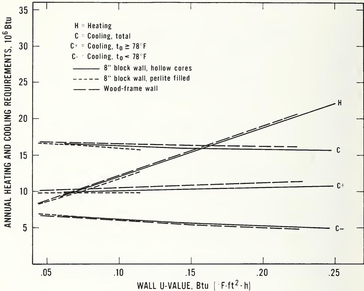
Figure B.11 Washington, D.C.: Relationship Between Annual Heating and Cooling Requirements and Wall U-value for an 1176 ft<sup>2</sup> House (8-in Block Walls and Wood-Frame Walls)
