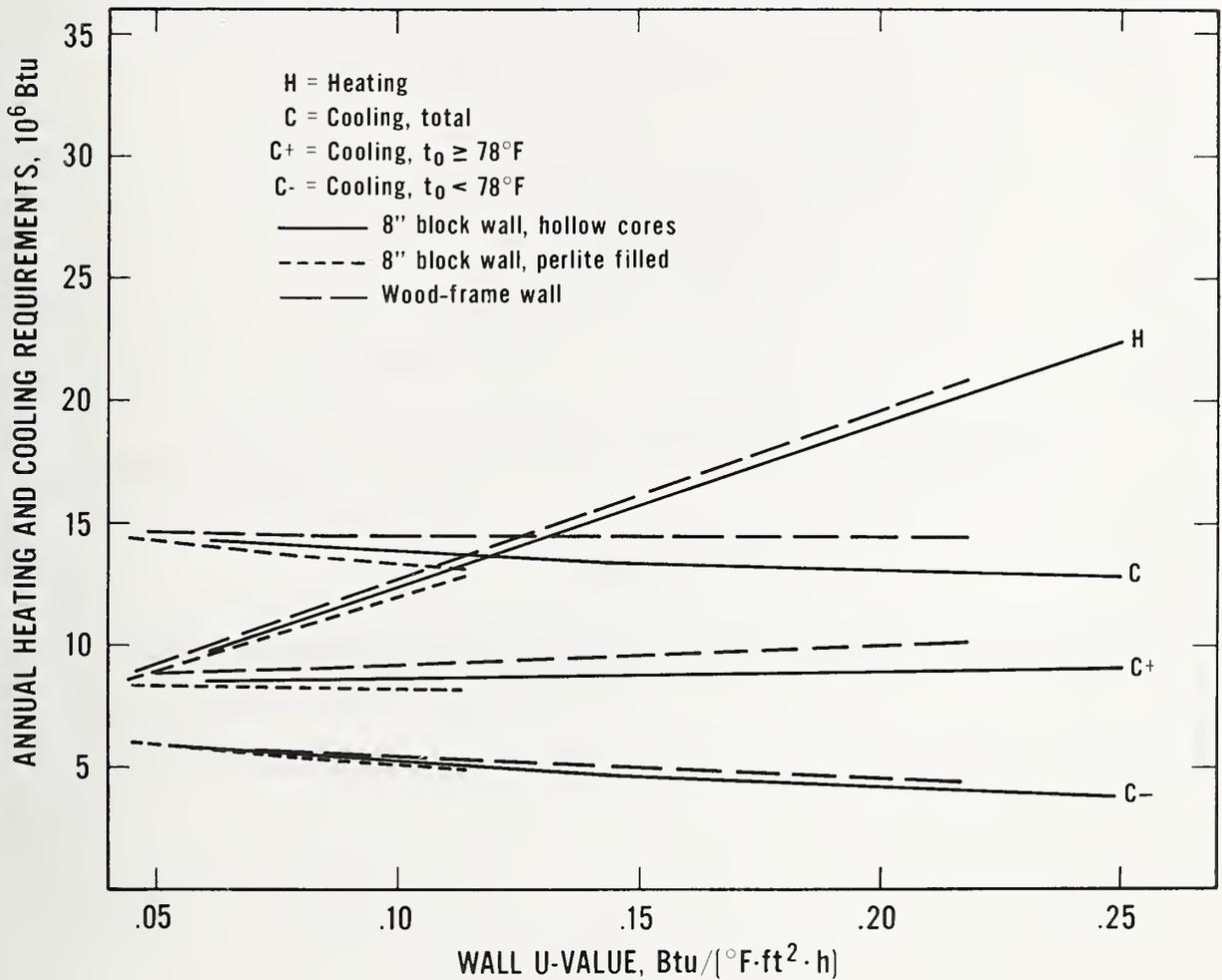
Figure B.2 Albuquerque, New Mexico: Relationship Between Annual Heating and Cooling Requirements and Wall U-value for an 1176  $\text{ft}^2$  House (8-in Block Walls and Wood-Frame Walls)
