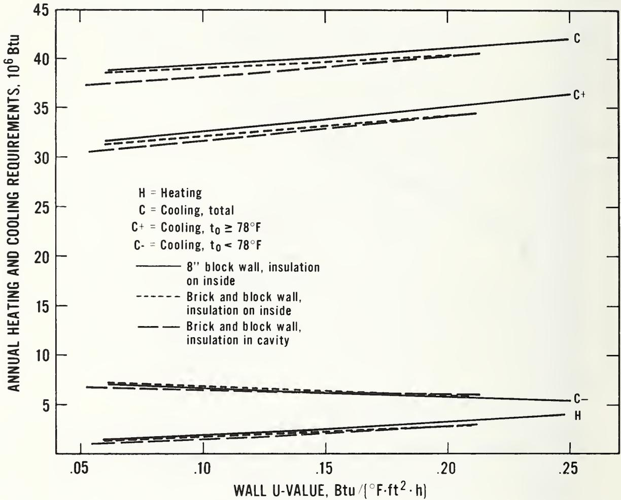
Figure B.17 Phoenix, Arizona: Relationship Between Annual Heating and Cooling Requirements and Wall U-value for an 1176 ft<sup>2</sup> House (8-in Block Walls and Brick and Block Walls)
