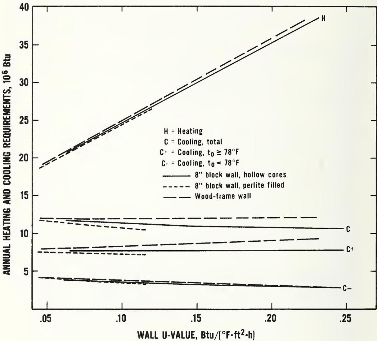
Figure B.9 Salt Lake City, Utah: Relationship Between Annual Heating and Cooling Requirements and Wall U-value for an 1176 ft<sup>2</sup> House (8-in Block Walls and Wood-Frame Walls)
