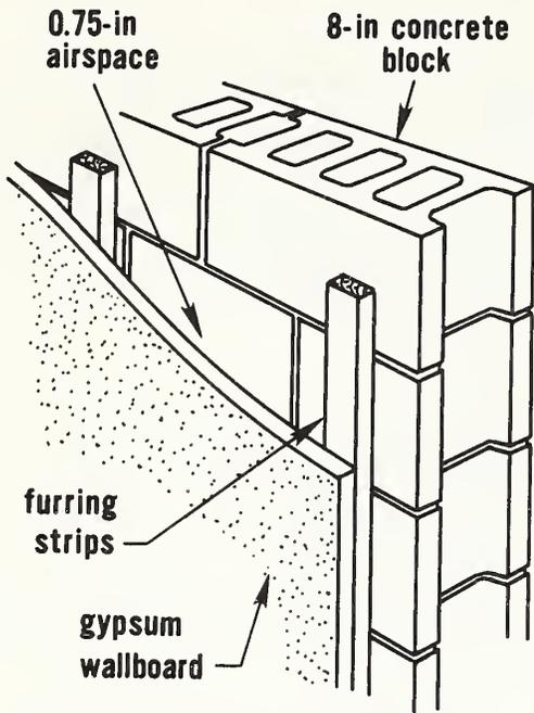
(a) 8-in concrete block wall
