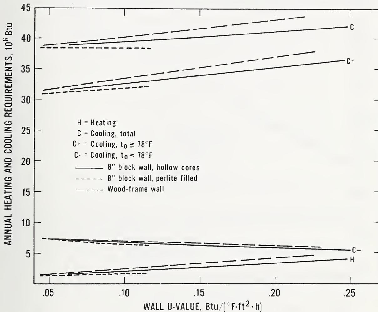
Figure B.8 Phoenix, Arizona: Relationship Between Annual Heating and Cooling Requirements and Wall U-value for an 1176 ft<sup>2</sup> House (8-in Block Walls and Wood-Frame Walls)
