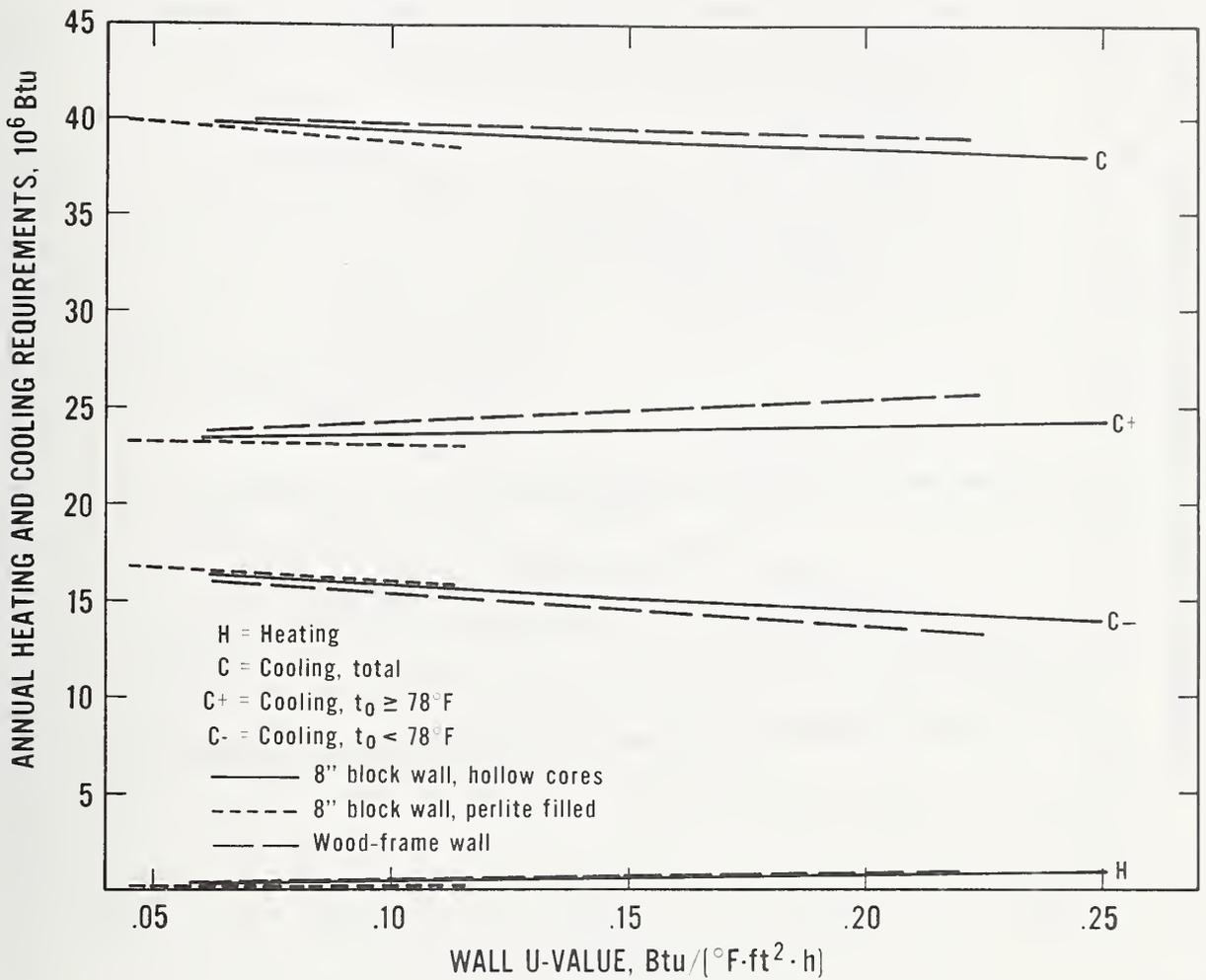
Figure B.10 Tampa, Florida: Relationship Between Annual Heating and Cooling Requirements and Wall U-value for an 1176 ft<sup>2</sup> House (8-in Block Walls and Wood-Frame Walls)
