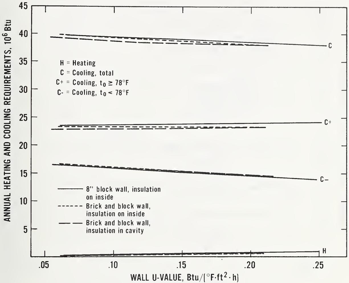
Figure B.18 Tampa, Florida: Relationship Between Annual Heating and Cooling Requirements and Wall U-value for an 1176 ft<sup>2</sup> House (8-in Block Walls and Brick and Block Walls)
