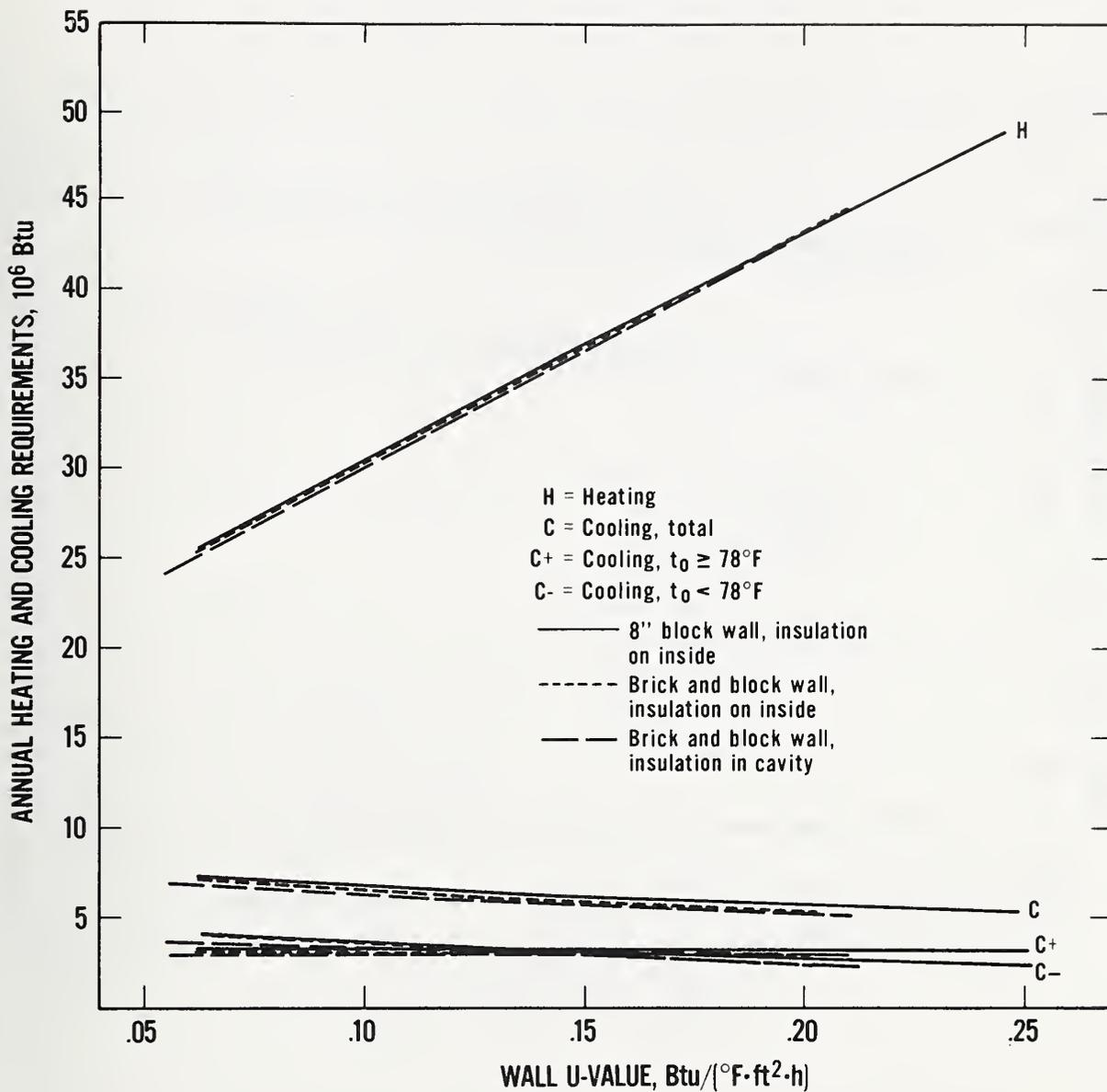
Figure B.16 Madison, Wisconsin: Relationship Between Annual Heating and Cooling Requirements and Wall U-value for an 1176 ft<sup>2</sup> House (8-in Block Walls and Brick and Block Walls)
