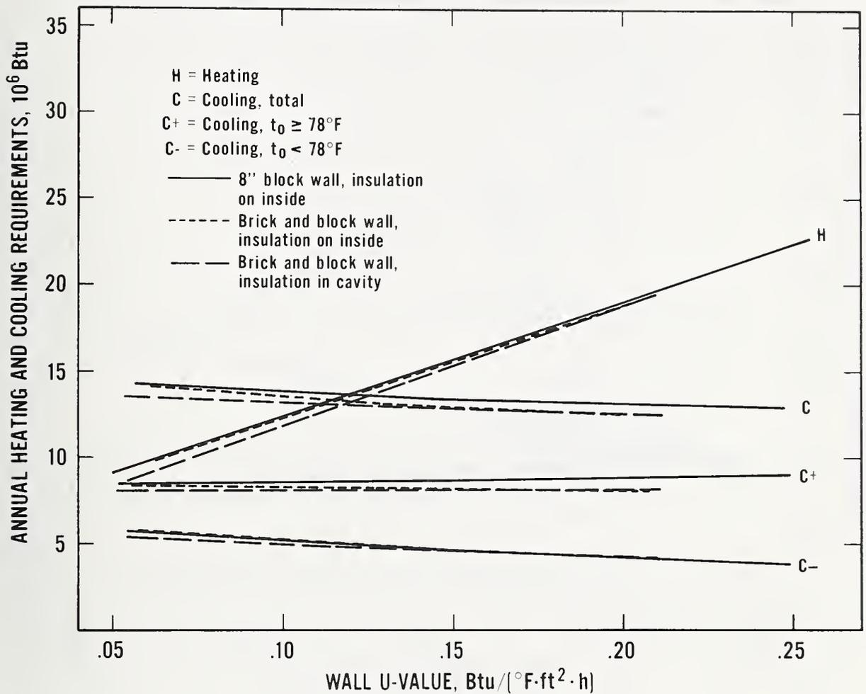
Figure B.12 Albuquerque, New Mexico: Relationship Between Annual Heating and Cooling Requirements and Wall U-value for an 1176  $\text{ft}^2$  House (8-in Block Walls and Brick and Block Walls)
