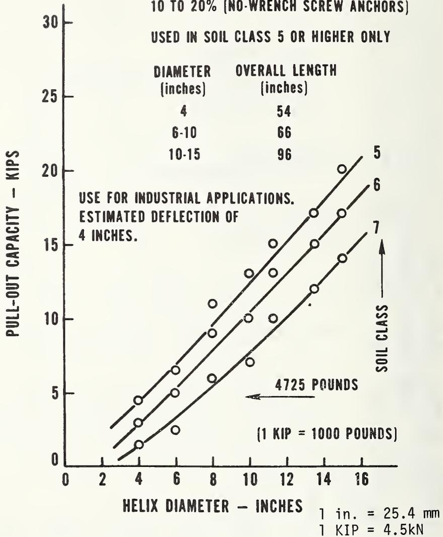
Figure 6.5 Pull-out Capacity versus Helix Diameter [25]
