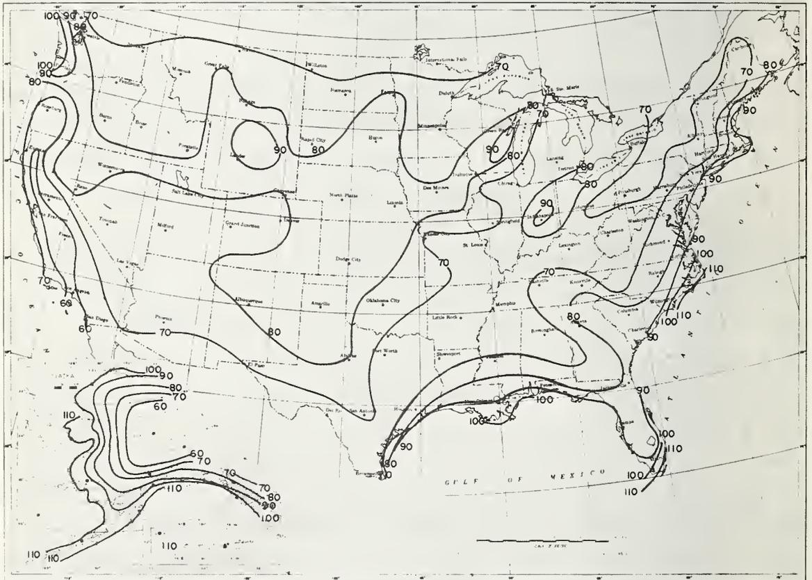
Figure 6.7 Basic Wind Speed in Miles Per Hour (mph). Annual Extreme Fastest Mile Speed 30 ft above ground, 50-year Mean Recurrence Interval [10]
