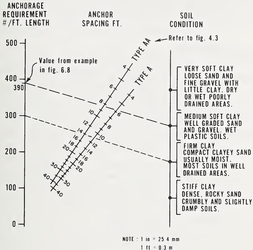
Figure 6.10 Anchor Spacing Chart, Type A and AA Anchors (6-inch Helix and 10-inch Arrowhead Shaped Anchors, Respectively) [46]
