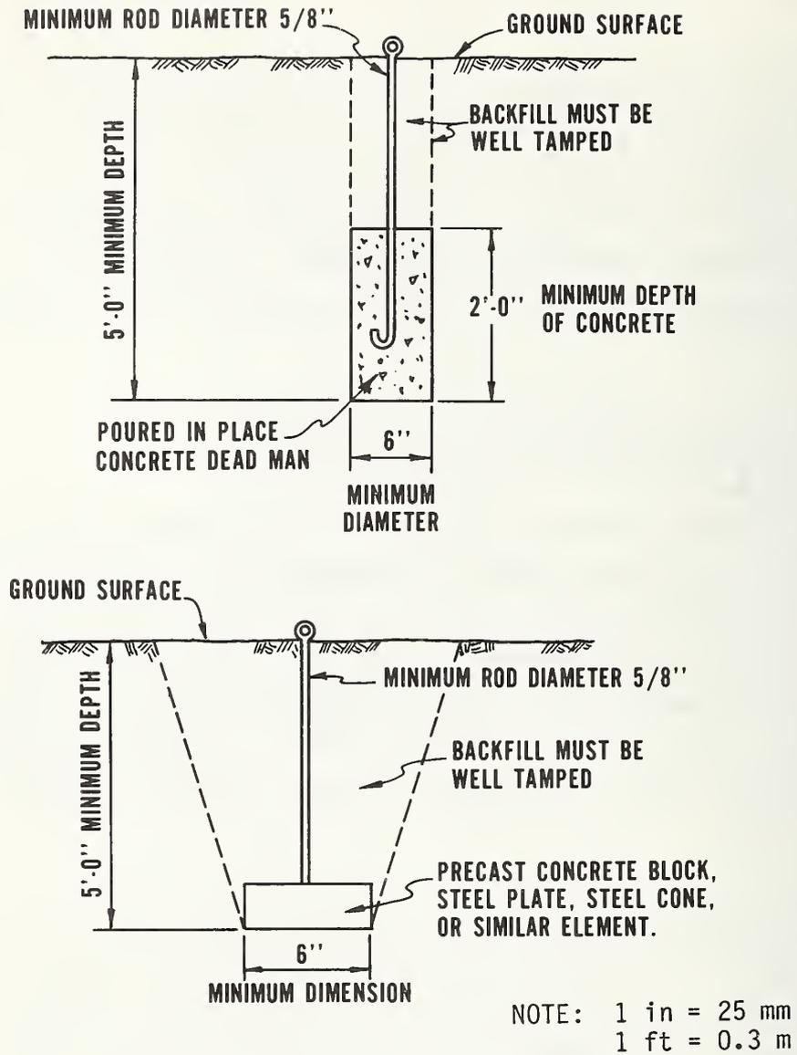
Figure 4.7 Examples of Dead-man Anchor Installation and their Minimum Requirements [46]
