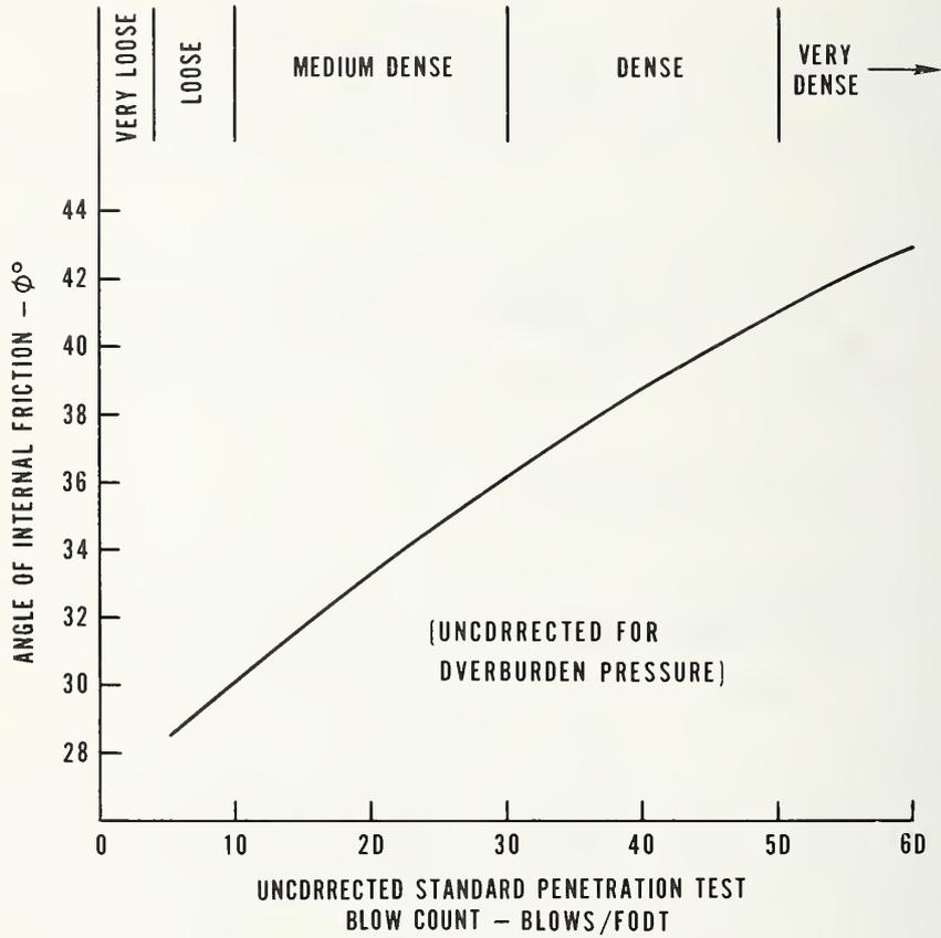
Figure 5.4 Angle of Internal Friction (Shearing Resistance) versus (Uncorrected) SPT Blow Count for Sands [83]
