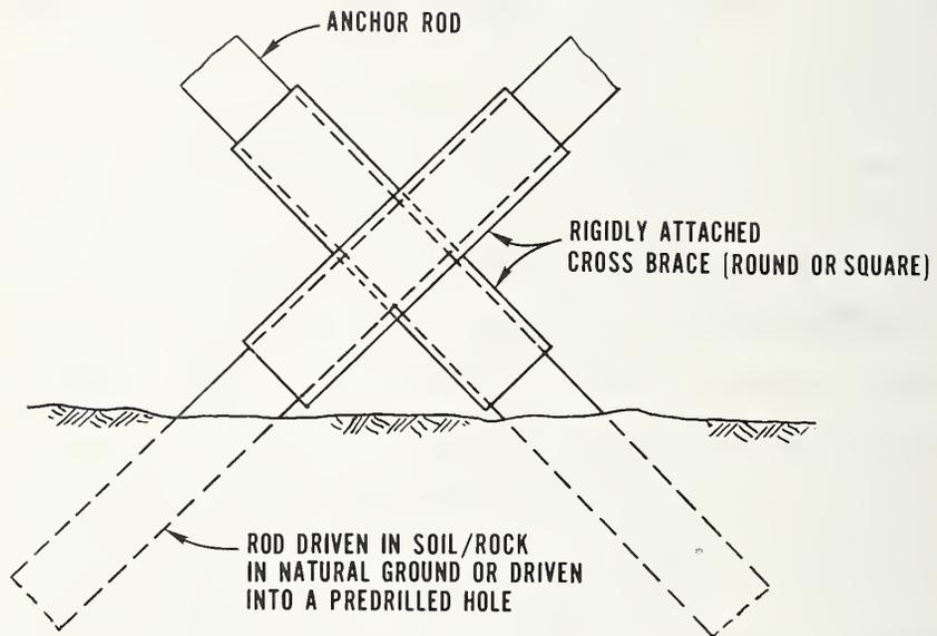
Figure 4.6 "X Type Rock" Anchor
