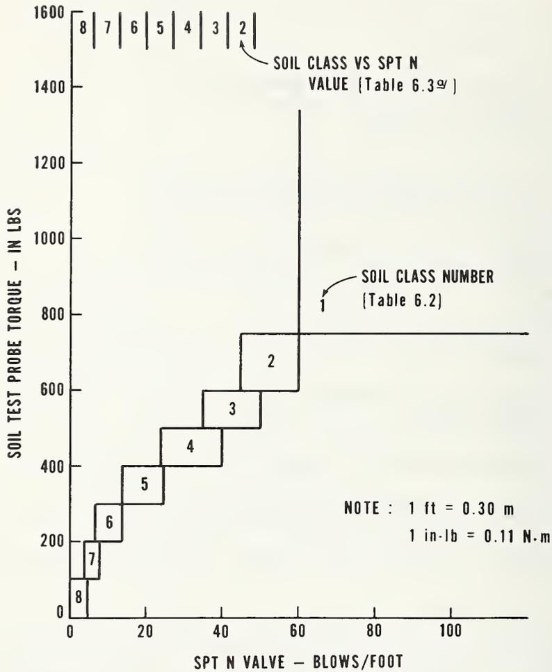
Figure 6.2 Soil Test Probe Torque versus SPT N Value [26, 58]
