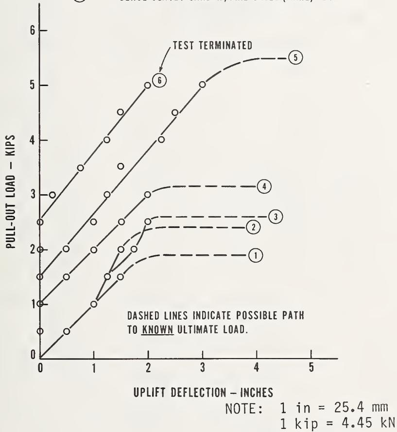
Figure 7.10 Pull-out Load versus Uplift Deflection for Expanding Plate Anchor [99]
