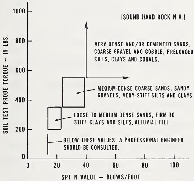
Figure 6.1 Soil Test Probe Torque versus SPT N Value [69]
