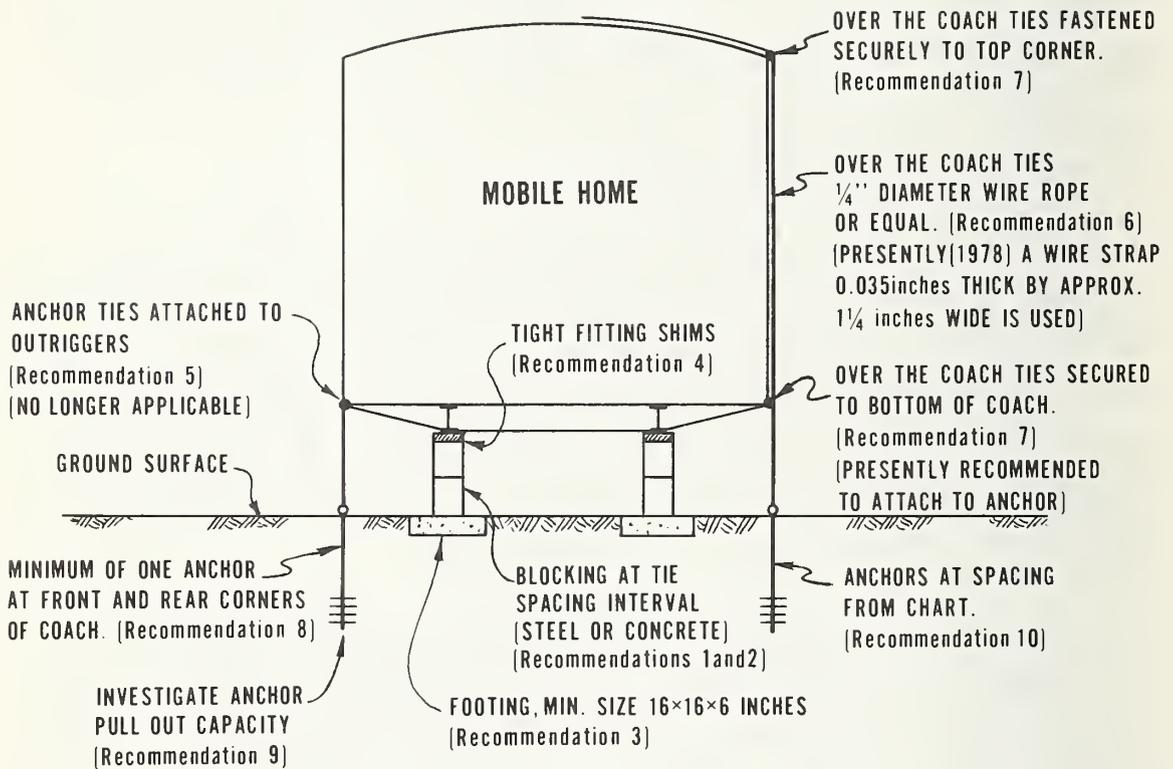
Figure 2.1 Summary of Recommendations for Installation of Anchors by Harris [46]
