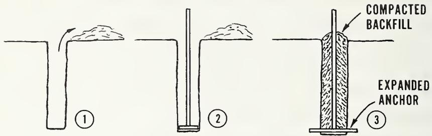
a. PROCEDURE ① EXCAVATE HOLE. ② INSTALL ANCHOR. ③ EXPAND ANCHOR AND BACKFILL.
