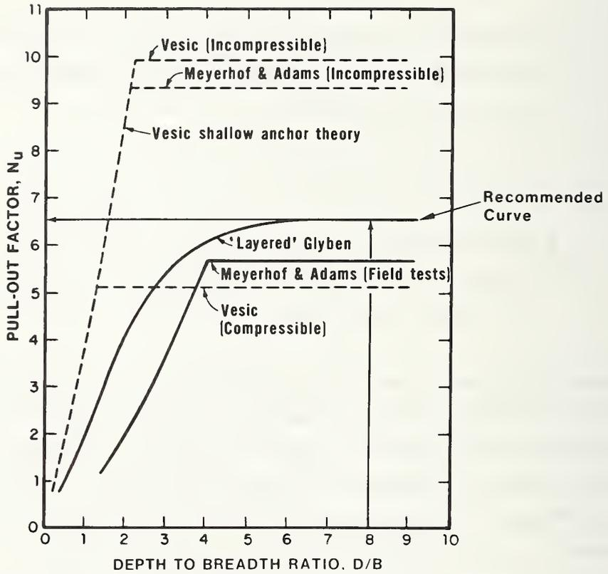
Figure 5.1 Pull-out factor  $N_u$ , versus  $D/B$  Ratio for Cohesive Soils [33]
