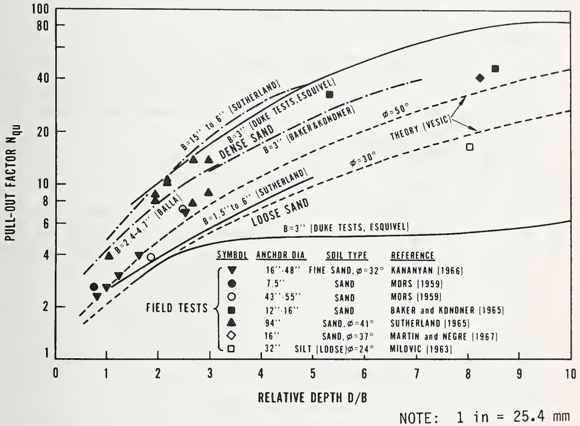
Figure 5.5 Pull-out Factor,  $N_{qu}$ , versus  $D/B$  Ratio for Sands [103]
