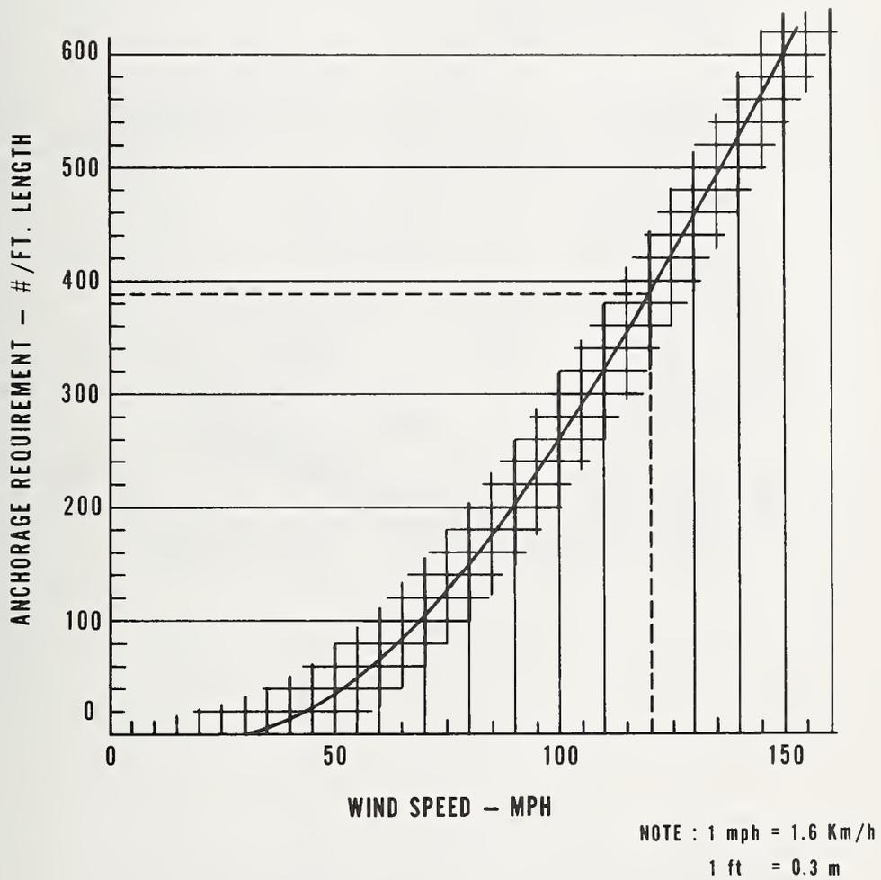
Figure 6.8 Recommended Wind Velocity - Anchorage Requirement Curve by Harris [46]
