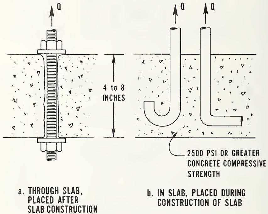
Figure 4.9 Concrete Slab Anchors
