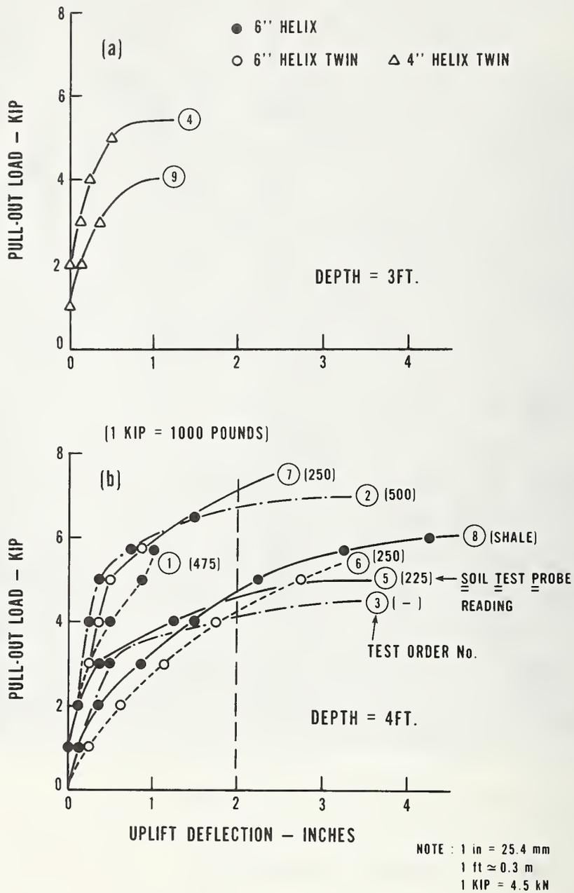
Figure 7.1 Pull-out Load versus Uplift Deflection for Helix Anchors. (A) 4-inch Anchors at 3-foot depth; and (B) 6-inch Anchors at 4-foot depth
