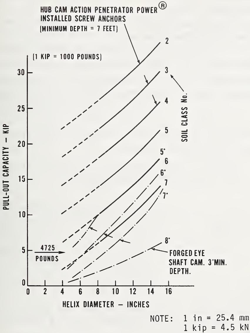
Figure 6.6 Pull-out Capacity versus Helix Diameter [58]
