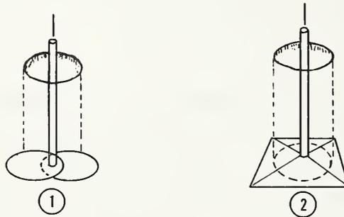
b. TWO AVAILABLE TYPES. ① ECCENTRIC PLATES. ② EXPANDING SCREW DOWN PLATES.
