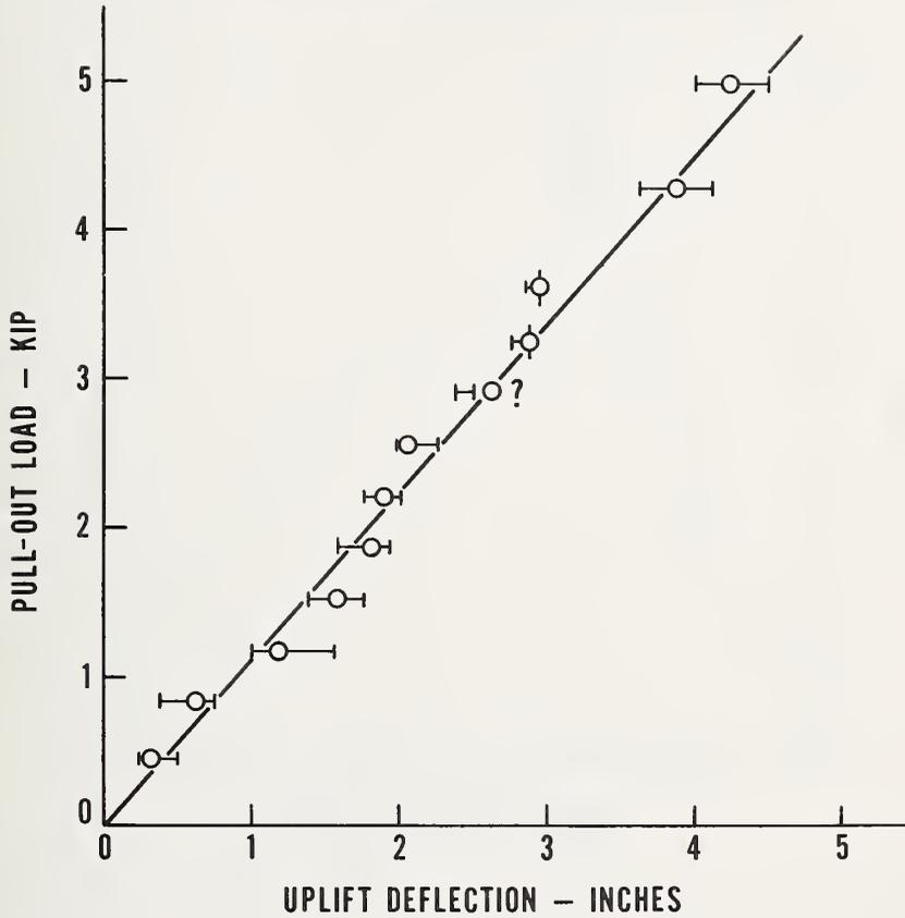
Figure 7.7 Pull-out Load versus Uplift Deflection for a 6-inch Arrowhead Anchor
