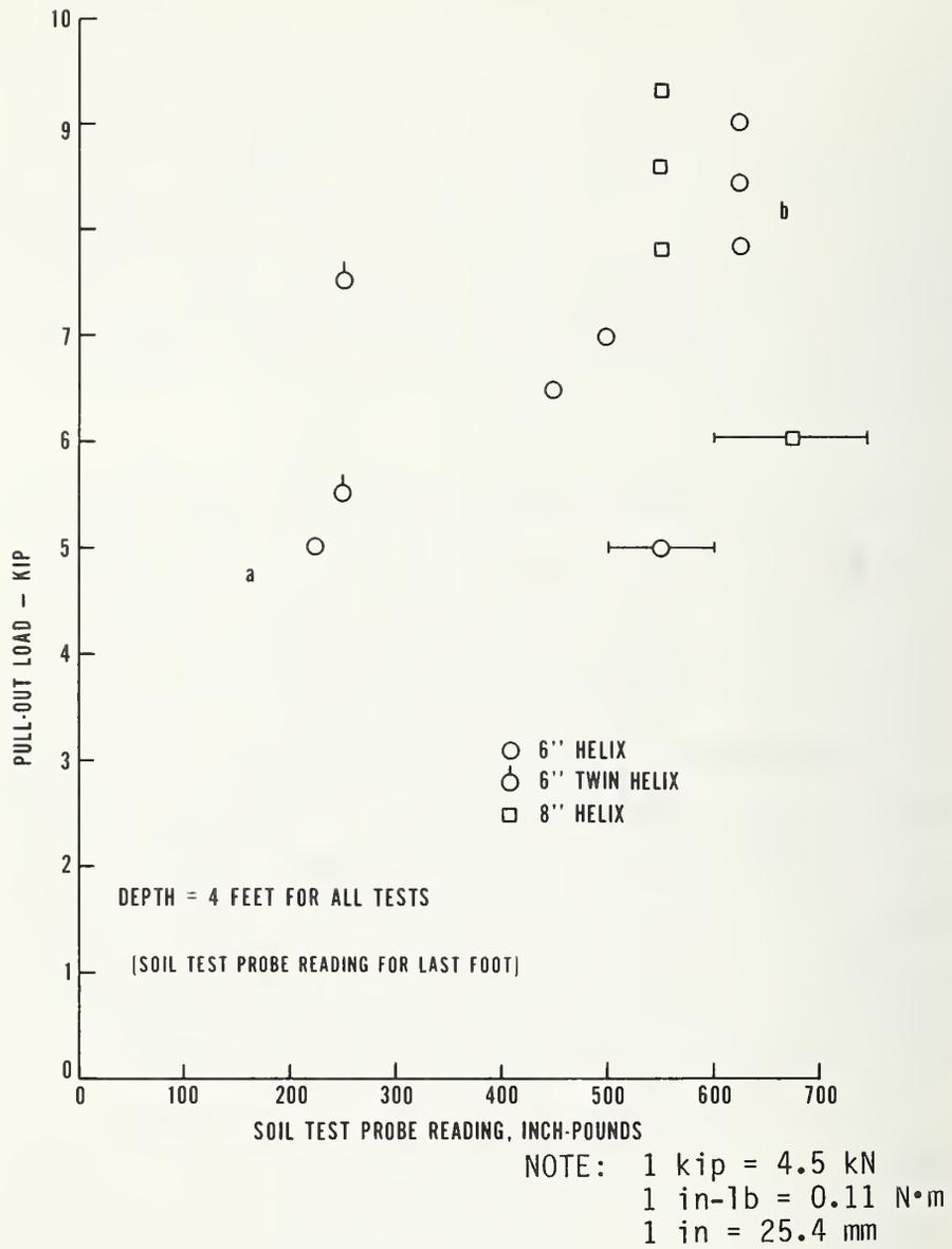
Figure 7.2 Pull-out Load versus STP for Various Anchor Types
