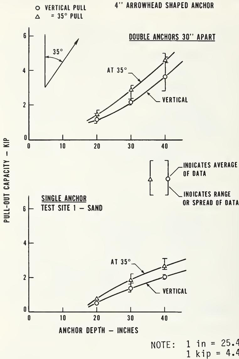
Figure 7.4 Summary of Pull-out Test Data for 4-inch Arrowhead Shaped Anchors, Sand Site [85]
