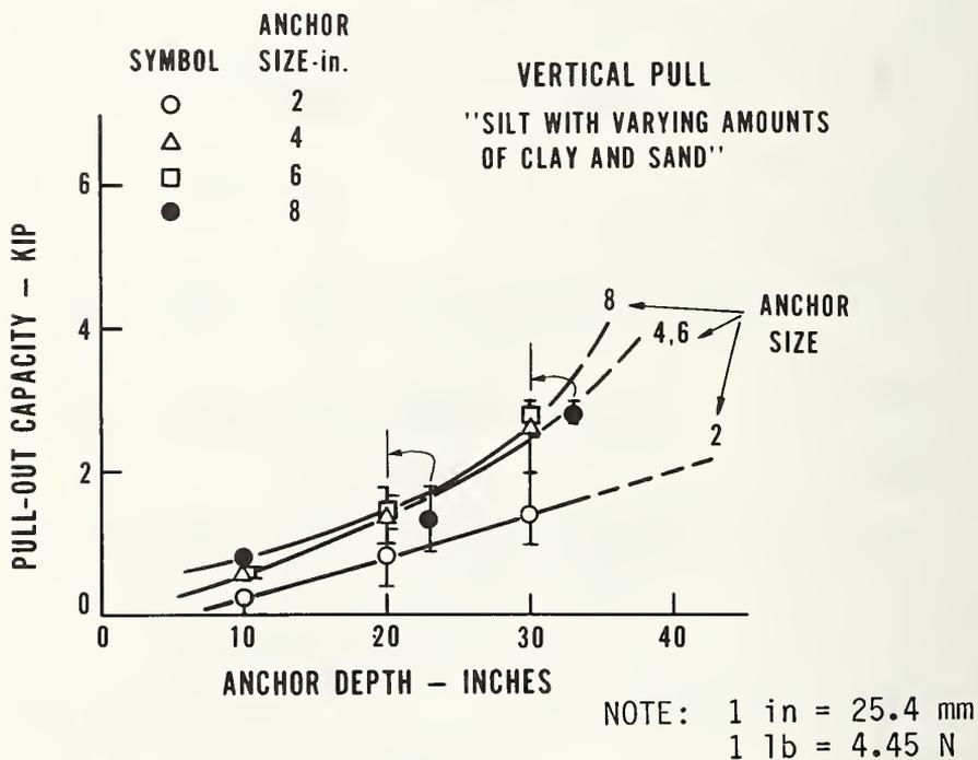
Figure 7.6 Pull-out Capacity versus Anchor Depth for 2-, 4-, 6-, and 8-inch Arrowhead Anchors, Silty Site [85]
