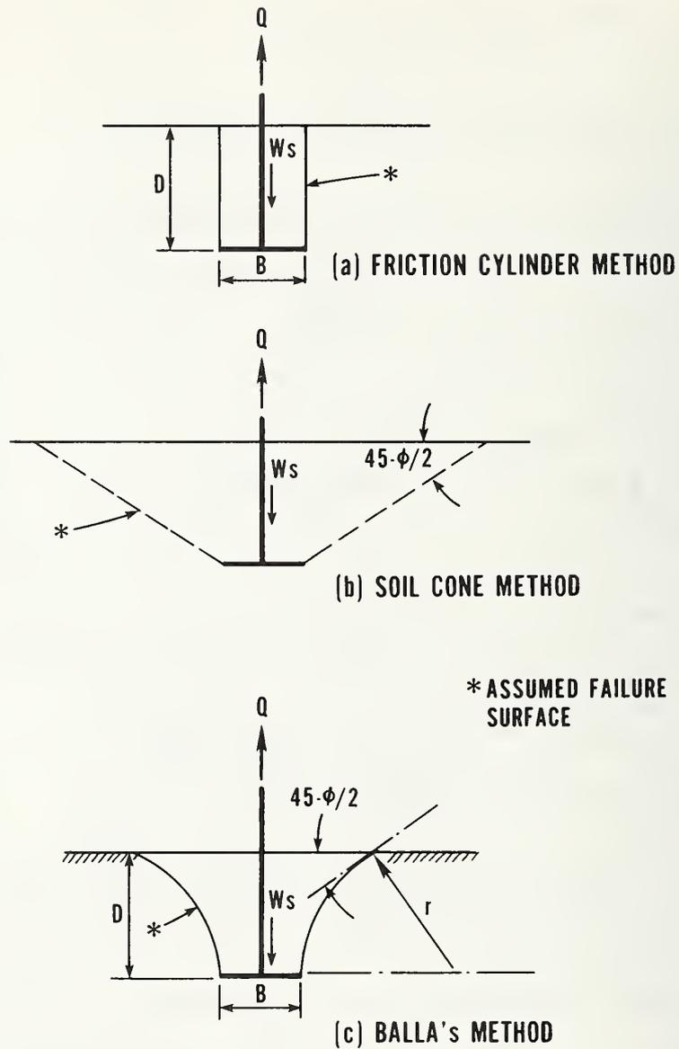
Figure 5.3 Methods of Calculating Pull-out Load Capacity [9]
