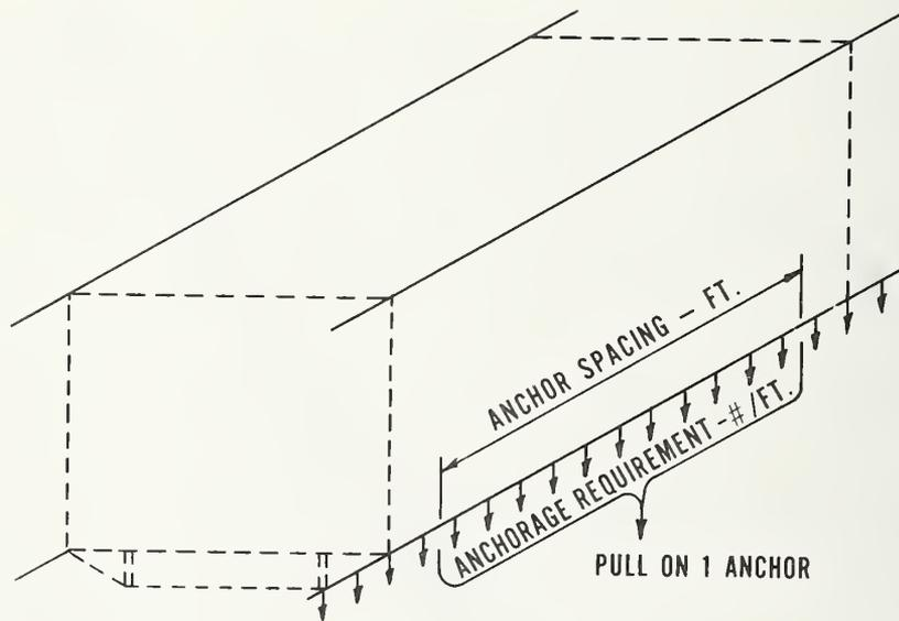
Figure 6.9 Relationship Between Anchor Spacing and Anchorage Requirement for the Pull on One Anchor [46]
