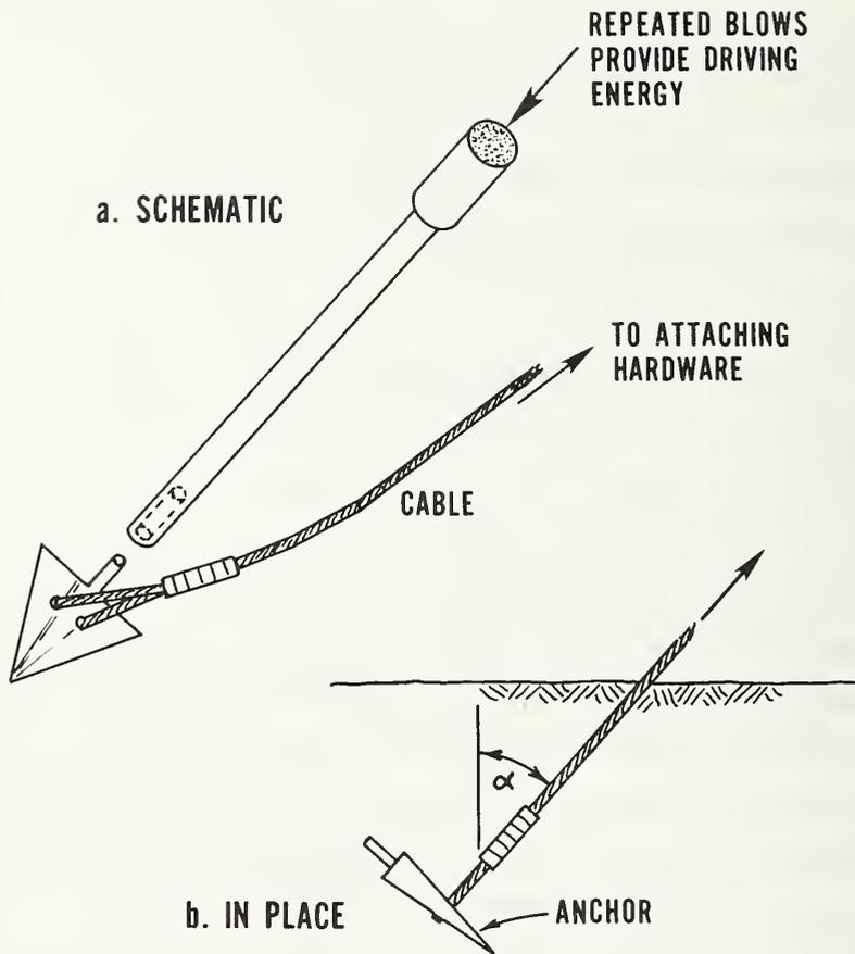
Figure 4.1 Triangular Ground Anchor
