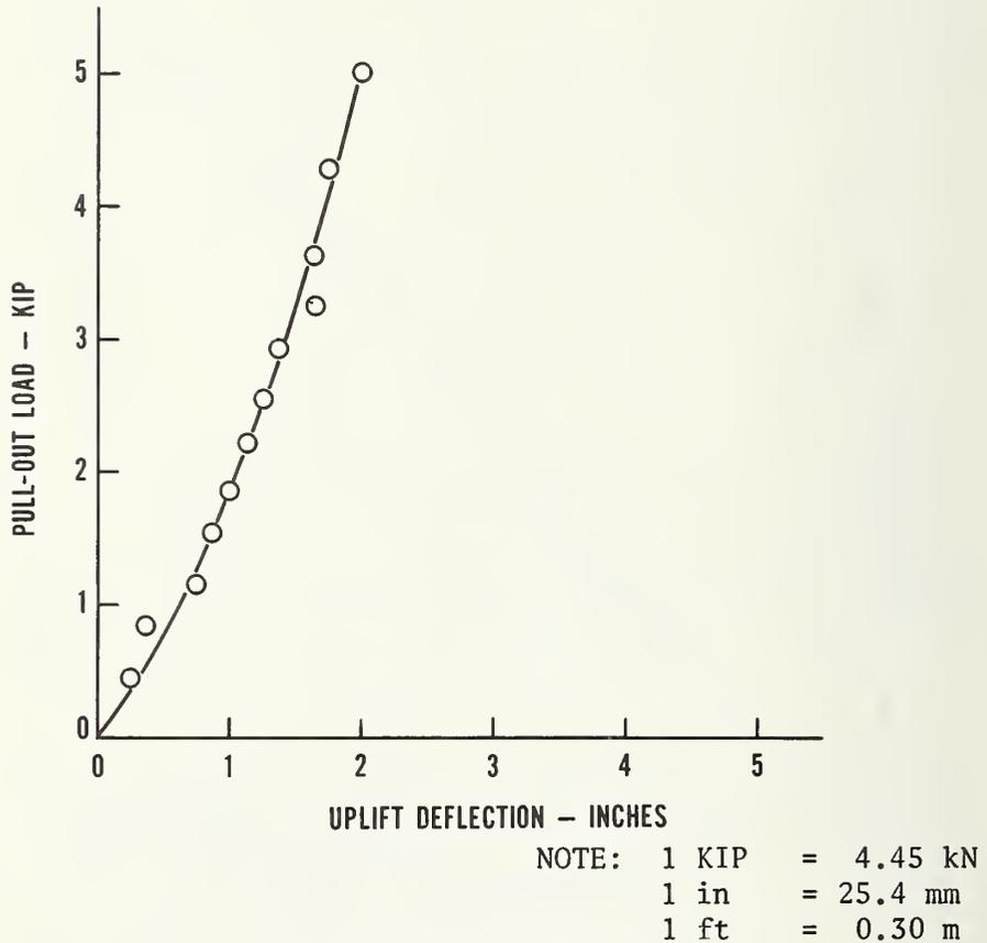
*Figure 7.8 Pull-out Load versus Uplift Deflection for a 6-inch Arrowhead Anchor*
