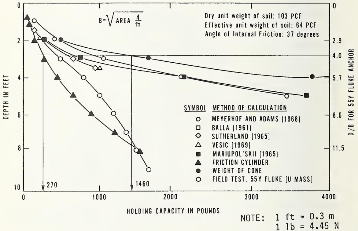
Figure 5.6 Comparison of the Holding Capacity of an Assumed 55 Square Inch Fluke in Anchor Saturated Sand Using Available Methods of Calculations [19]
