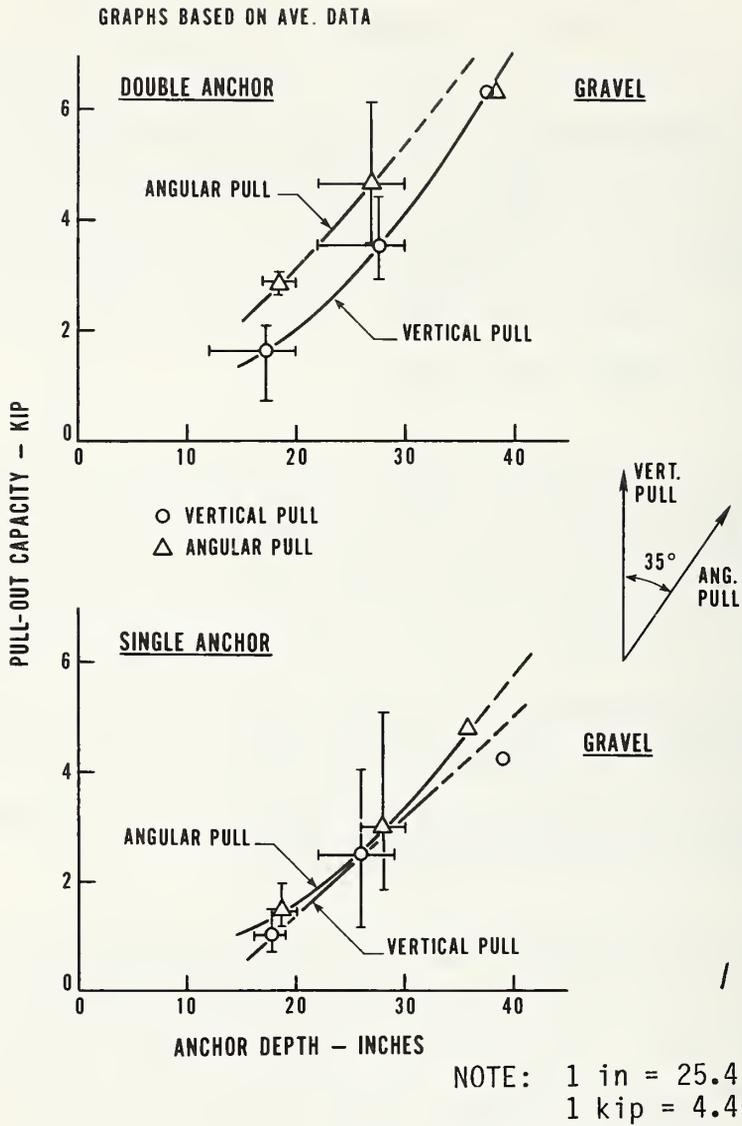
Figure 7.5 Pull-out Capacity versus Anchor Depth for 4-inch Arrowhead Shaped Anchors, Gravel Site [85]
