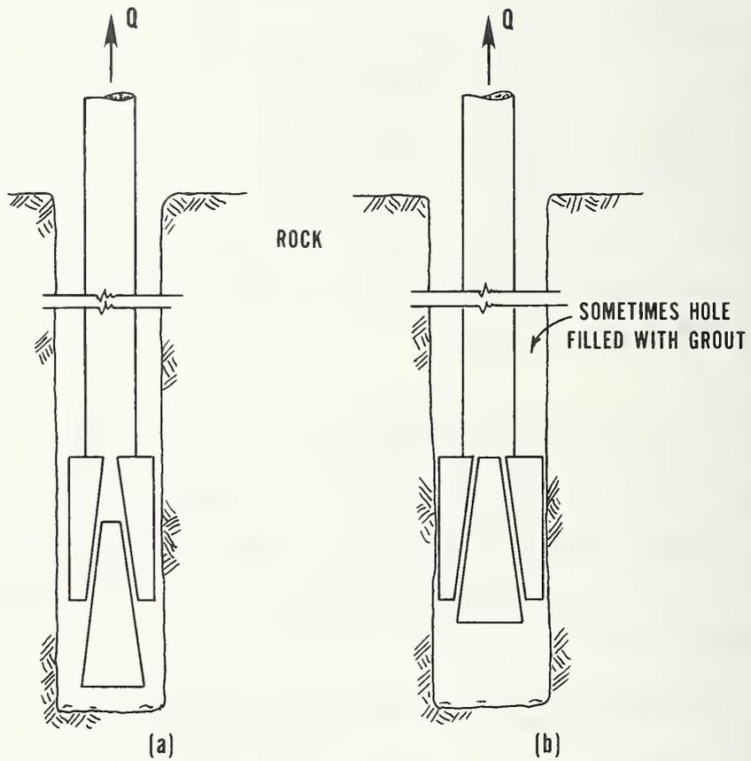
Figure 4.5 Principle of Expanding Rock Anchor: (A) Inserted in Drilled Hole; (B) In Expanded Position
