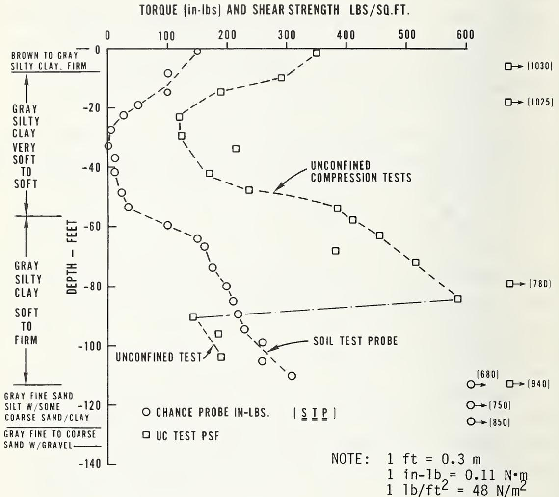
Figure 6.3 Soil Test Probe Torque and Shear Strength versus Depth for Site 5 [3]
