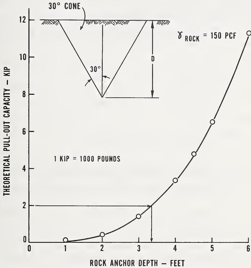
Figure 5.7 Theoretical Pull-out Capacity versus Rock Anchor Depth
