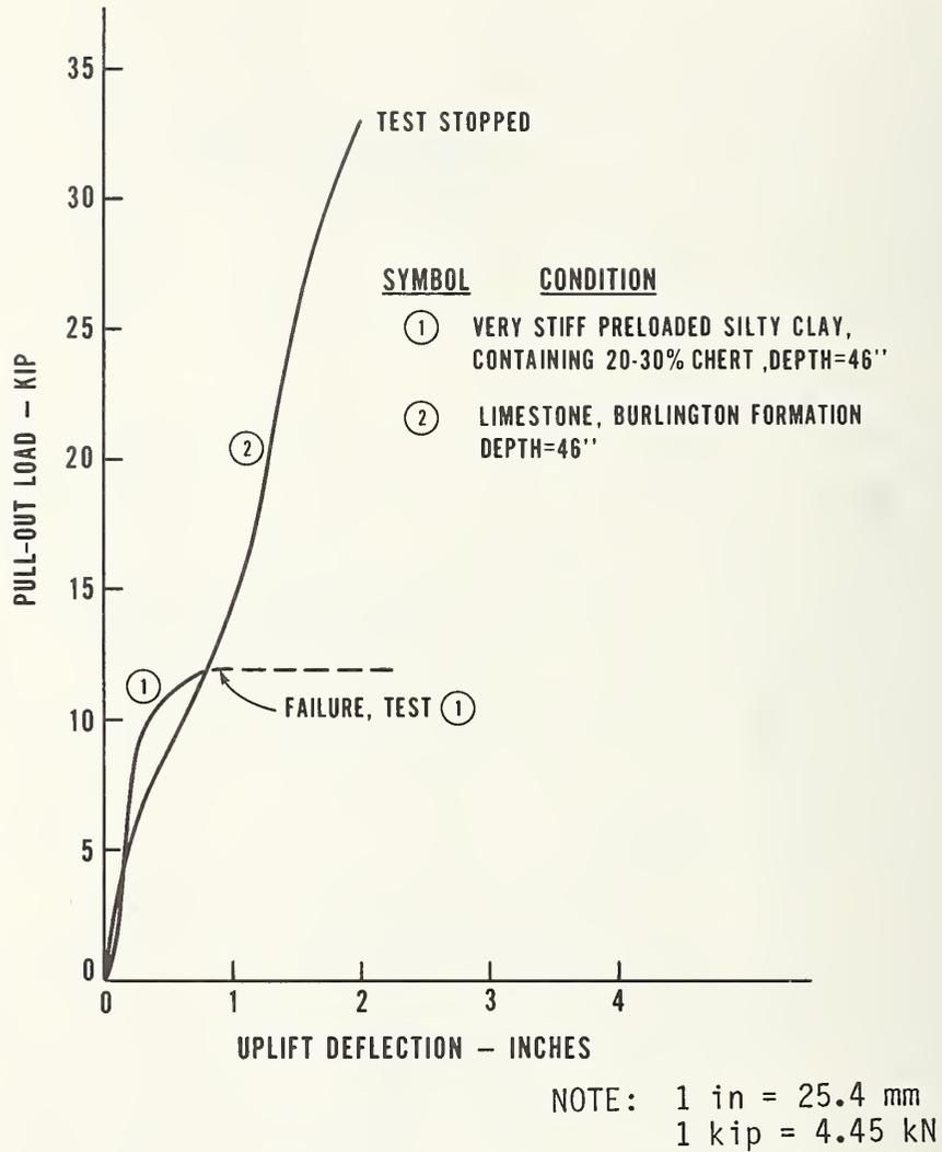
Figure 7.12 Pull-out Load versus Uplift Deflection for Expanding-Anchors in Rocky Material [23]
