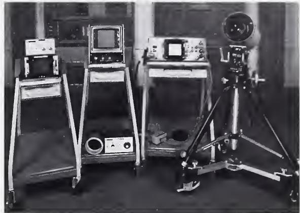
FIGURE B-1. Infrared television system.
