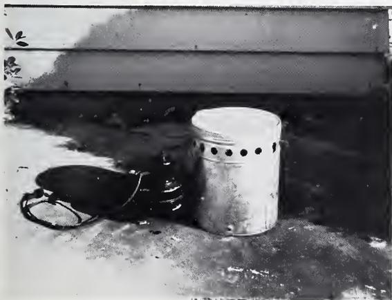
FIGURE C-1. *Drum-type smoke distributor.*
