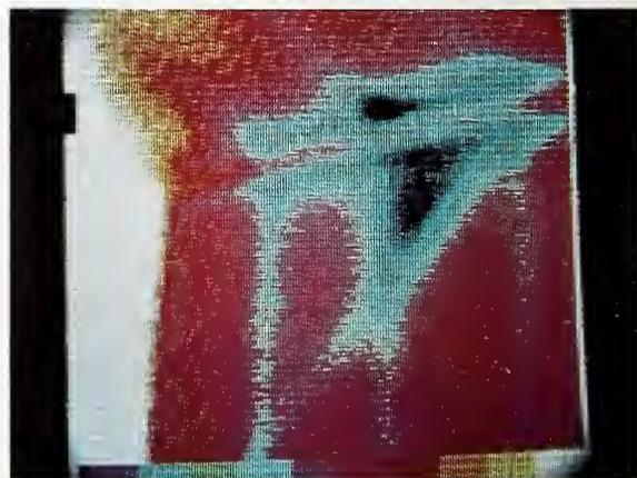
FIGURE B-8. Winter thermogram of inside surface of cellulose wall section in dining room.
