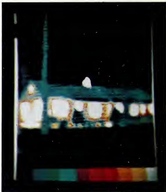
FIGURE B-2. Overall view of exterior surfaces of the test house. (b) Thermogram before retrofit.
