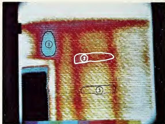
FIGURE B-7. Winter thermogram of inside surface of U-F wall section.
