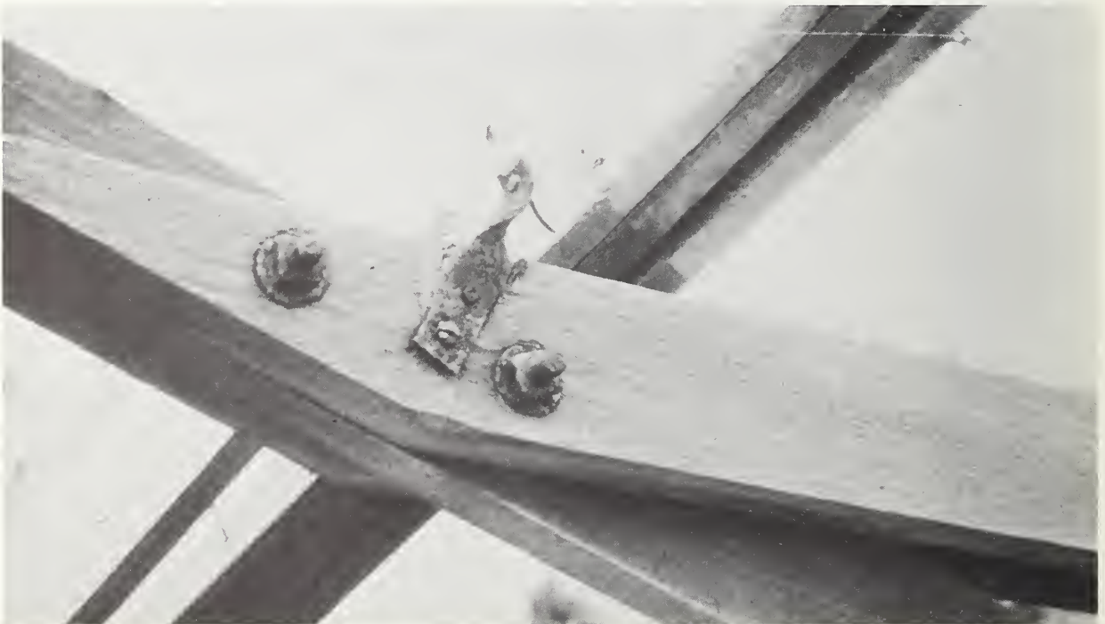
FIGURE 46 METAL STRAP ON ONLY ONE SIDE OF FRAMING FAILED TO RESIST BENDING LOAD.
