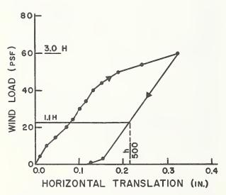
FIGURE 11. Performance of test structure under wind load.
