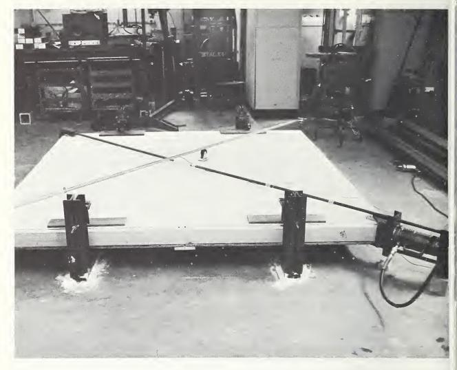
FIGURE 1. NBS Diagonal Racking Test Method.
