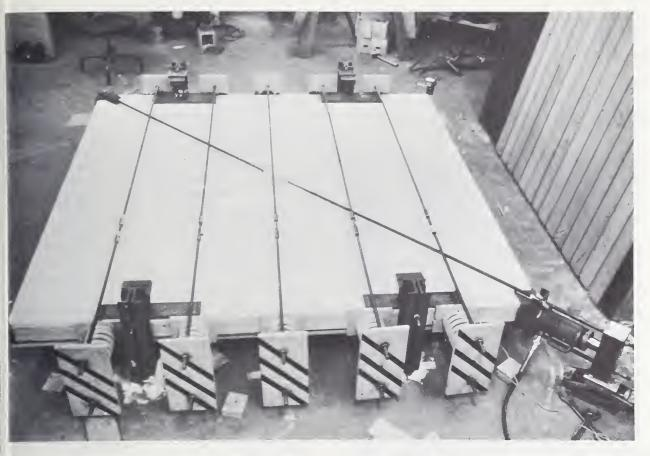
FIGURE 2. NBS Combined Compressive and Racking Test Method.
