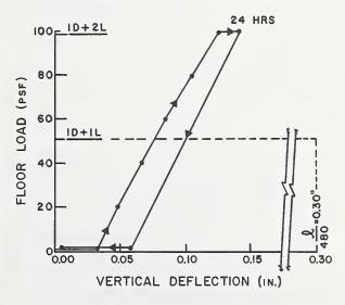
FIGURE 10. Performance of test structure under vertical load.
