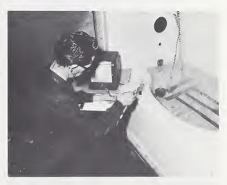
FIGURE 5. Apparatus used for studying the effects of prolonged exposure to hot water on a bathtub.
