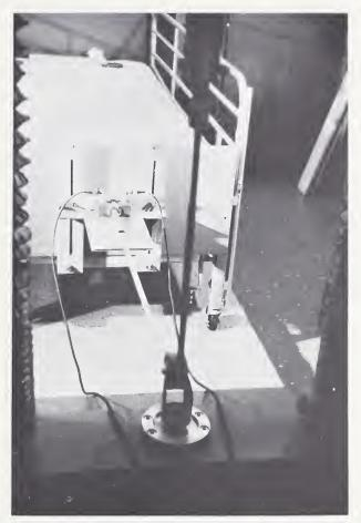
FIGURE 1. Equipment for testing resistance to wheeled equipment. Platform with carpet; hospital bed and connections to load cell, pulley, crosshead of load-strain testing machine.
