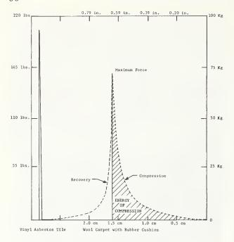
FIGURE 6. Typical compression-recovery curves.
