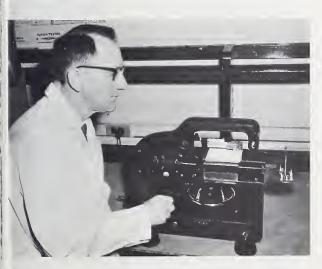
FIGURE 3. Modified PEI Gouge Test apparatus used for investigating the scratch resistance of sanitary plumbing fixtures.
