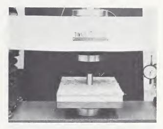
FIGURE 5. Apparatus and specimen for compression-recovery test. Shown from top to bottom: crosshead and load cell; cylindrical plate; cylindrical indentor; carpet sample; cement mortar panel; square steel plate; cylindrical plate.
