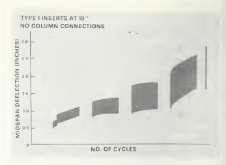
FIGURE 16. Component test on floor beam under cyclic loading.
