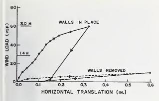
FIGURE 13. Ultimate strength of test structure under wind load.
