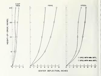
FIGURE 6. Concentrated load test (Dynamic), 150-lb. leather bag.
