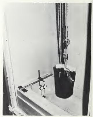
FIGURE 2. Apparatus used for application of dynamic loading of the interior of a bathtub.
