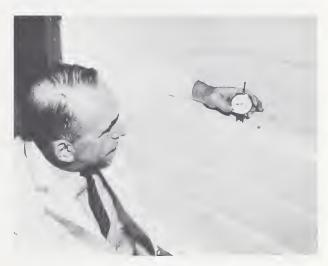
FIGURE 4. An investigator measures the amount of material that must be scoured away to remove the discoloration and char caused by a cigarette lying on the rim of a bathtub.
