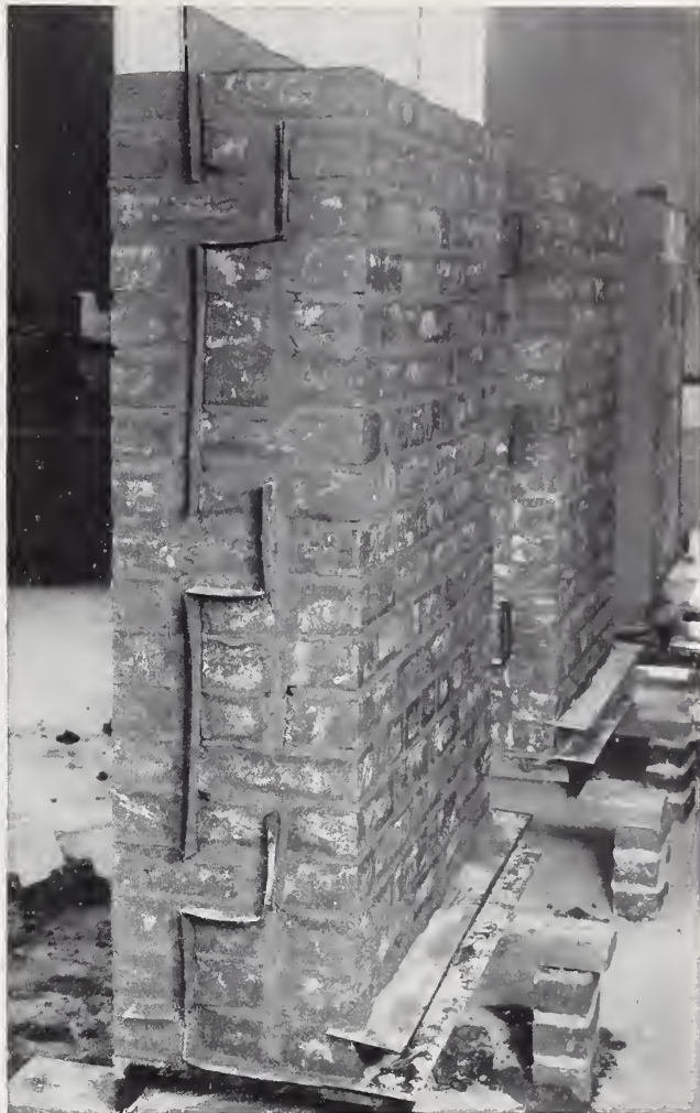
FIGURE 5.— Brick wall containing membrane waterproofing.
