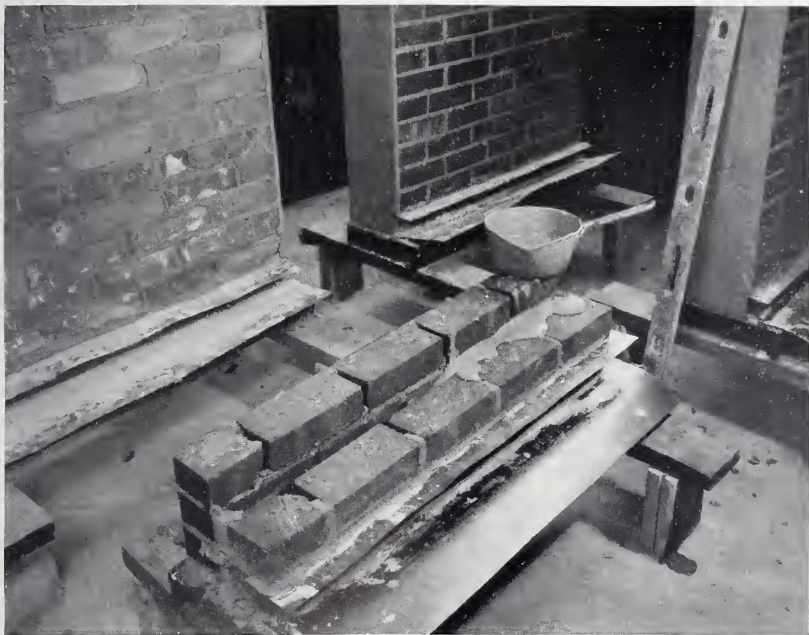
FIGURE 11.—Brick wall of workmanship H, grouted.
