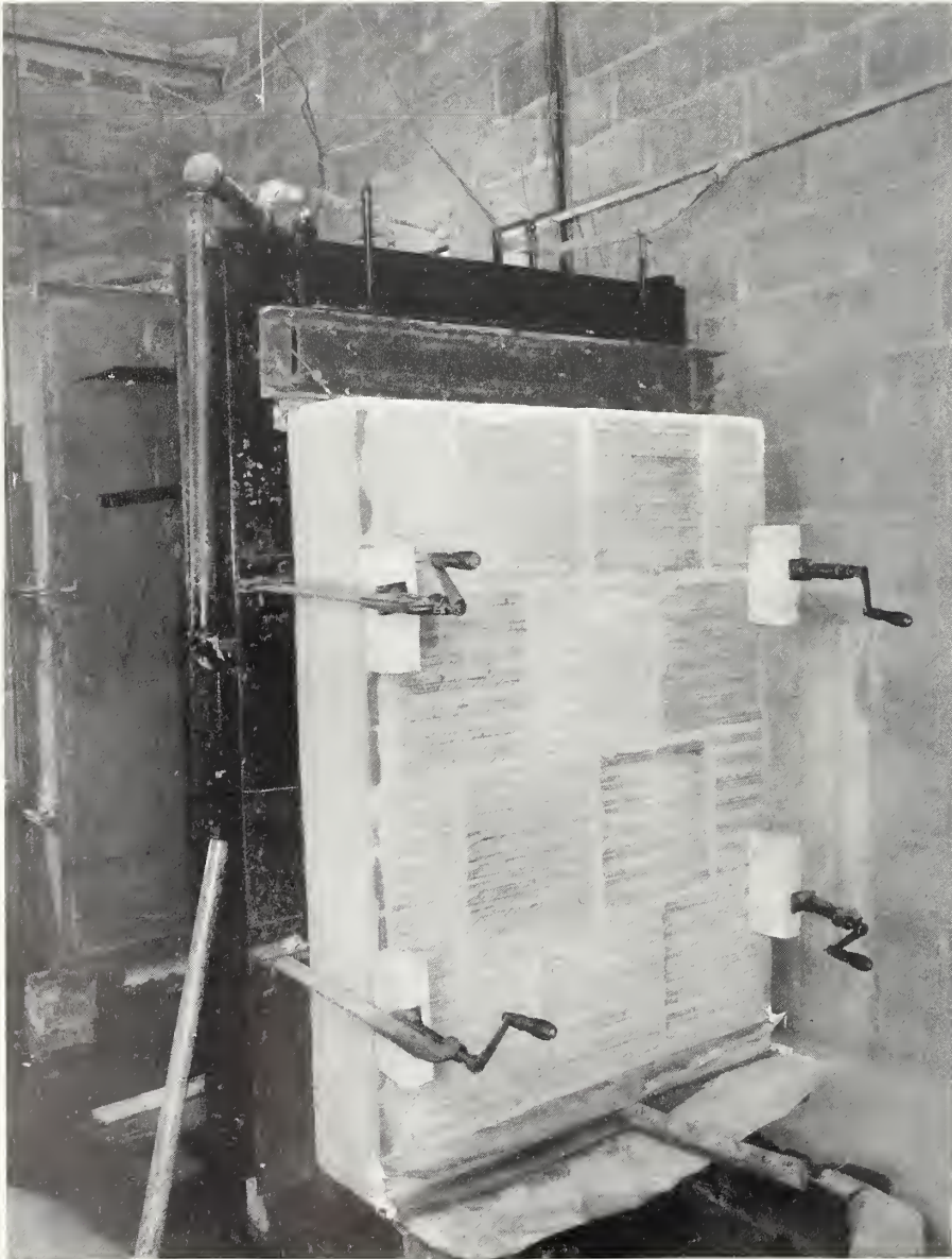
FIGURE 15.— Water-permeability test chamber.
