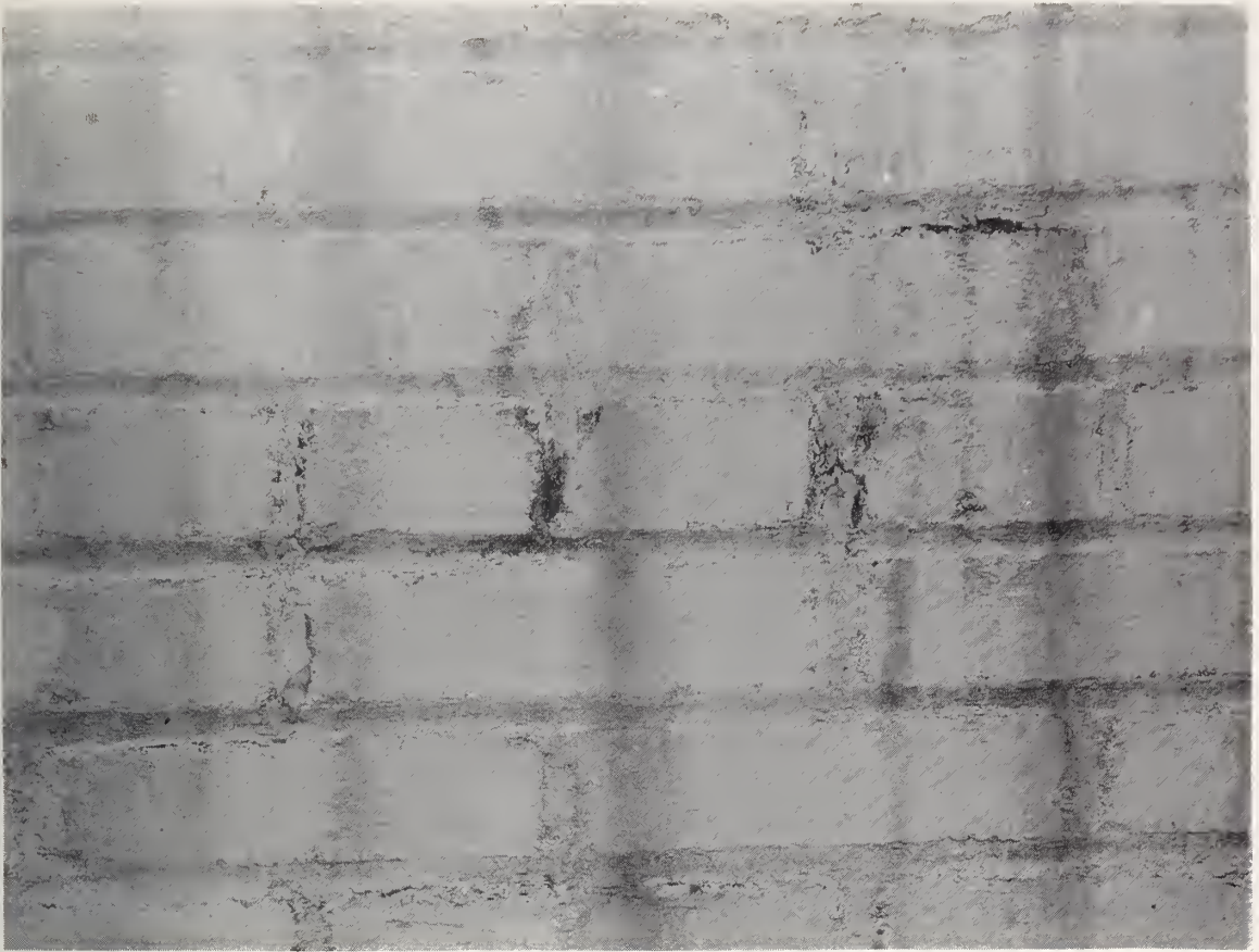
FIGURE 6.—Oil paint film on wall A10-bb8B2, after 3 years' outdoor exposure.
