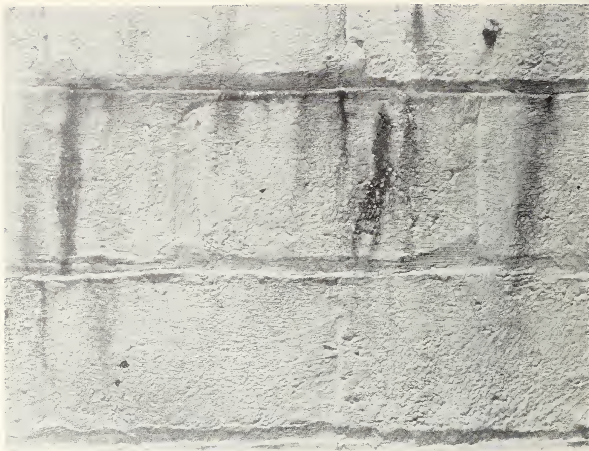
FIGURE 7.—Cement-water paint film on cinder block wall A11-n8B2 after 3 years' outdoor exposure.
