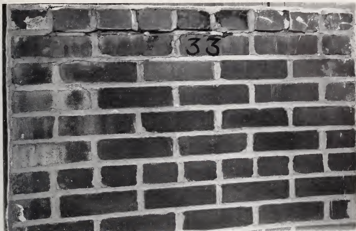
FIGURE 2.—Top portion of wall 33-cc12A3 after 3 years' outdoor exposure.
