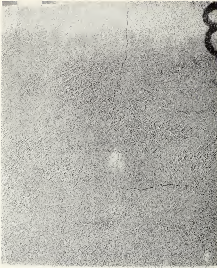
FIGURE 5.— Upper portion of wall 8-sj9A2 after 3 years' outdoor exposure.
