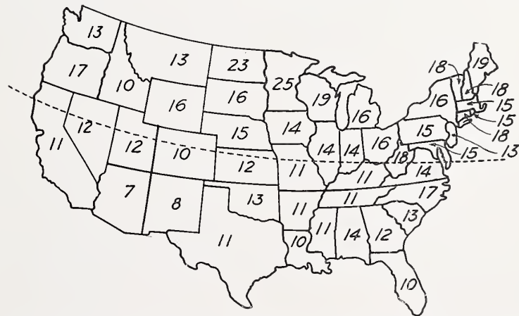
FIGURE 3.—Reported life of asphalt shingles, in years, averaged for each State.
