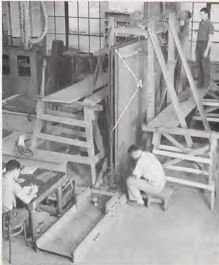
FIGURE 17.—Wall specimen CQ-R3 under racking load.
