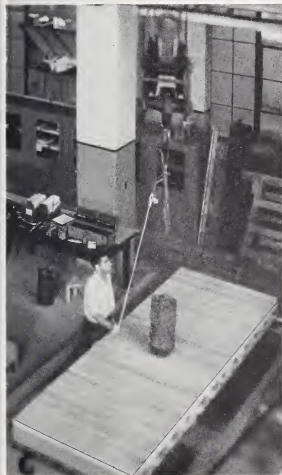
FIGURE 23.—Floor specimen CR-I1 during the impact test.
