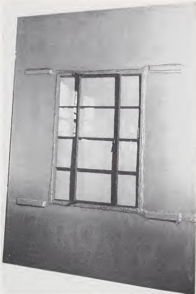
FIGURE 5.—*Light steel casement mounted in test panel.*
