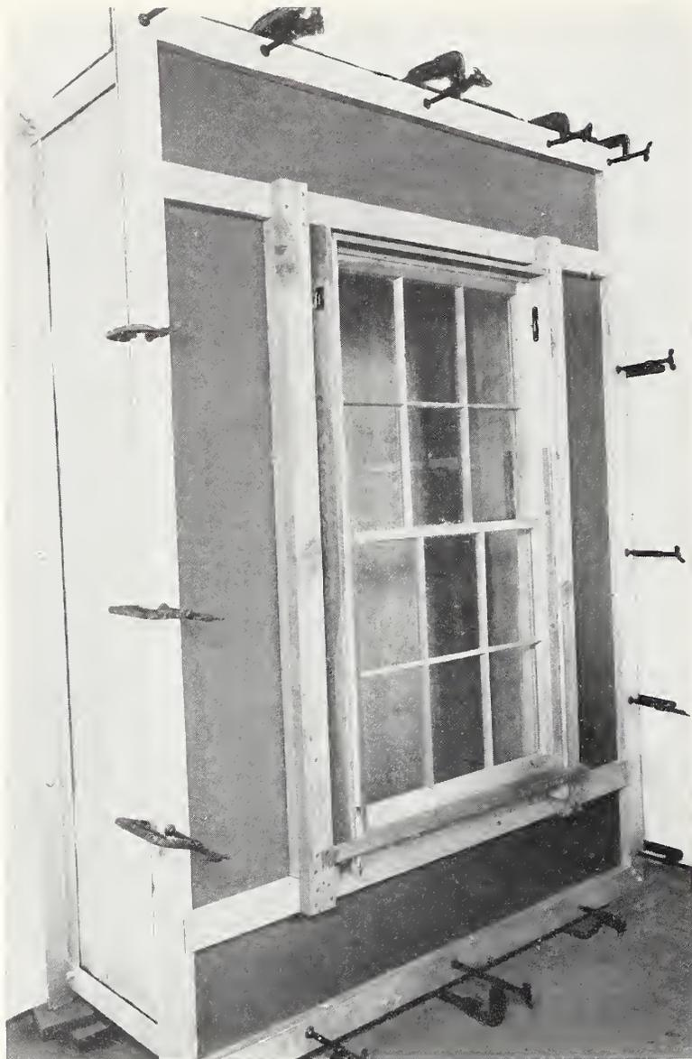
FIGURE 6.—*Double-hung wood window mounted in test panel.*
