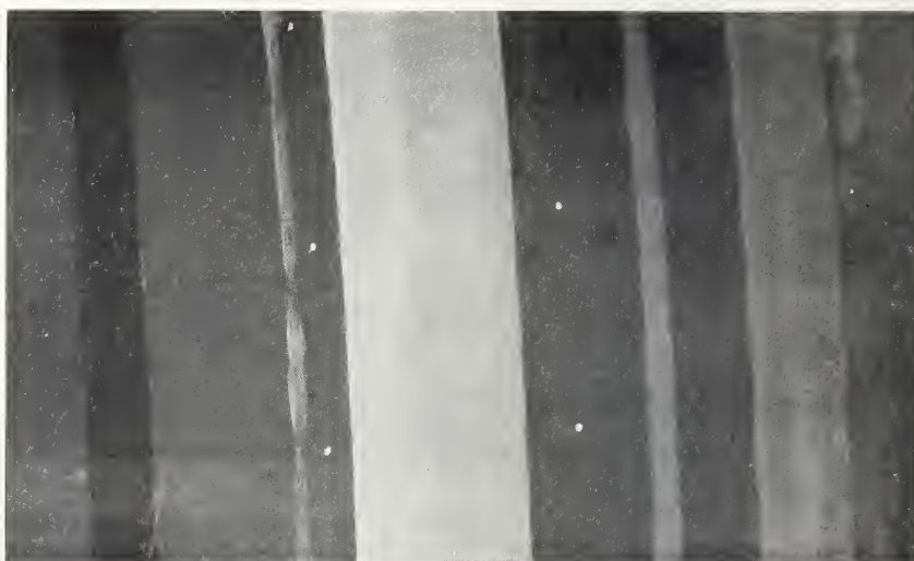
FIGURE 3.— \frac{1}{8} -in. battleship linoleum on wood subfloor (test panel 2L).
