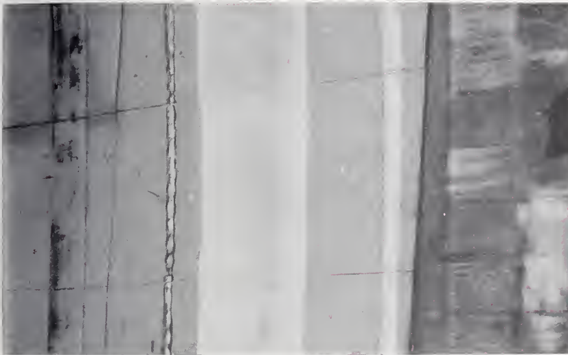
FIGURE 23.— \frac{3}{16} -in. asphalt tile, cumar-resin type, on concrete subfloor (test panel 15L).
