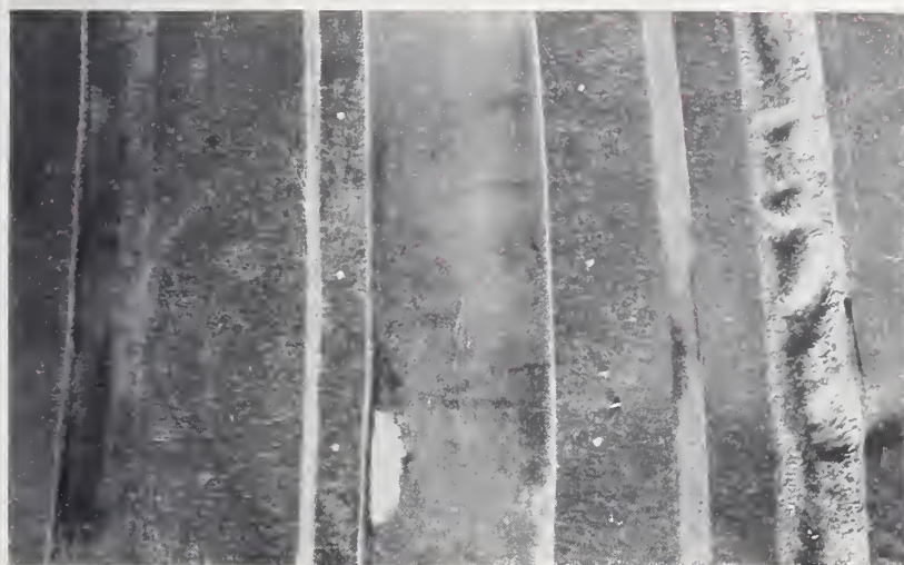
FIGURE 11.— Nitrocellulose composition felt base on wood subfloor (test panel 8L).
