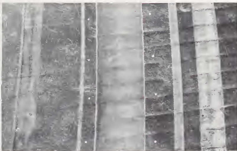
FIGURE 12.— Pitch and resin mastic felt base on concrete subfloor (test panel 7R).
