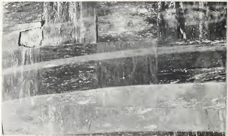
FIGURE 9.— \frac{1}{8} -in. rubber tile on concrete subfloor (test panel 5L).
