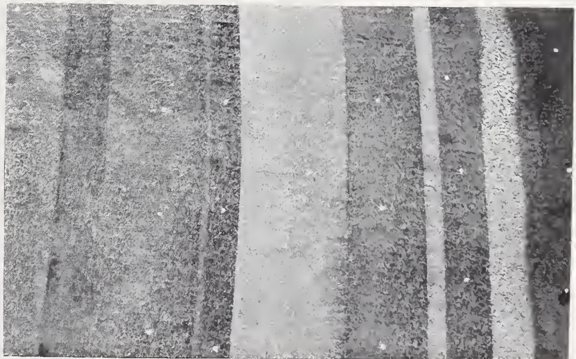
FIGURE 18.— \frac{1}{4} -in. alumina cement-later monolithic composition on cement-mortar subfloor (test panel 11L).
