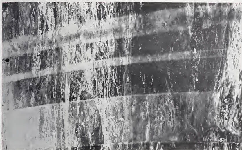
FIGURE 5.— \frac{1}{8} -in. sheet rubber on wood subfloor (test panel 4R).
