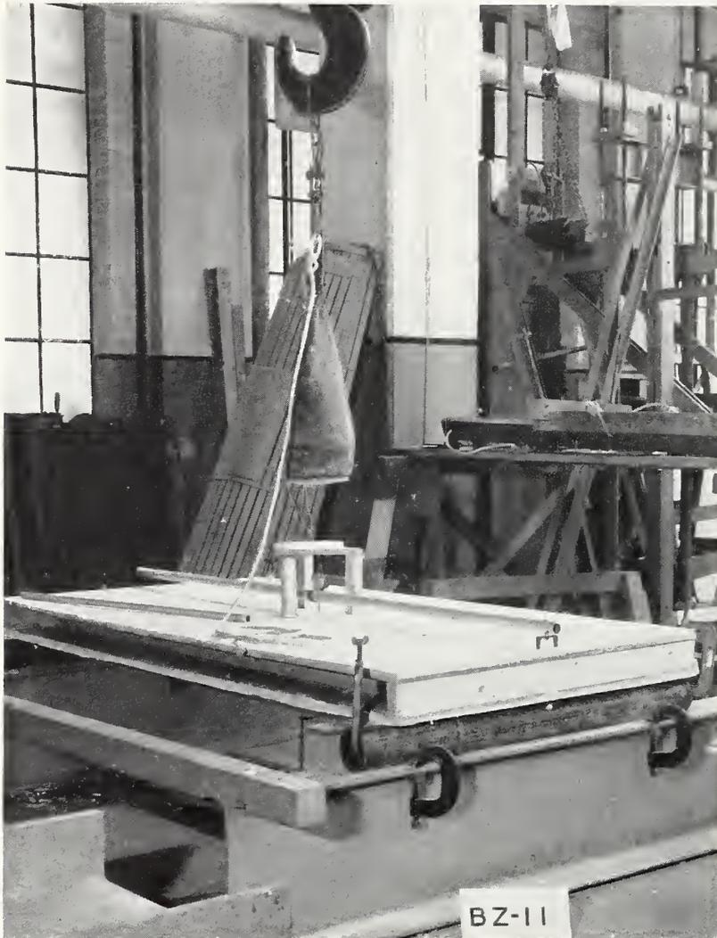
FIGURE 32.—Partition specimen *BZ-11* during the impact test.
