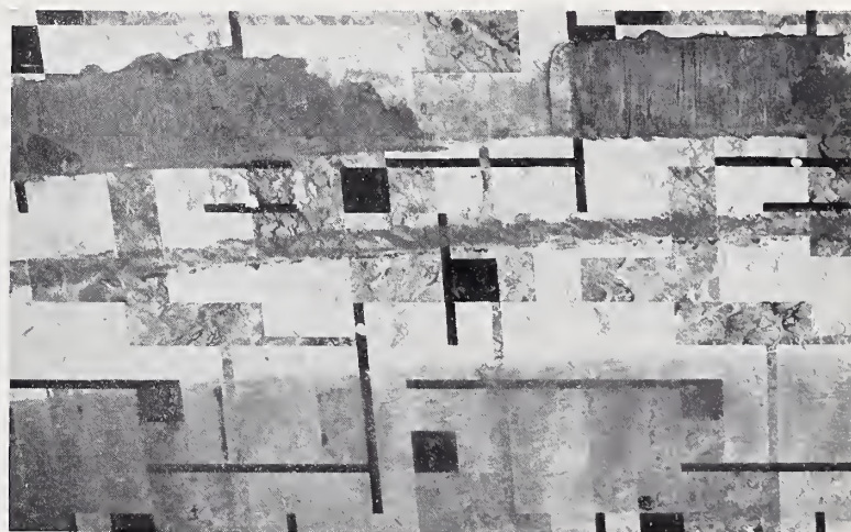
FIGURE 11.— Inlaid felt base on wood subfloor (test panel 10-L).
