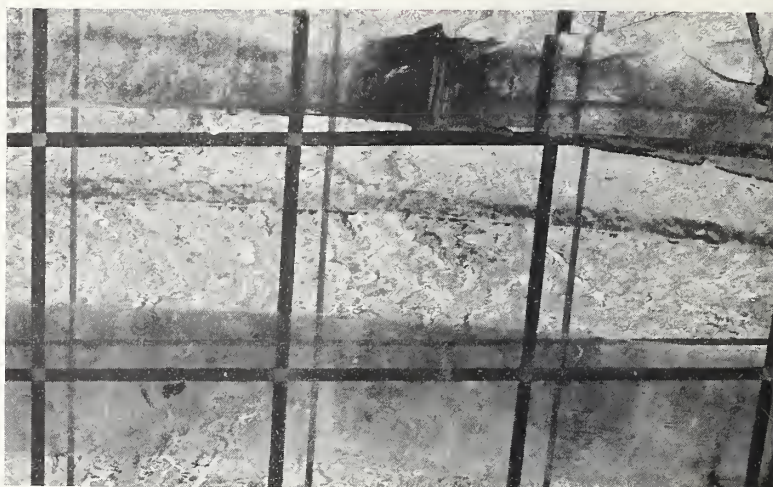
FIGURE 13.— Inlaid felt base on wood subfloor (test panel 12-R).
