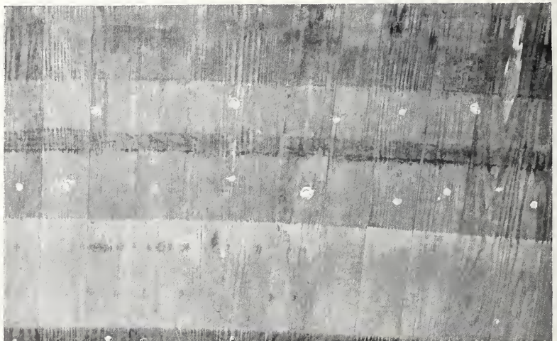
FIGURE 20.— \frac{25}{32} -in. strip yellow pine on wood sleepers (test panel 20-R).
