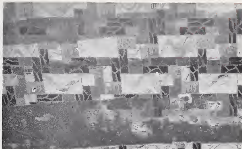
FIGURE 9.— Printed linoleum on wood subfloor (test panel 8-L).
