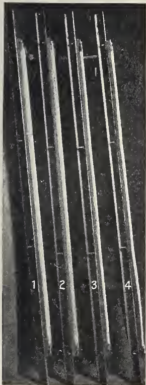
FIGURE 14.— Four panels showing that buckling across the studding was insignificant when plaster which set within 2 hours was used but with slower setting plaster the buckling was considerable.
