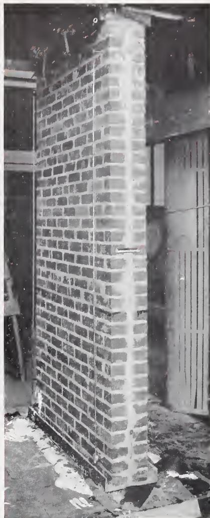
FIGURE 2.—*Wall specimen AT-C3 under compressive load*
