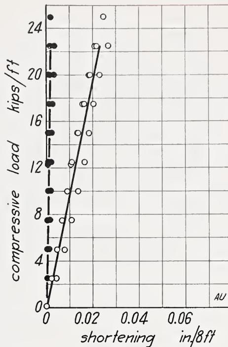
FIGURE 12.—Compressive load on wall *AU*.
