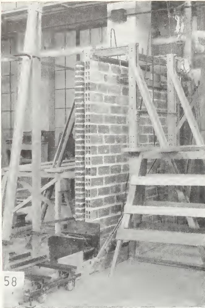
FIGURE 22.—Wall specimen AU-R1 under racking load.
