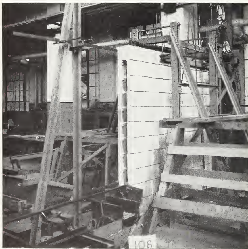
FIGURE 13.—Impact load on wall BE, load applied to inside face.
