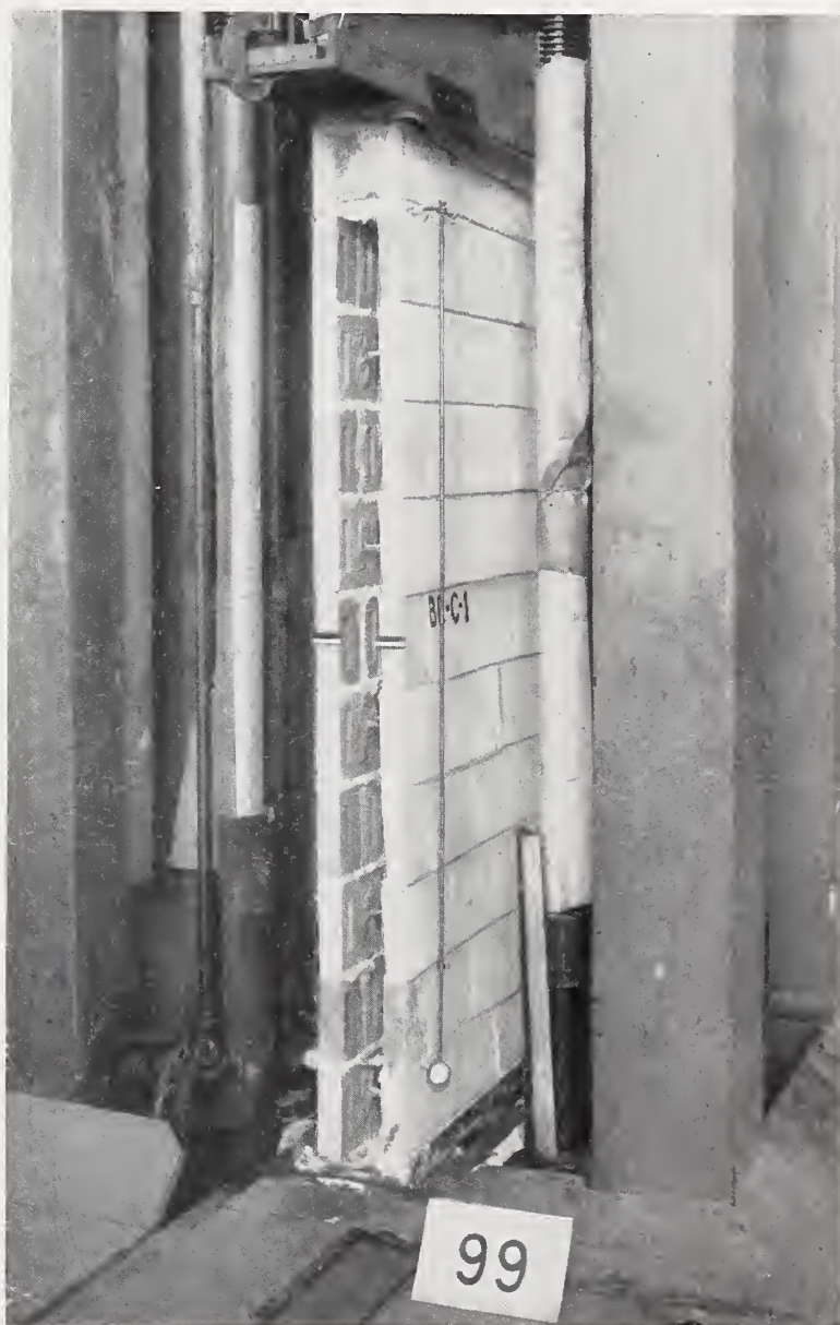
FIGURE 3.—Wall specimen BE-C1 under compressive load.
