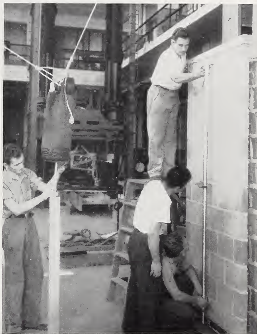
FIGURE 12.—Wall specimen BE-I1 during the impact test.
