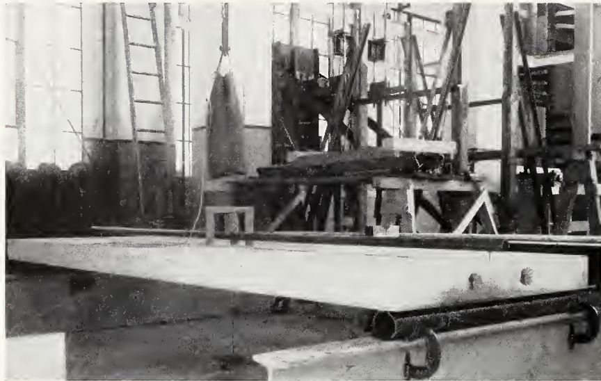
FIGURE 18.—Floor specimen AS-13 during the impact test.
