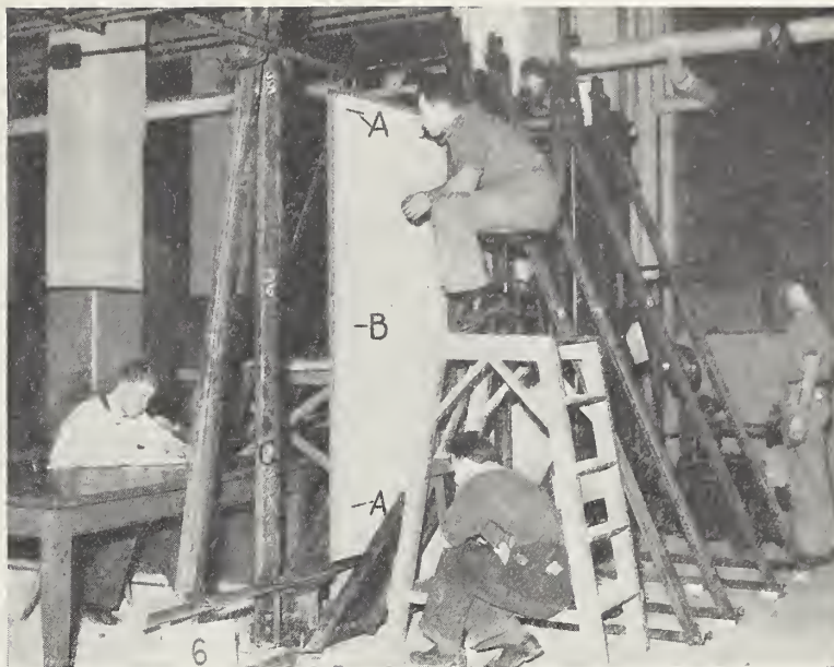
FIGURE 17.—Apparatus for racking load on specimen.
