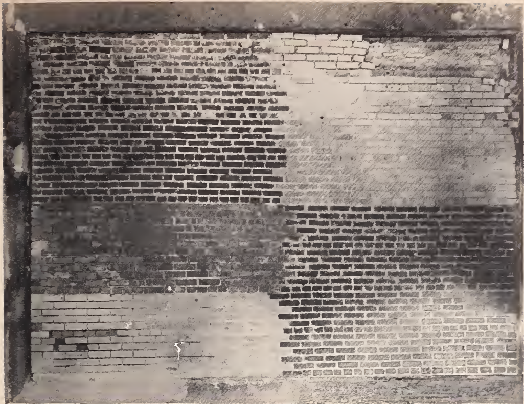
FIGURE 42. Exposed side of 8-in. solid unrestrained wall 74 after fire and hose-stream test.
