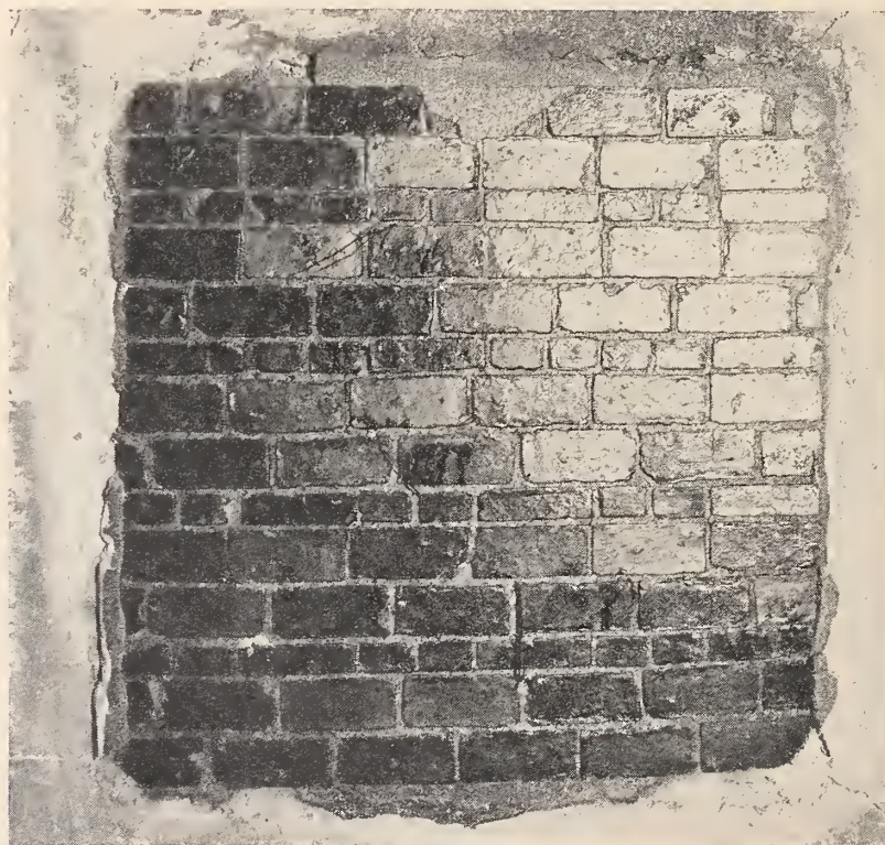
FIGURE 39. Fire-exposed side of 12-in. flat-bond rolok wall 67 after 10-hr 50-min fire exposure.
