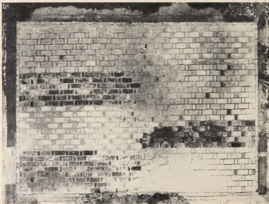
FIGURE 45. Exposed side of 8-in. all-rollok restrained wall 76 after fire and hose-stream test.
