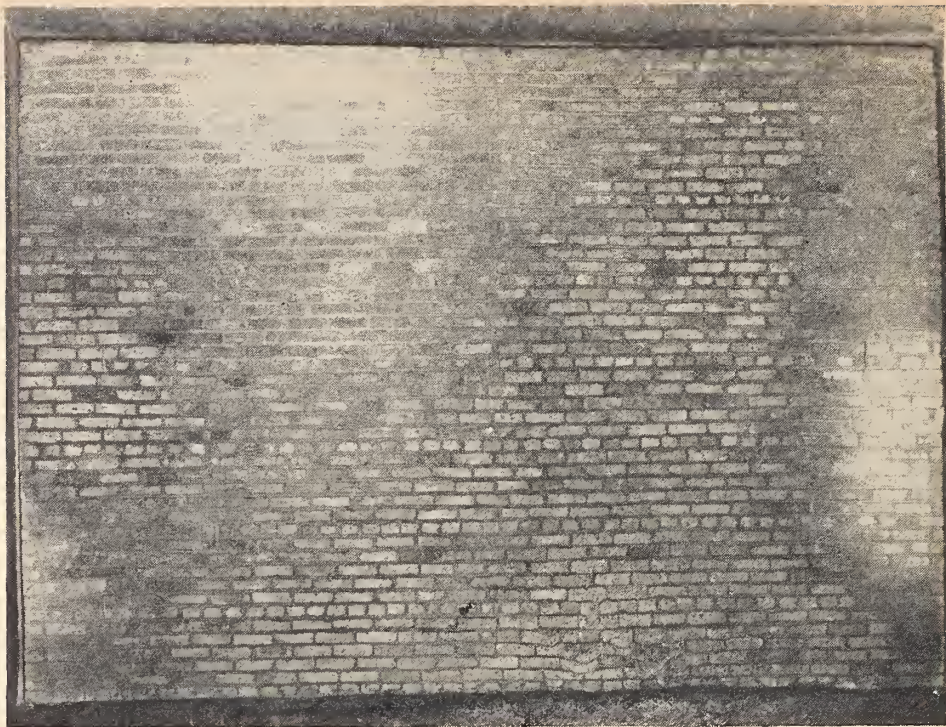
FIGURE 22. Fire-exposed side of 8-in. concrete-brick wall 25 after 6-hr fire test.
