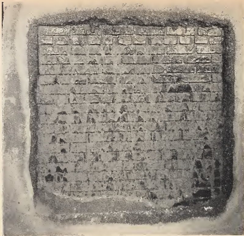
FIGURE 18. Fire-exposed side of plastered clay-brick wall 37 after 11-hr fire test.
