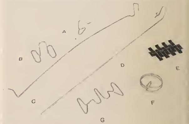
FIGURE 3. Various clips used in applying ceiling laths for the test specimens.
