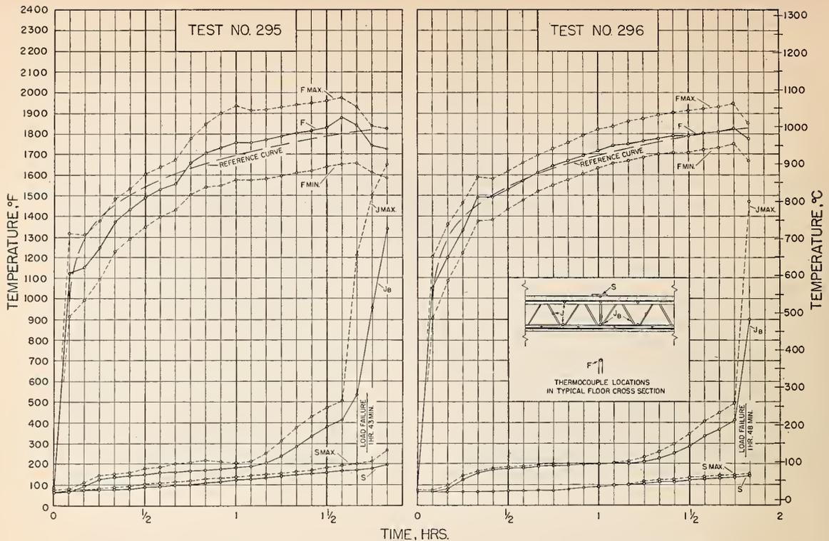
FIGURE 9. Time-temperature curves from tests 295 and 296, unreinforced ceilings.
