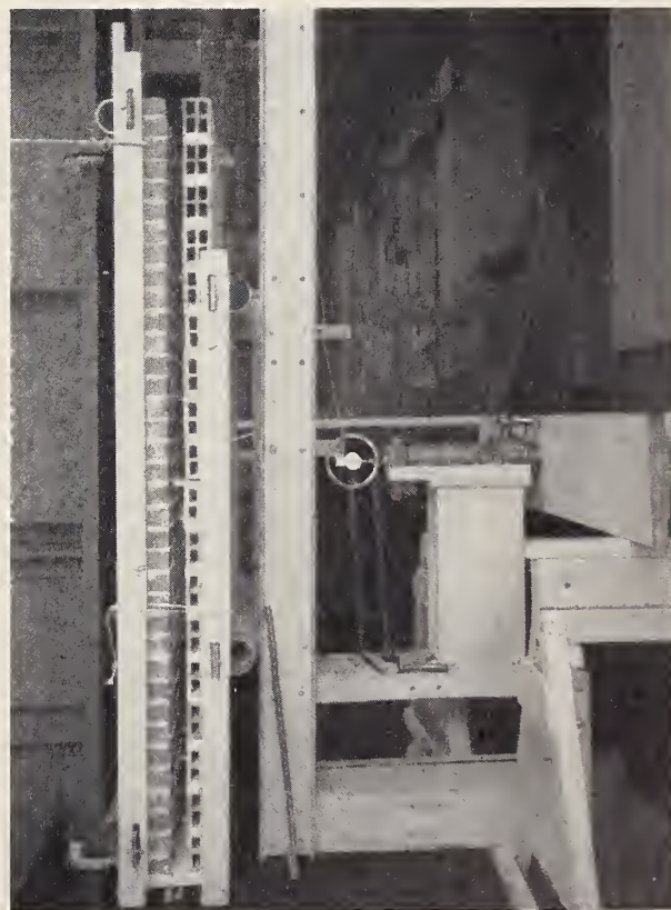
FIGURE 8. Brick-tile cavity wall under transverse load. Loading rollers at quarter span are shown to the right of the wall.
