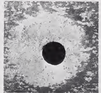
CORROSION FROM LEAD WASHER MATERIAL 9A
