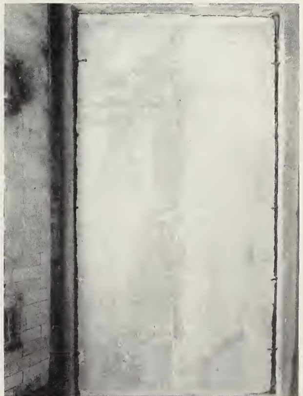
FIGURE 13. Fire-exposed face of a crushed quartz concrete wall slab after 1½-hr test.
