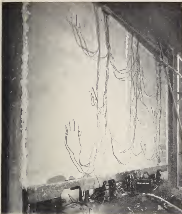
FIGURE 3. Unexposed side of load-bearing wall, 10, after fire exposure of 3 hr 55 min on the opposite side.
